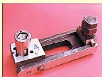
Various designs of diamond anvil cells (DAC) developed (1. Modified Mao Bell DAC, 2. Miniature clamp type DAC, 3. Bassett DAC, 4. Modified Merrill Bassett DAC)
