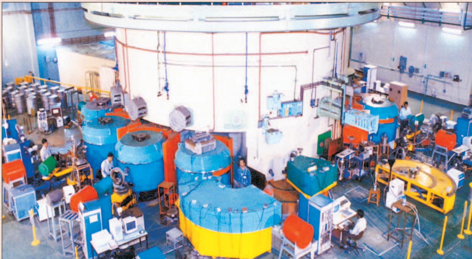
Panoramic view of the neutron spectrometers at Dhruva reactor, BARC. The facilities existing are powder and single crystal diffractometers for crystal structure determination, Hi-Q diffractometer for structural studies in amorphous and liquid systems, polarization neutron spectrometer for magnetic scattering studies, for small angle neutron scattering (SANS), quasi-elastic scattering studies (QENS), inelastic neutron scattering studies
