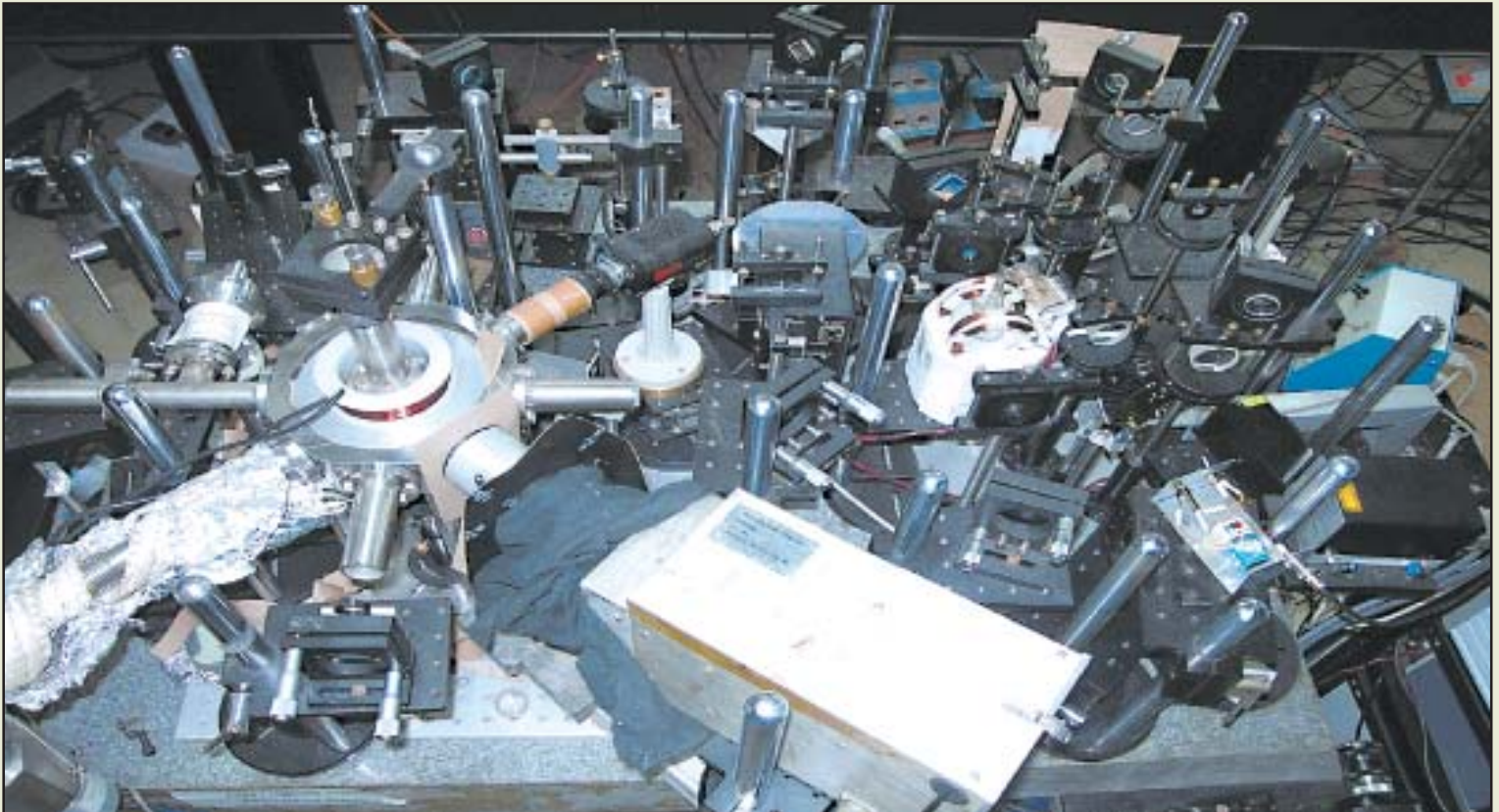
A view of the laser-cooling facility in BARC. The picture shows the magneto-optical trap (MOT) consisting of an octagonal chamber, diode lasers, optics and opto-mechanical components, and diagnostic equipments
