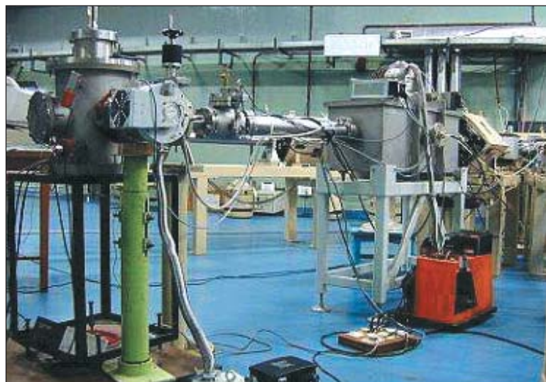
AMS beamline. The 15° cylindrical ESA is located before the chamber
