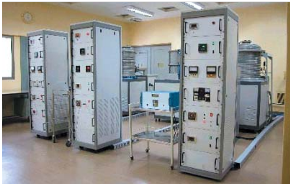
Systems for the single crystal growth of fluoride materials under high vacuum conditions
