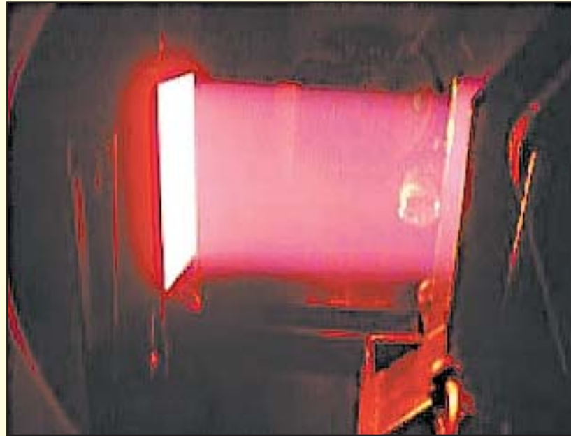
5 MW ion source in operation (ion + neutral) during test run
