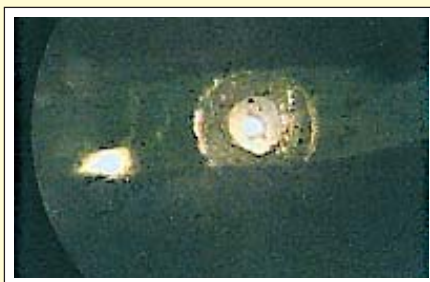
Direct conversion of graphite to a "Diamond-Like" phase using the LHDAC facility at 14 GPa, with CO 2 laser power of ~15 watts. (a). black graphite sample under high pressure inside the DAC, (b). the shining laser heated zone of the pressurized graphite sample, and (c). formation of the translucent diamond-like phase after heating
