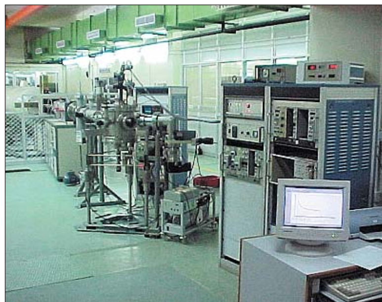
1.7MV Tandatron accelerator along with the ion irradiation and ion beam analysis experimental setup installed at 10 degree beam line for materials research
