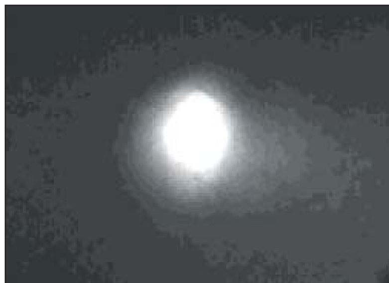
Fluorescence image of the cold cloud of atoms ( \sim 100 million) formed at the centre of the MOT. The cloud has diameter of \sim 1 mm and the temperature of \sim 100 microKelvin
