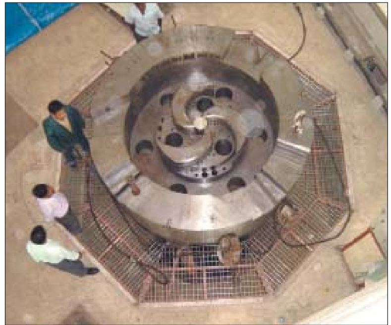
Top view of the main magnet frame of superconducting cyclotron under assembly
