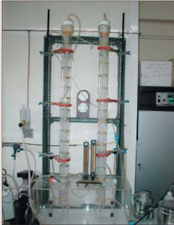
An Inebriometer used for study of general anaesthesia in flies
