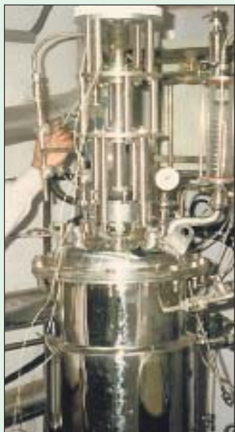
Bioreactor (100 L) equipped with helix impeller for growth of Catharanthus roseus cultures
