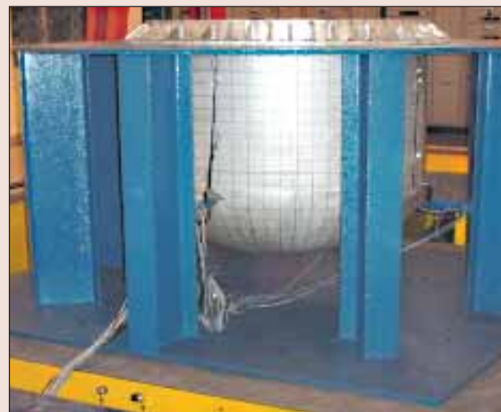
Seismic tests on reactor assembly model
