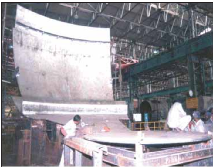
Main vessel under fabrication for FBR
