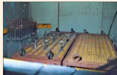
Model of lower axial plenum region of FBR core subassembly used for shielding experiments in APSARA to estimate the neutron damage to the grid plate.
