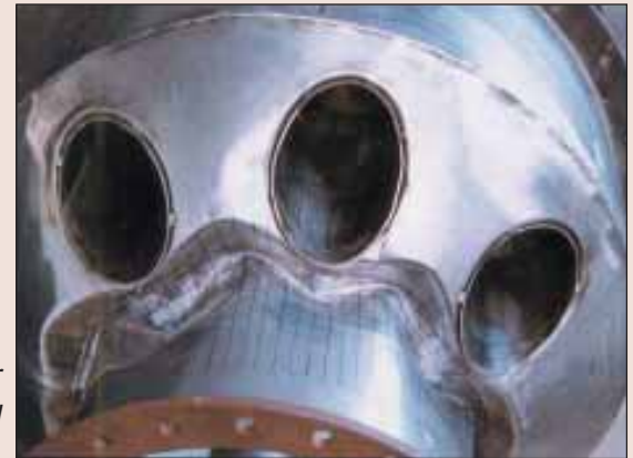
Buckling of inner vessel model
