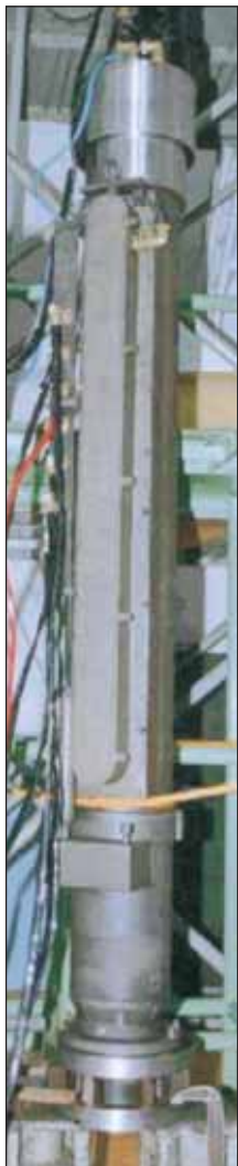
Diverse Safety Rod Drive Mechanism (DSRDM)
