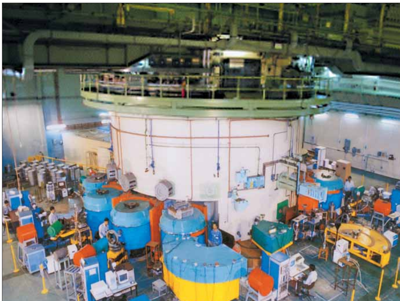
Facility to extract a beam of neutrons from the DHRUVA for its utilization in experiments
