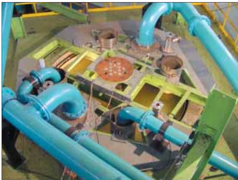
SAMRAT - 1/4 scale model of PFBR reactor assembly
