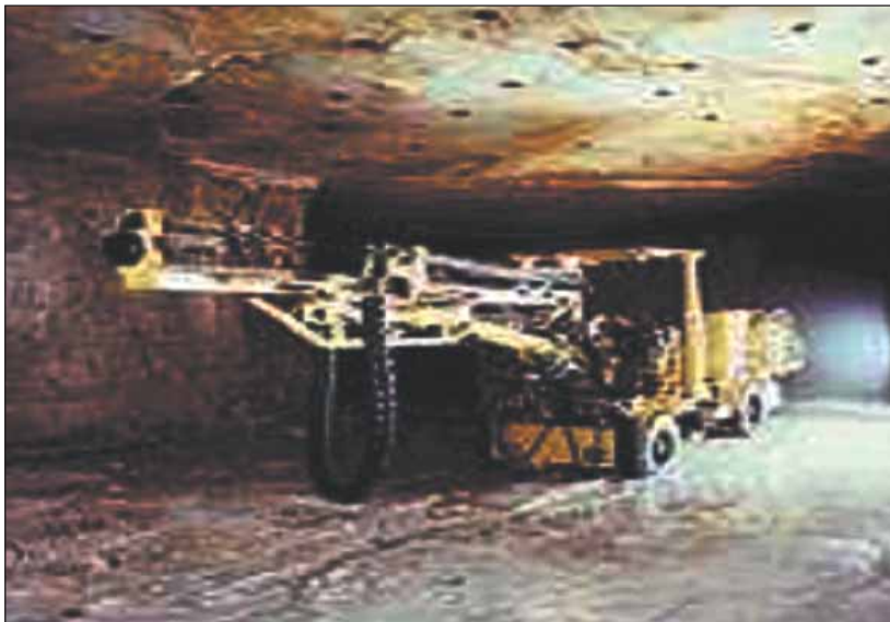
Mechanised ore drilling at Jaduguda
