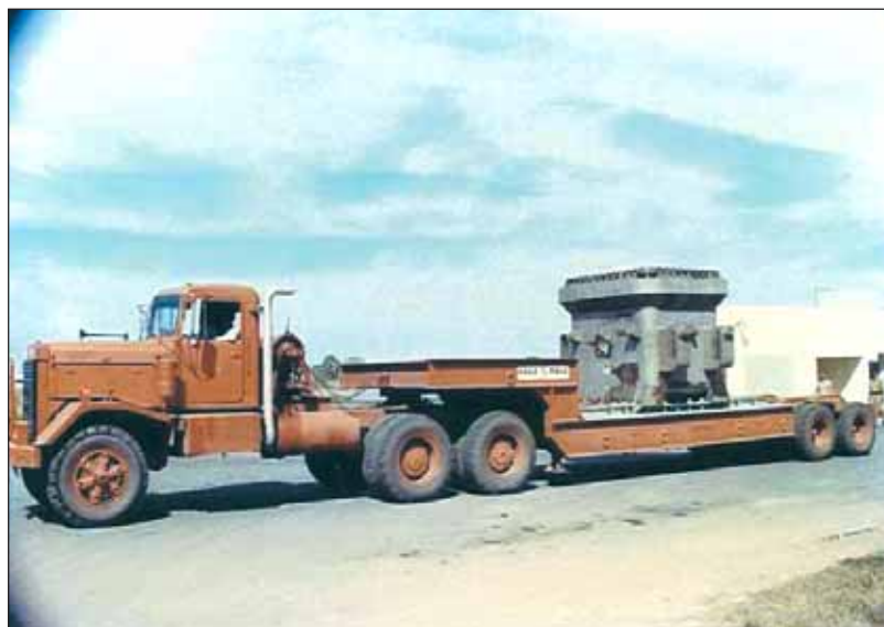
Shipping of the cask containing spent fuel on trailer
