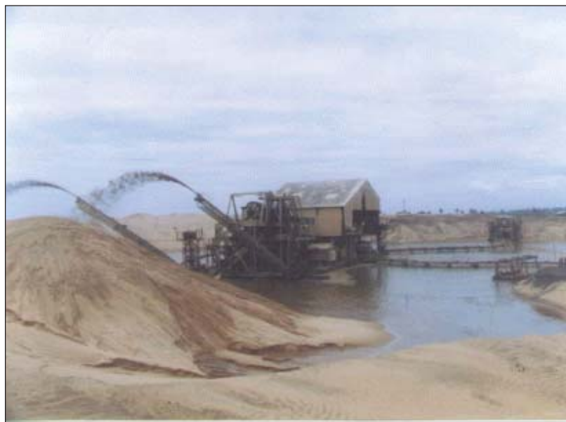
A Dredge and Wet Concentrator in operation at Orissa Sands Complex (OSCOM)
