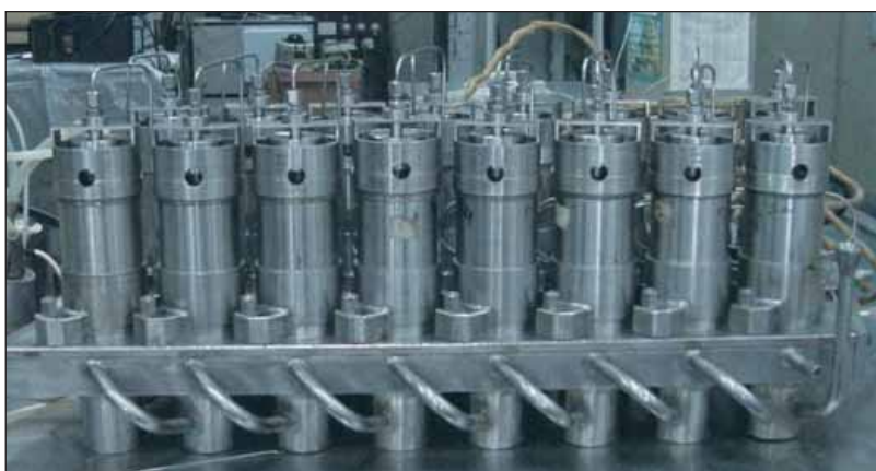
16-Stage centrifugal extractor bank
