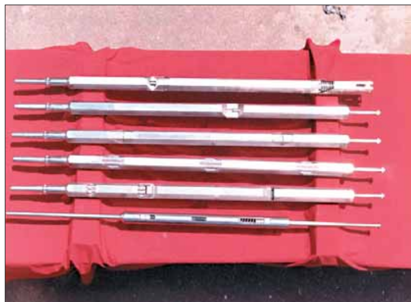
Demonstration of indigenous technological capability - FBTR Fuel sub-assemblies with cut sections
