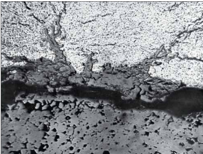
Typical fuel-clad chemical interaction site and a SEM photomicrograph of clad inner surface of TAPS fuel pin. Top picture shows the fission product deposit on the inside surface of cladding tube. Bottom picture shows the fuel cladding interaction
