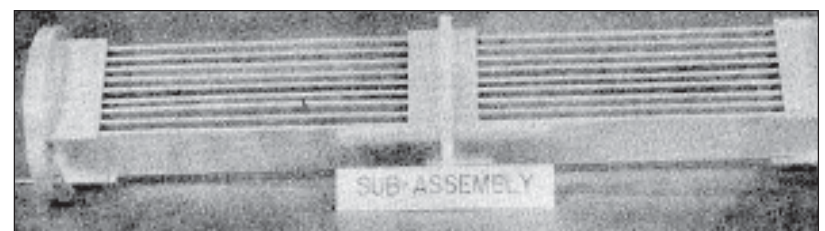
9-plate fuel subassembly of Al clad Al-Pu alloy for ZERLINA
