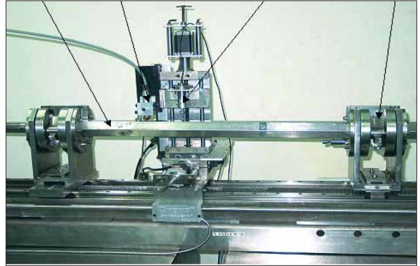
Mechanical system used for the laser-dismantling of FBTR FSA
