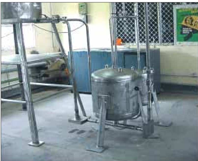
Fluidic diode pump top: schematic, bottom : under evaluation in plant
