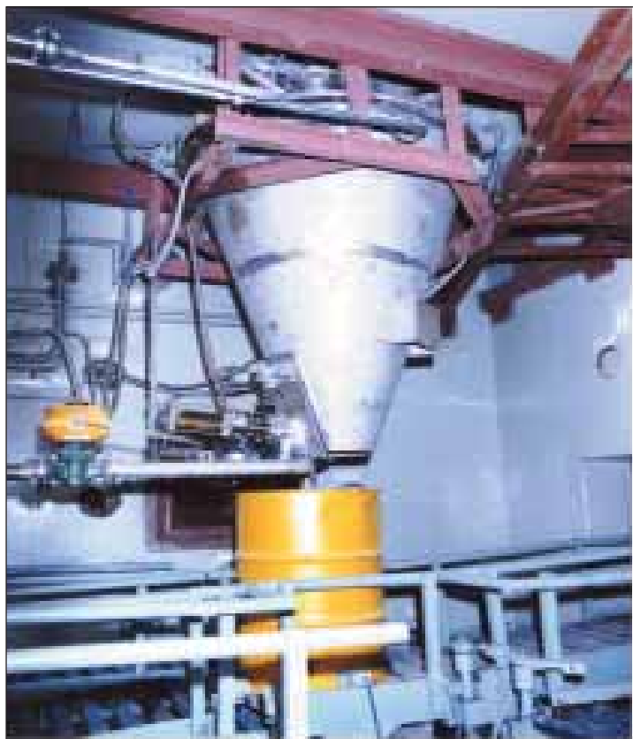
Cone mixer deployed at waste immobilisation plant, Trombay
