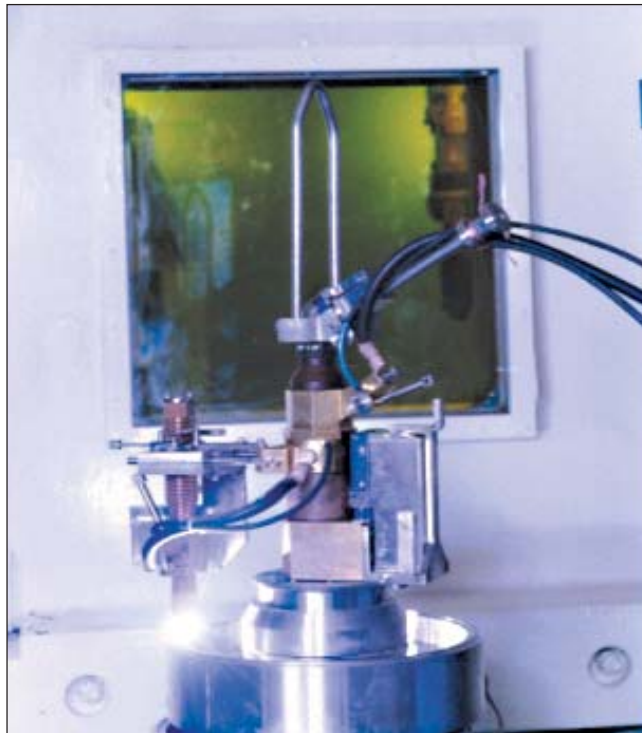
Remote welding of high level vitrified waste canister
