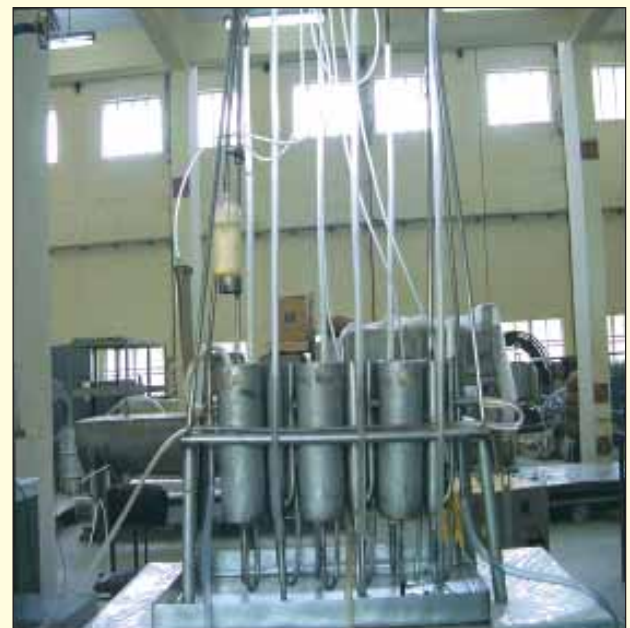
High efficiency ejector mixer settler
