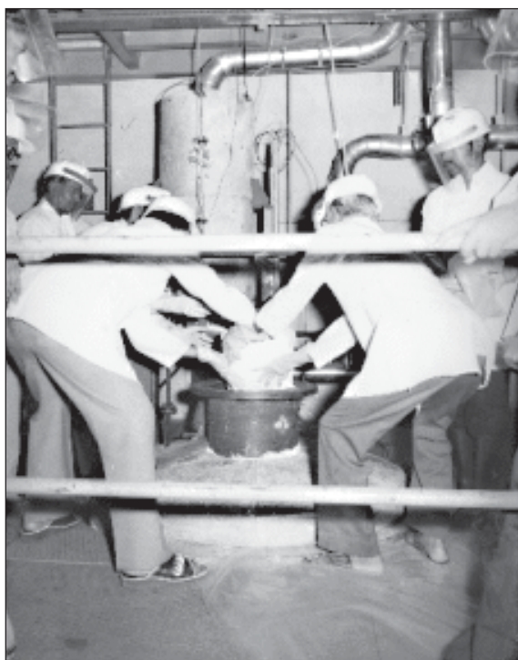
First charging of commercial sodium brick for purification
