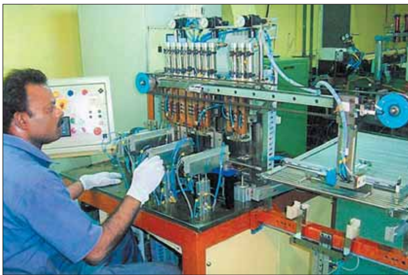
Integrated Appendage welding machine for 37 element PHWR Fuel — designed and fabricated in-house
