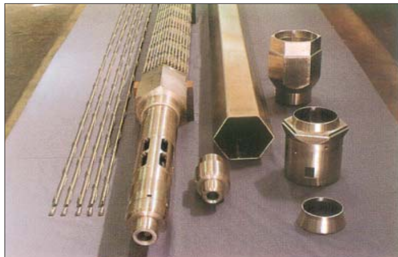
SS 316/D-9 hardware for fuel assemblies & core components for FBTR and PFBR
