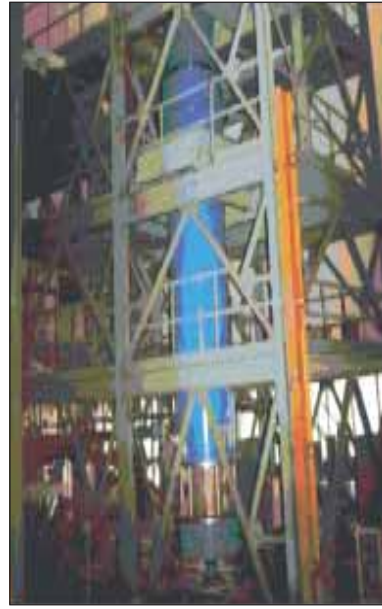
Centrifugal pump – rotor assembly test facility
