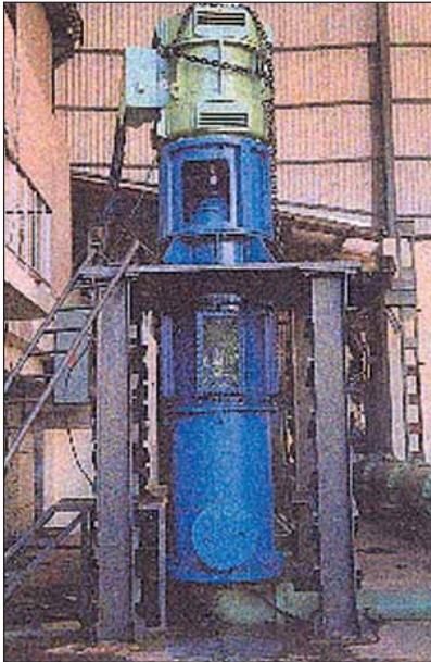
Centrifugal pump – model test facility
