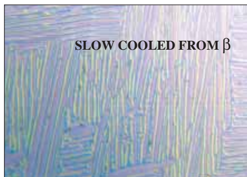
The thermo-mechanical treatments of the Ti-Ta-Nb alloy can yield either desirable (left micrograph) or deleterious structures, with corrosion rate in boiling HNO 3 as 0.3 and 1.5 mpy respectively
