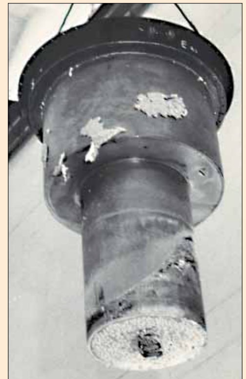
Sodium vapour deposition in cover gas region
