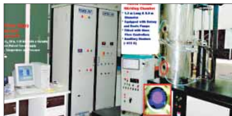
Flow chart (a) and industrial level nitriding set up developed at IGCAR (b). This set up can carry out the pulsed plasma nitriding on chrome-plated stainless steel PFBR grid plate sleeves. This has been used to demonstrate that the PFBR grid plate sleeves can be nitrided and the product- Cr_2N coating meets the specifications for the final use in PFBR.
