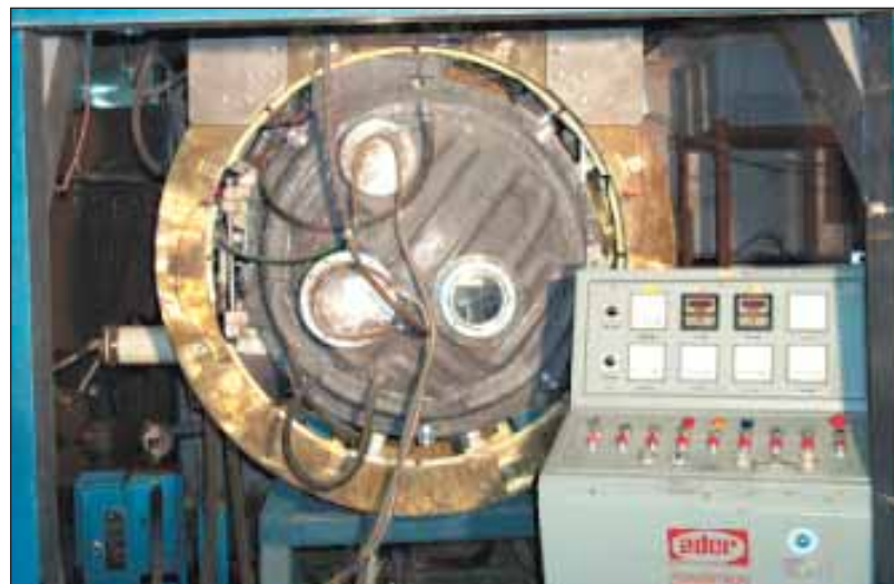
200 kW EB evaporation system
