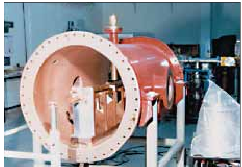
Inner view of the Low Power RFQ (LPRFQ). BARC was the first to develop this technology in the country
