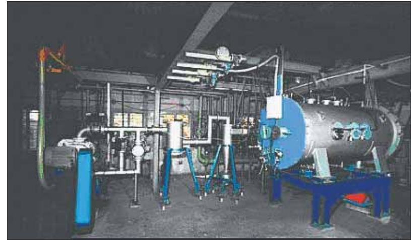
Controlled environment plasma spray unit at BARC
