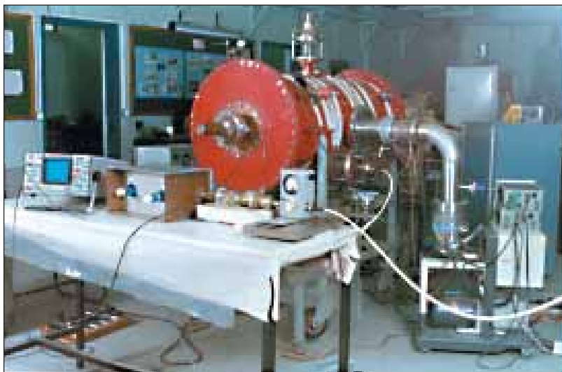
A View of LPRFQ in the commissioning phase
