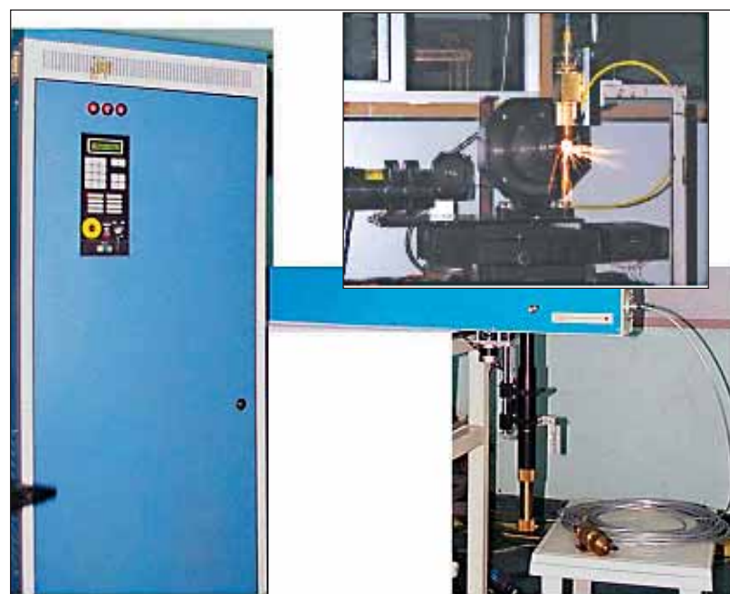
Industrial YAG laser with power supply and controls unit (Top right: Laser cutting of Zircaloy tube)
