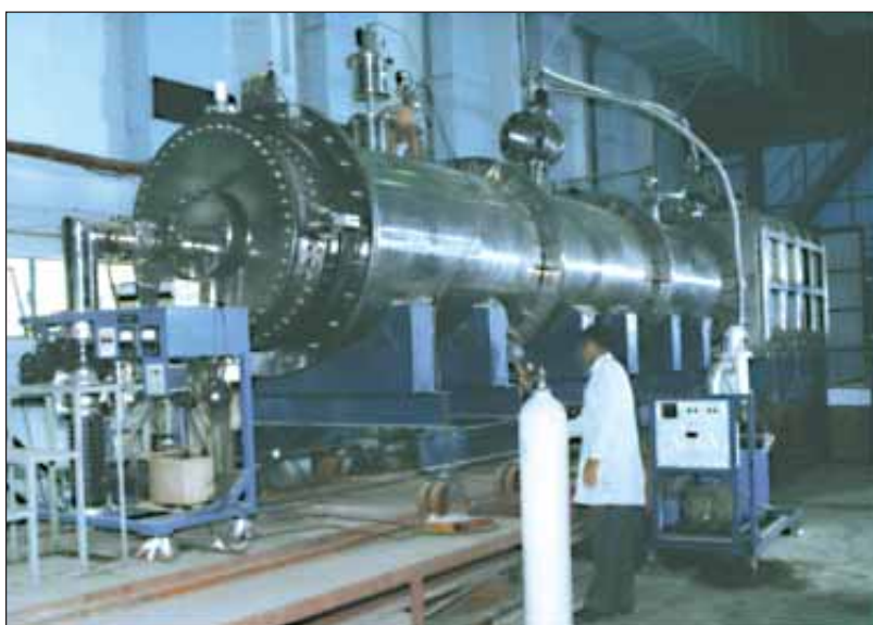
KALI-5000 Pulse Power System : It is the most powerful pulsed electron source designed and built indigenously in the country
