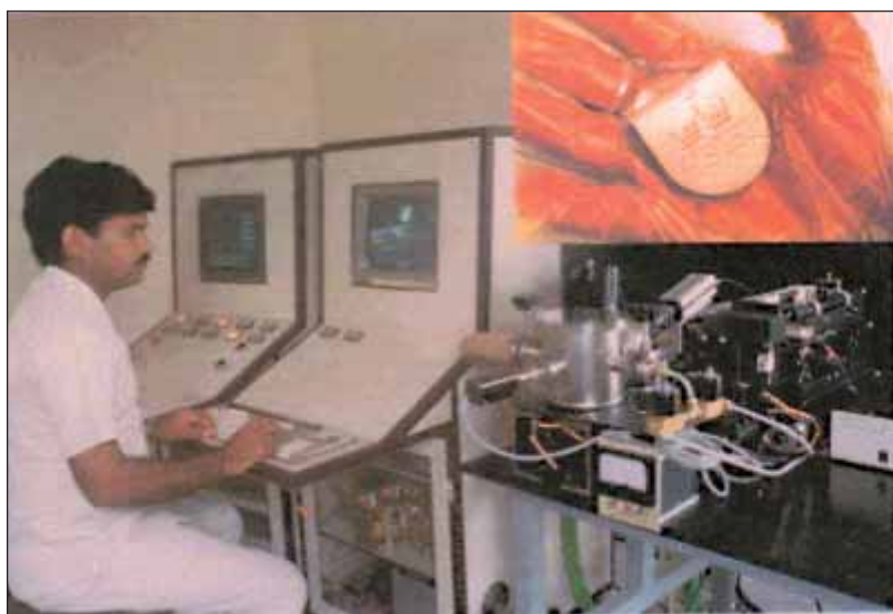
Automated pace maker welding station. Inset shows a welded pace maker
