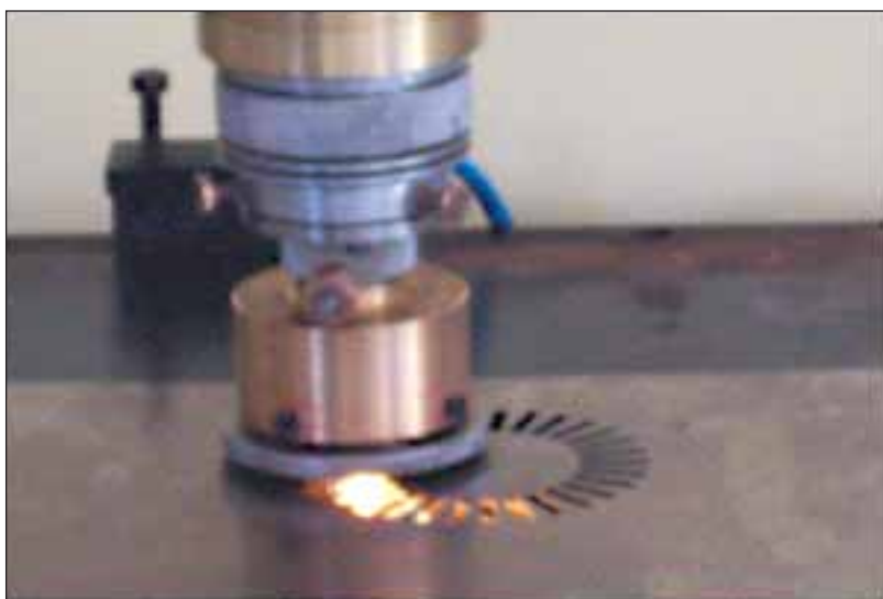
Laser cladding operation
