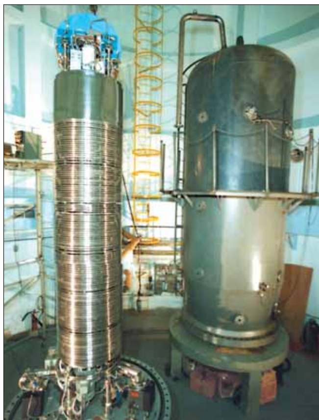
Folded Tandem Ion Accelerator (FOTIA) column and the tank developed at BARC
