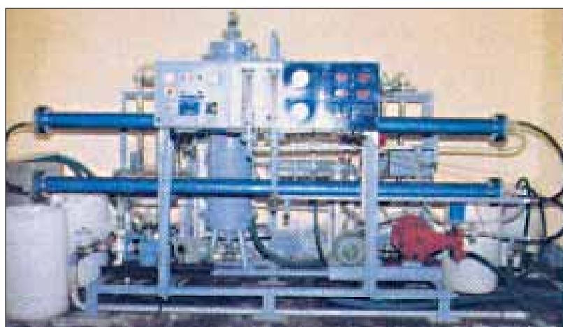
Reverse osmosis plant (capacity : 30 cubic metre per day) set up at Sheelgan village, district Barmer, Rajasthan
