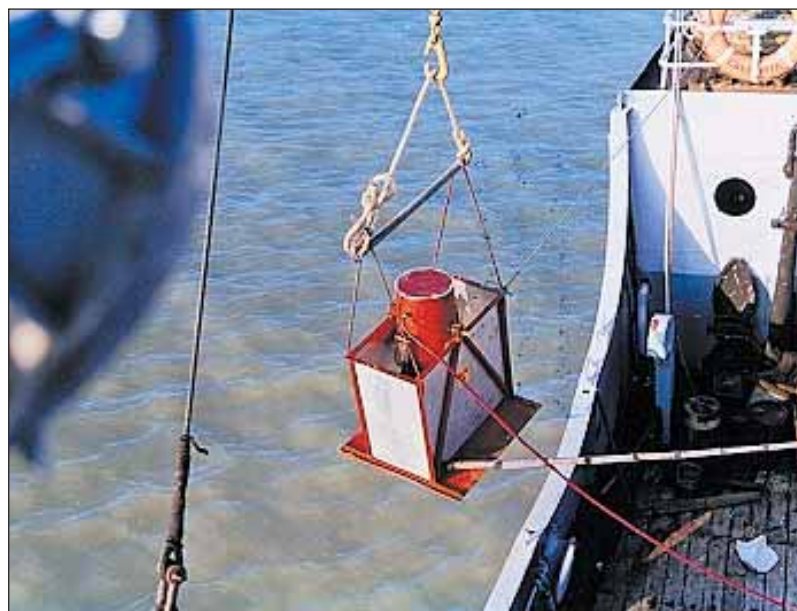
The radioisotope being injected for sediment transport studies at Hooghly river, West Bengal
