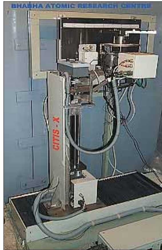
160 kV X-ray based experimental tomography system for industrial applications
