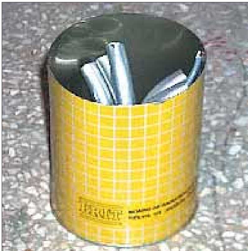
A thin metallic container partially filled with water [100mm(H) x 100mm(OD)] housing a section of welded aluminium curved tubes
