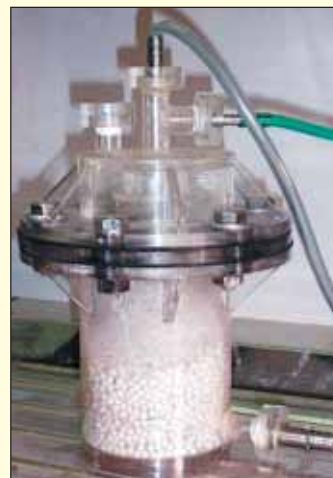
(a) Small test trickle bed reactor used in the experiment.
