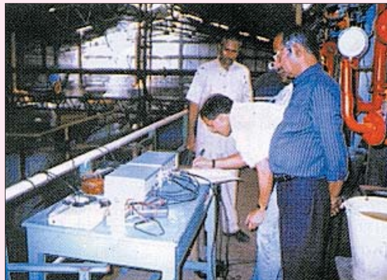
Radiotracer experiment for residence time distribution estimation in Sugar Industry.
