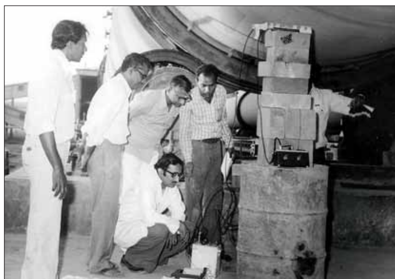
Radiotracer experiment being conducted at one of the cement factories near Coimbatore, for residence time distribution in the rotary kiln
