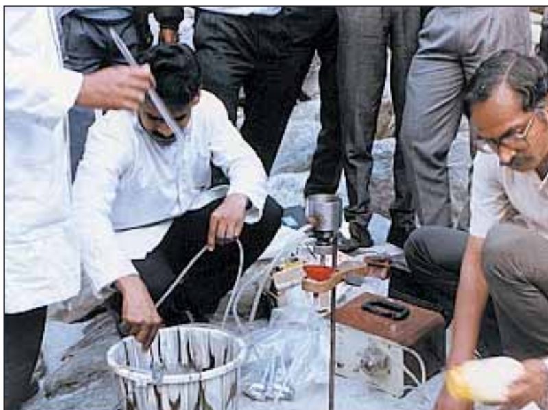
Isotope injection preparation in progress for studying discharge of Teesta River, Sikkim
