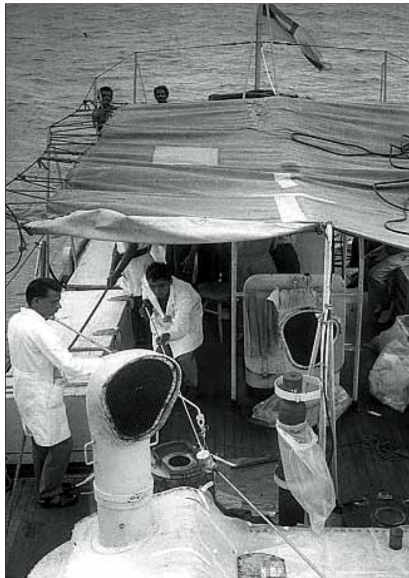
Radiotracer being removed from the lead shield for the first tracer experiment conducted on 14 th March 1959 for sediment movement of Bombay Harbour
