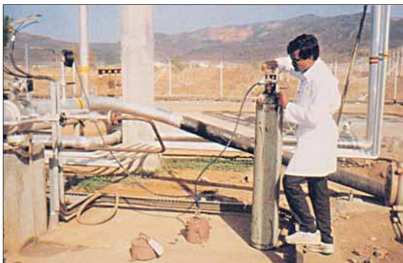
Leak location in underground pipelines using radiotracers
