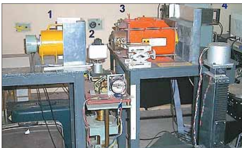
Cesium-137 gamma ray based industrial tomography system
