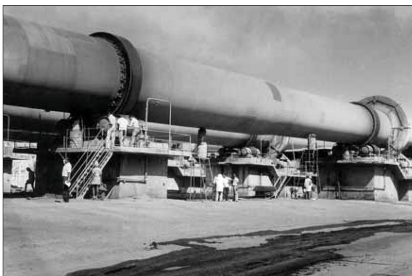
Radiotracer experiment being conducted at one of the cement factories near Coimbatore, for residence time distribution in the rotary kiln
