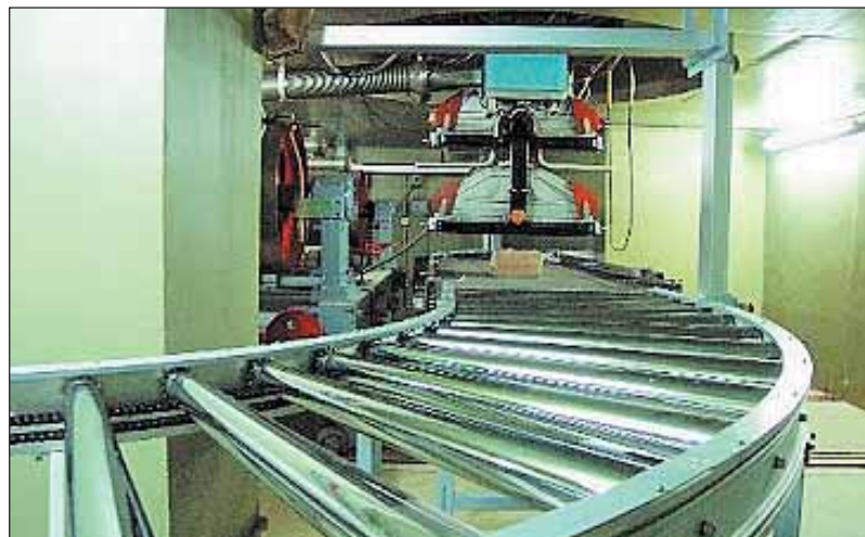
ILU-6 Electron beam accelerator with continuous conveyor system
