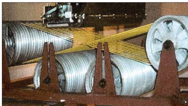
Electron beam crosslinking of wires
