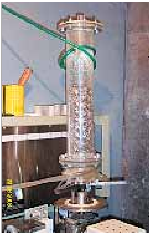
A test specimen column designed and fabricated for the X-ray based process tomography visualisation. The specimen is mounted on the experimental 160 kV X-ray ICT System
