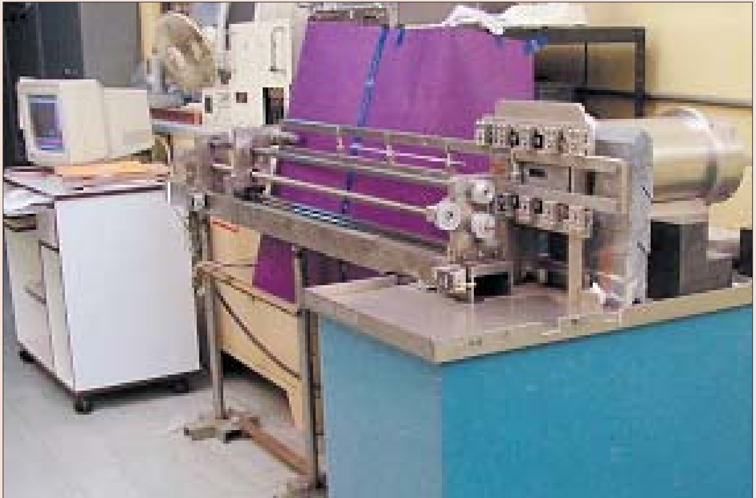
Fuel pin scanner for FBTR fuel pins
