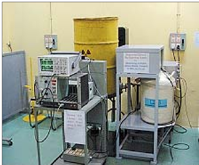
Segmented gamma scanning assembly for 200L waste drum to screen solid alpha waste
