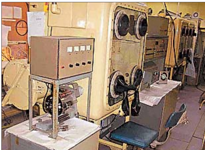
Glove-box adopted Atomic Absorption Spectrometer with electrothermal atomizer
