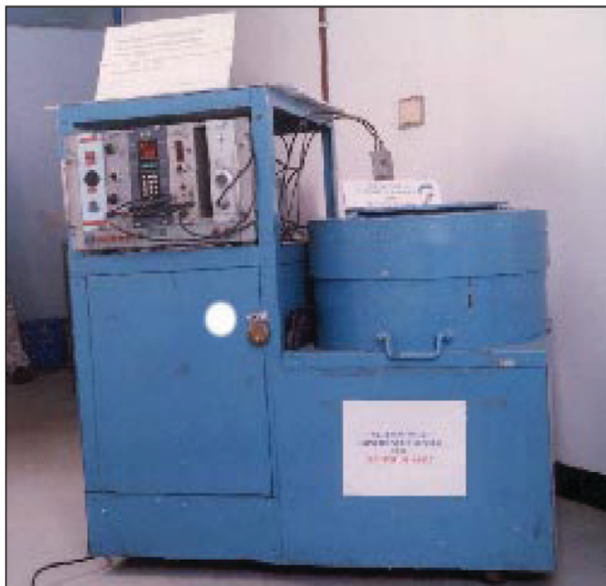
Neutron Well Coincidence Counter
