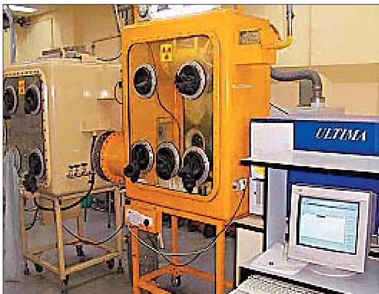
Glove-box adopted high resolution ICP Spectrometer
