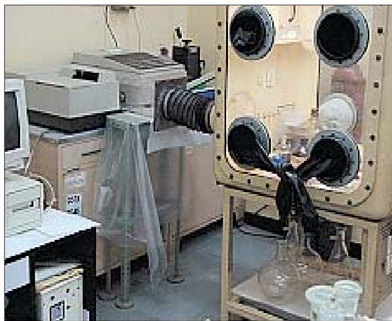
Glove Box assembly for Infra-red spectrophotometer
