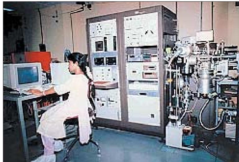
Mass spectrometer setup at Radiological Laboratory BARC, Trombay
