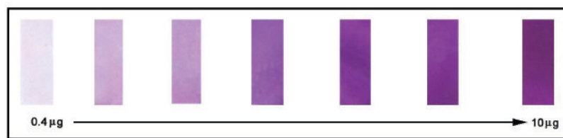
Variation of colour on polymer inclusion sorbent (PIS) as a function of amount of loaded Cr(VI)
