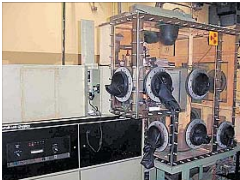
Glove-box adapted direct reading spectrometer equipped with DC arc and ICP excitation sources
