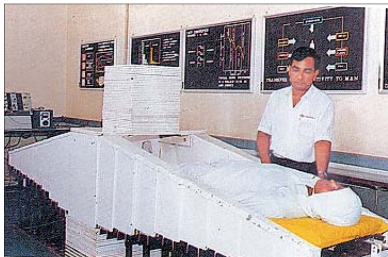
Shadow-shield bed whole body counter
