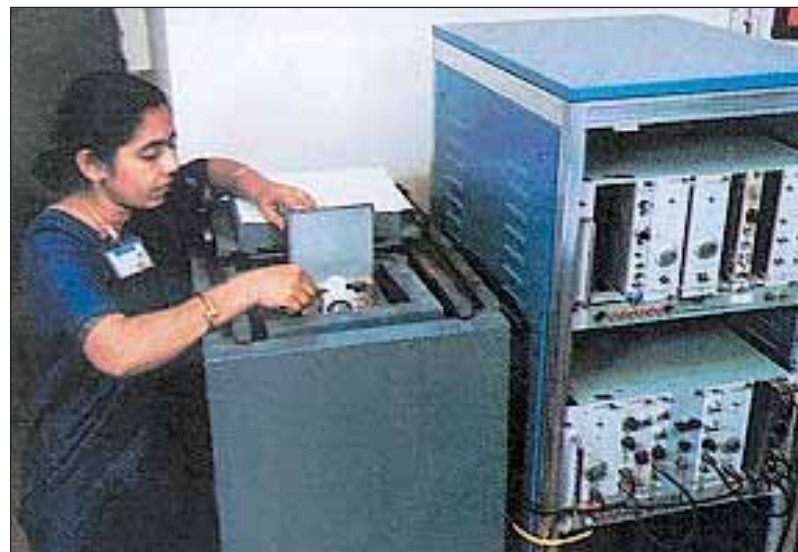
4 \pi - \beta,\gamma Coincidence counting system
