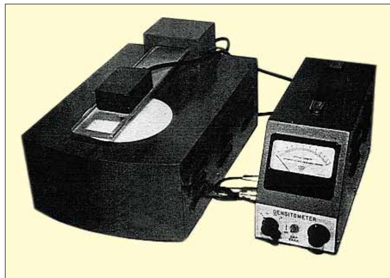
Densitometer developed at BARC for measurement of optical densities of films used in radiation measurement
