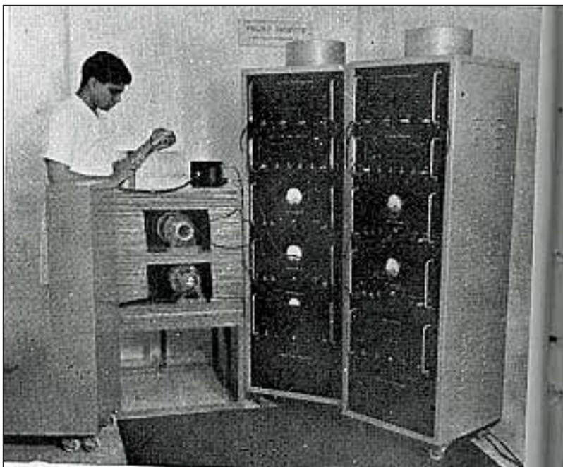
Low level counting equipment used in the early days for measuring small quantities of the fallout of isotope strontium-90 in milk and other food samples
