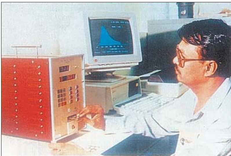
Personnel Dose Assessment with TLD in a TLD Laboratory
