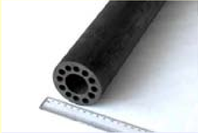
Prototype of fuel tube of CHTR made of high density graphite
