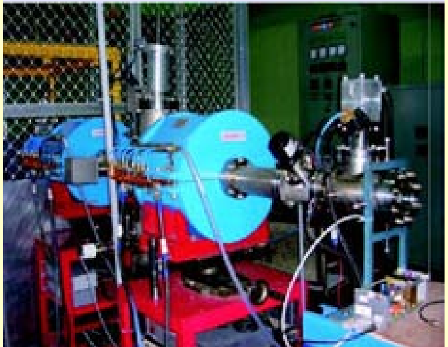
A test bench used to characterize Low Energy Beam Transport System. Two solenoids used for focussing and matching the beam
