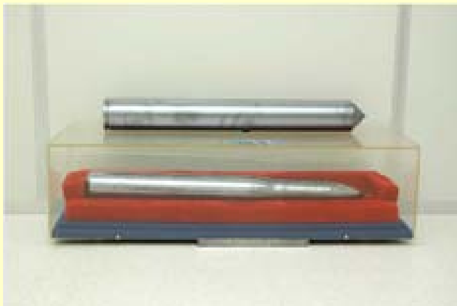
Poly-Silicon ingot (top) & single crystal ingot (bottom) (double size) pulled by FZ
