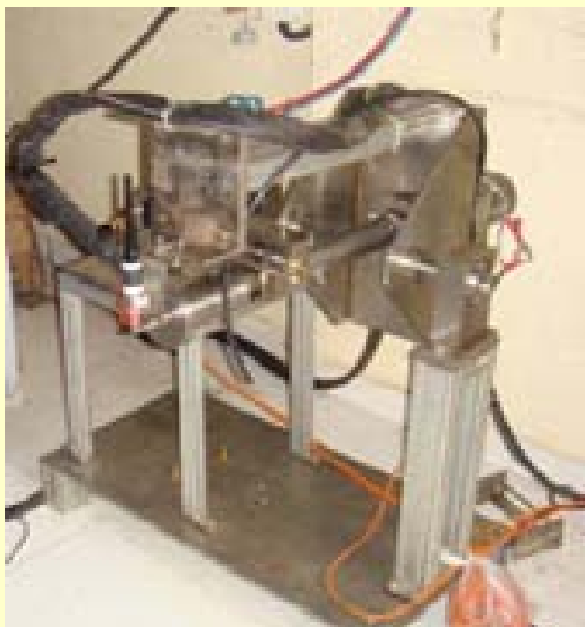
Remotely Operated Semi-automated Two-axis Welding Fixture
