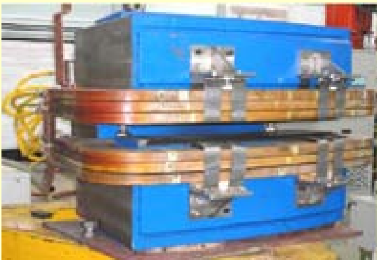
Pre-prototype dipole magnet core with 1.5mm thick low carbon laminations
