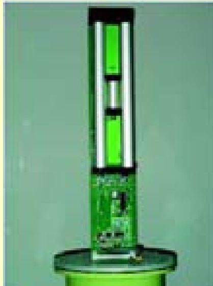
Interior of system with 3 GM tubes
