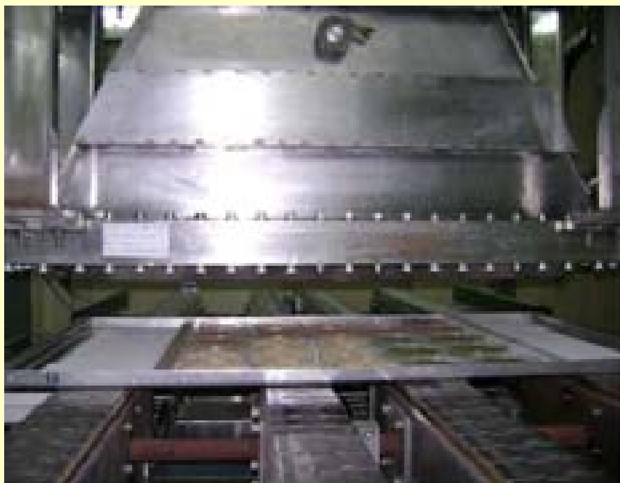
Seed in the irradiation tray on the conveyor belt ready for irradiation. Electron beam scanner of the accelerator is seen above the tray
