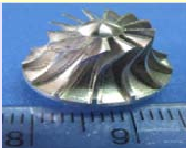
16 mm cryogenic turbine impeller
