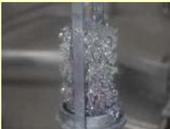
Uranium metal deposited on a solid cathode ( IGCAR)
