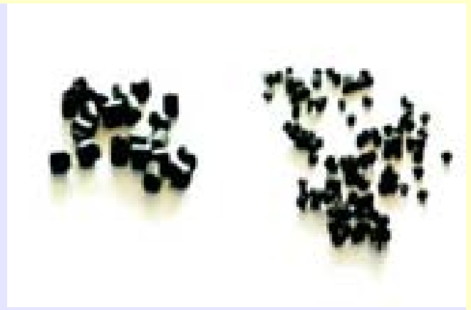
Six mm raschig ring shaped hydro phobic catalyst (earlier catalyst) and (right) 3 mm SS Dixon ring supported hydrophobic catalyst Improved Catalyst
