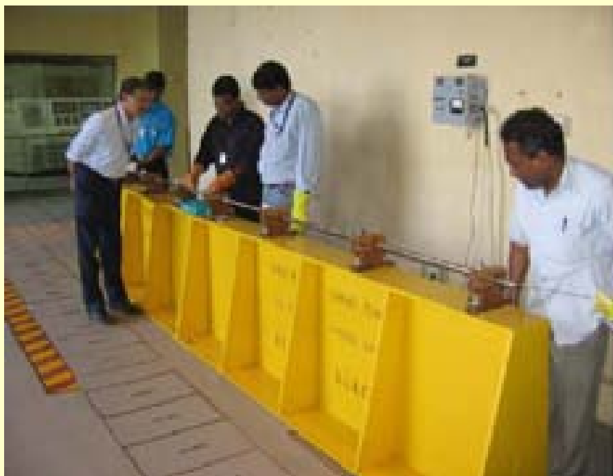
Extracting the irradiated activation foils from fuel pin assembly
