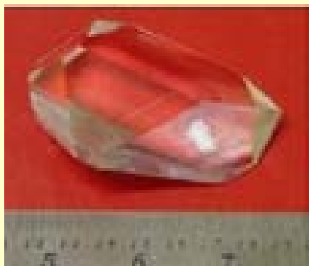
Transparent crystals of L-Arginine Phosphate monohydrate
