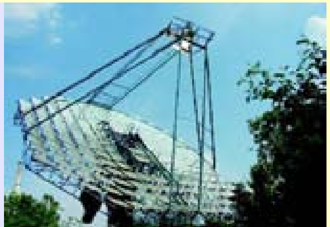
Solar Evaporator for steam generation at the Heavy Water Plant, Kota
