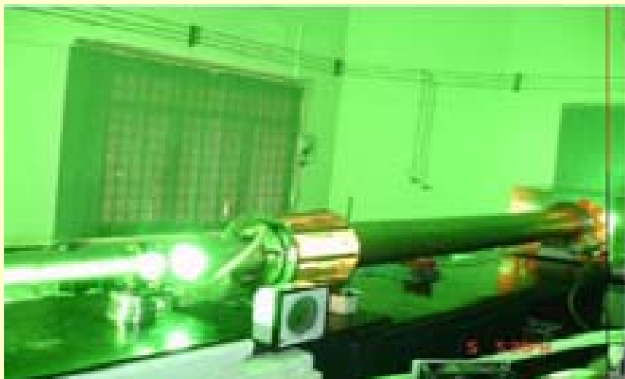
110W average power Copper-HyBrID laser
