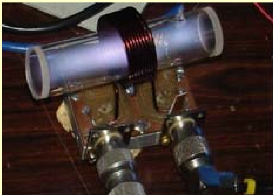
RF discharge in the Kr cell for Doppler-free signal of metastable Kr atoms
