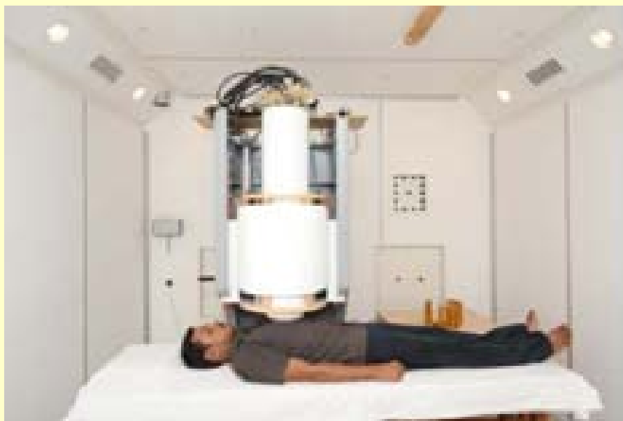
Channel SQUID based system for magnetocardiography
