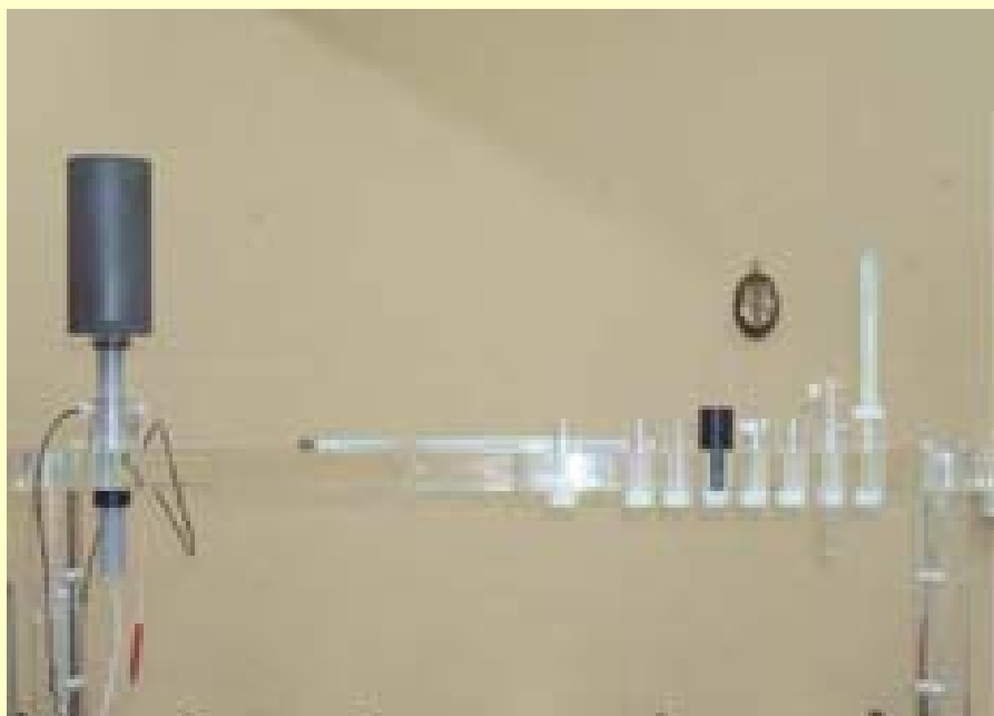
Experimental set up showing measurement of RAKR of ^{137}\text{Cs} and ^{192}\text{Ir} brachytherapy sources using in-house developed cylindrical graphite ionization chamber
