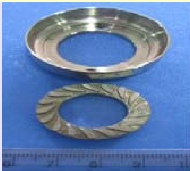
16 mm cryogenic turbine impeller (L) and nozzle components (R)
