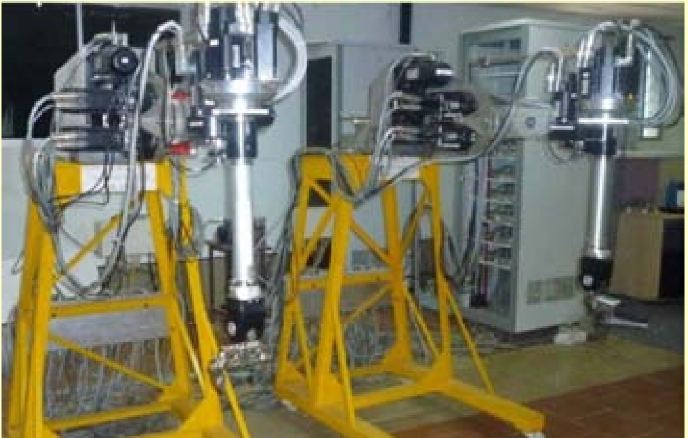
Slave and Master Arms of the Telerobot developed at BARC
