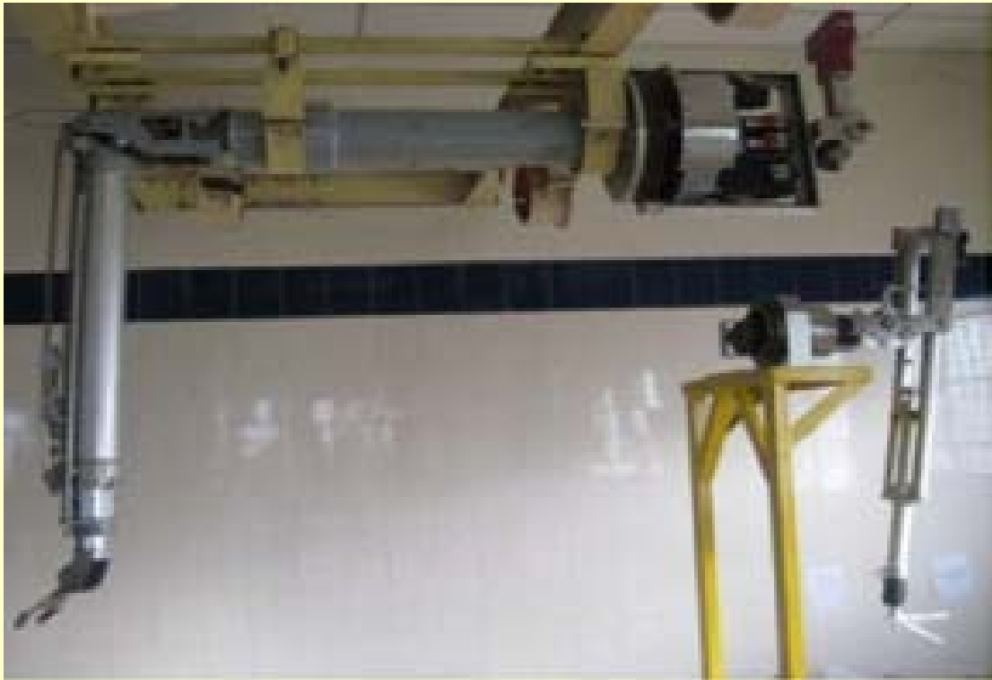
The Slave Arm and the Master Arm of Four-Piece Servo Manipulator
