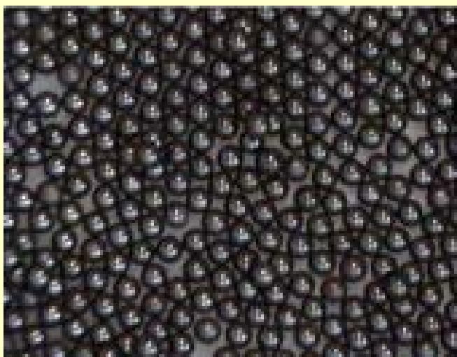
(U 0.47 , Pu 0.53 )O 2 microspheres sintered at 1450°C (BARC)
