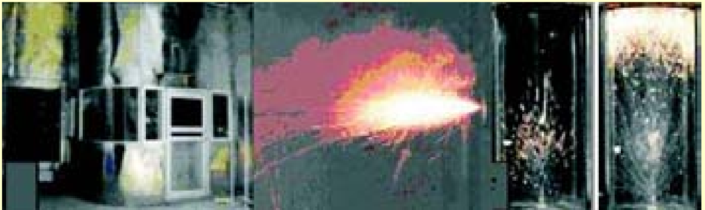
Simulation of sodium spray fire scenarios in MINA Facility
