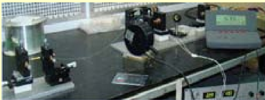
5 W Erbium -Ytterbium co-doped CW fiber laser at 1564 nm
