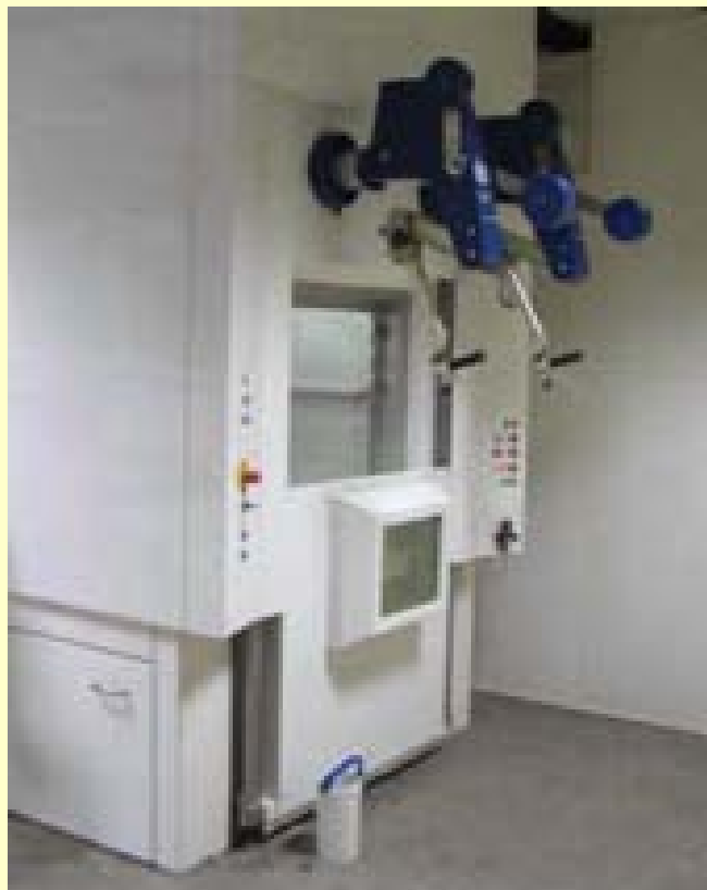
^{99}\text{Mo} - ^{99\text{m}}\text{Tc} Column Generator Plant
