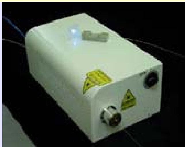
Compact high average power Nitrogen Laser for treatment of tuberculosis of lung and lymph node
