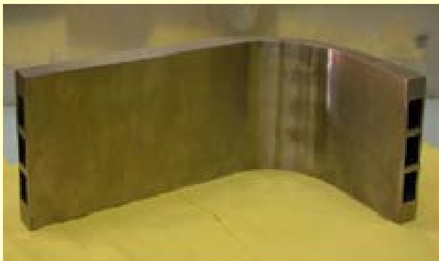
A 3-channel specimen of first wall of ITER TBM with a single bend fabricated through drilling and bending route
