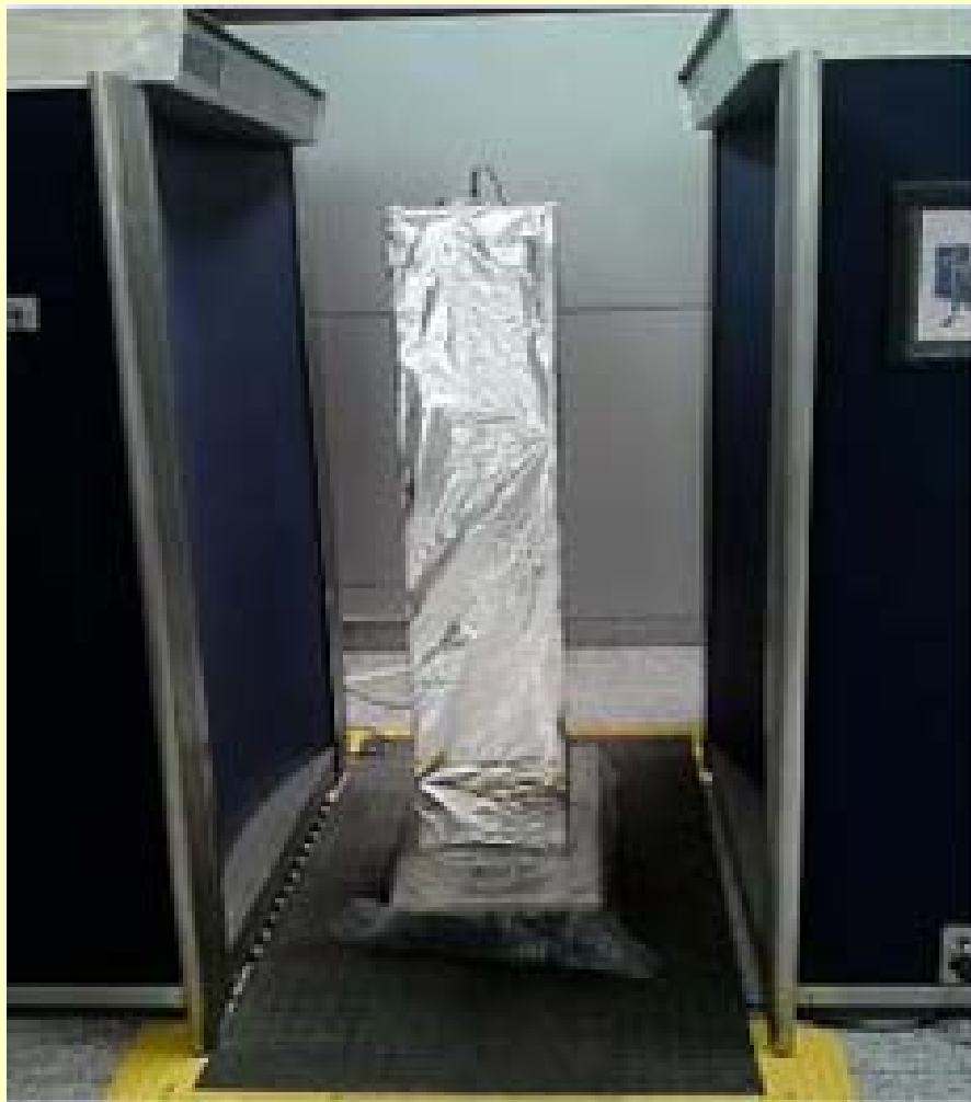
High sensitivity ion chamber for measurement of X-Ray dose from RAPI SCAN system
