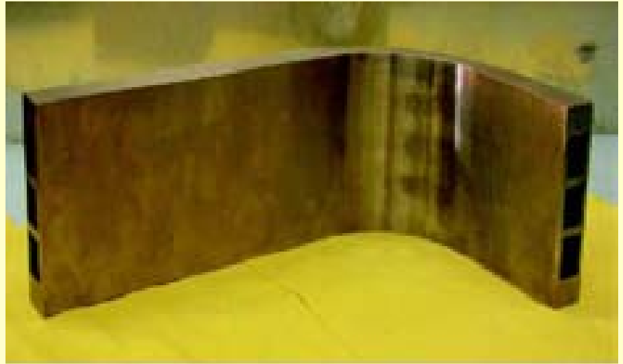
A 3-channel specimen of first wall of ITER TBM with a single bend fabricated through drilling and bending route
