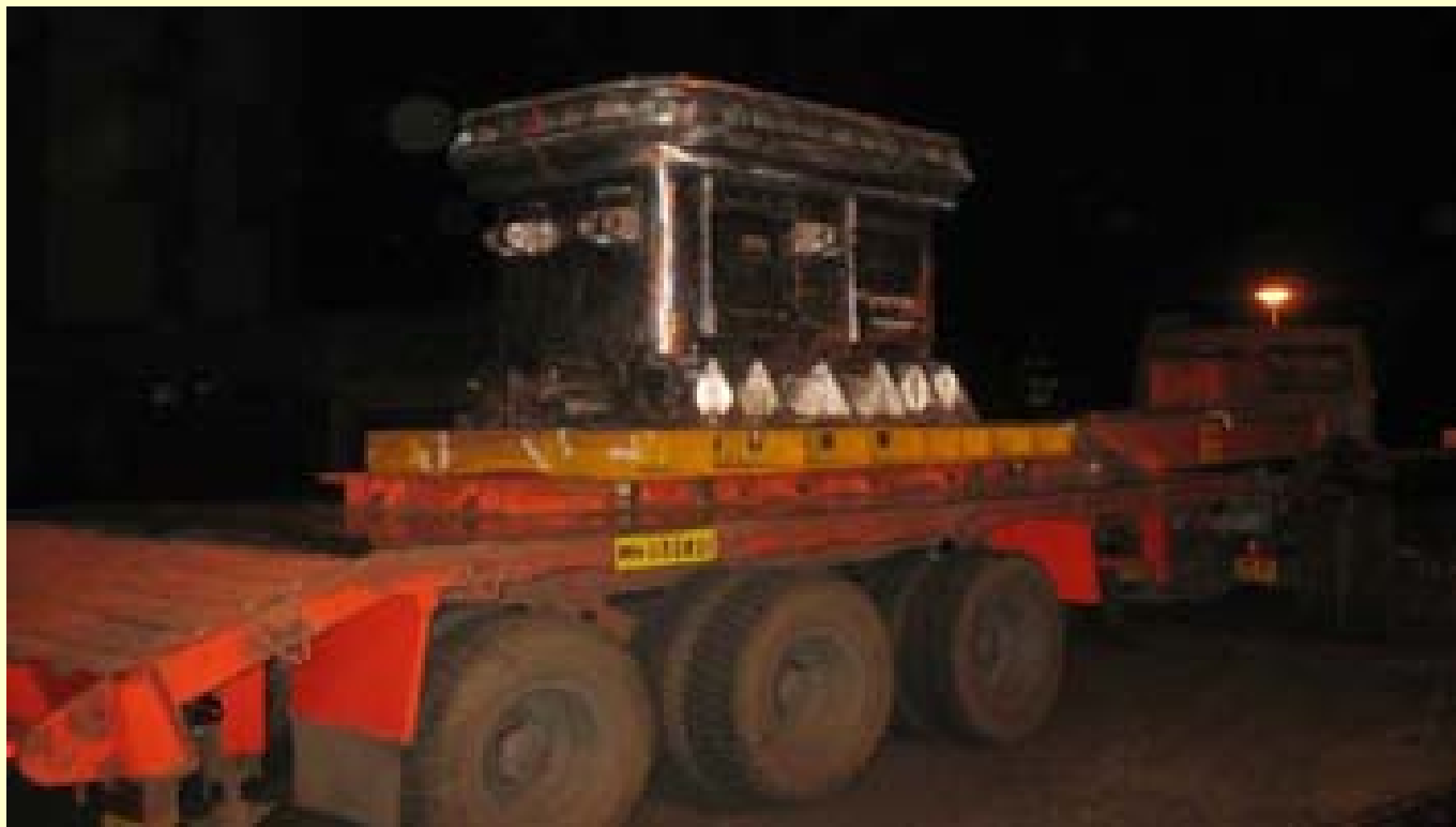
Shipping cask (along with tie down structure) used cages (holding the fuel assemblies) inside cask
