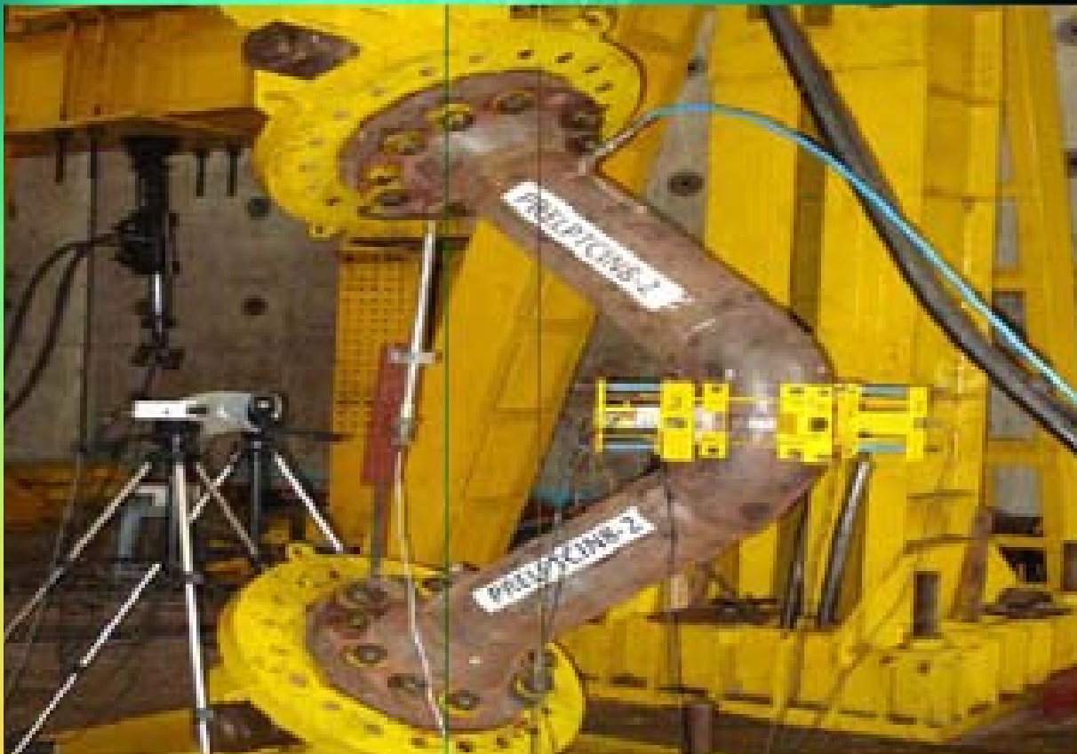
Study of fracture behaviour of pipe-elbow under different loading configurations by BARC at SERC, Chennai
