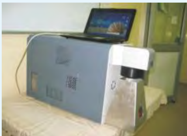
Laser Marker system installed at NFC, Hyderabad for serial number marking on the fuel elements
