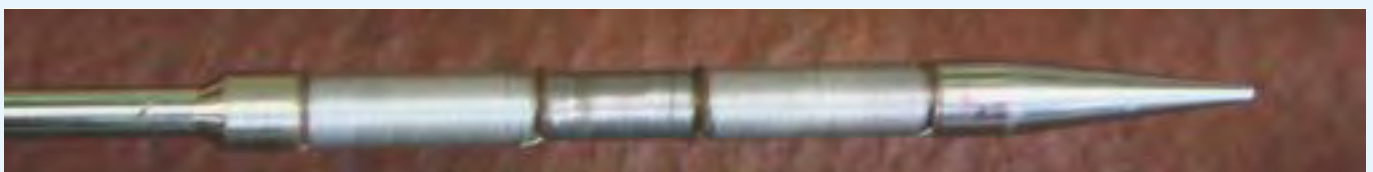
Eddy Current Flow Meter sensor for PFBR Pump
