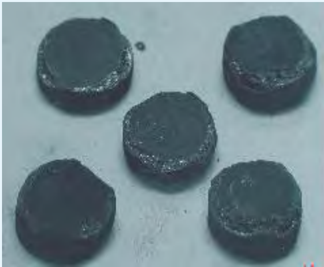
Uranium silicide pellets after synthesis
