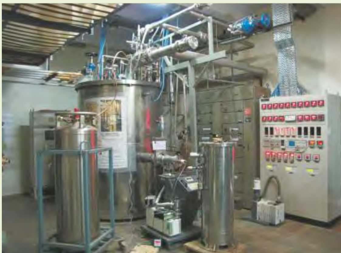
Helium liquefier under commissioning at Trombay
