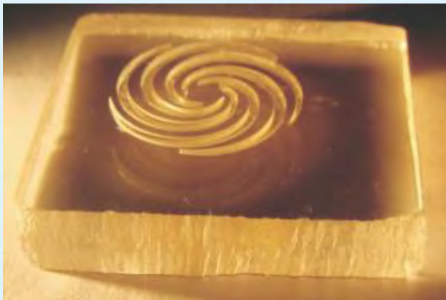
High speed bearing related structures developed by using X-ray lithography beamline on Indus-2
