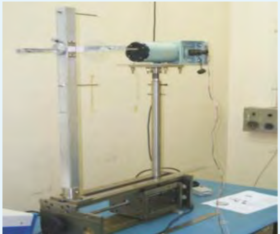
Standard Facility for calibration of beta monitors
