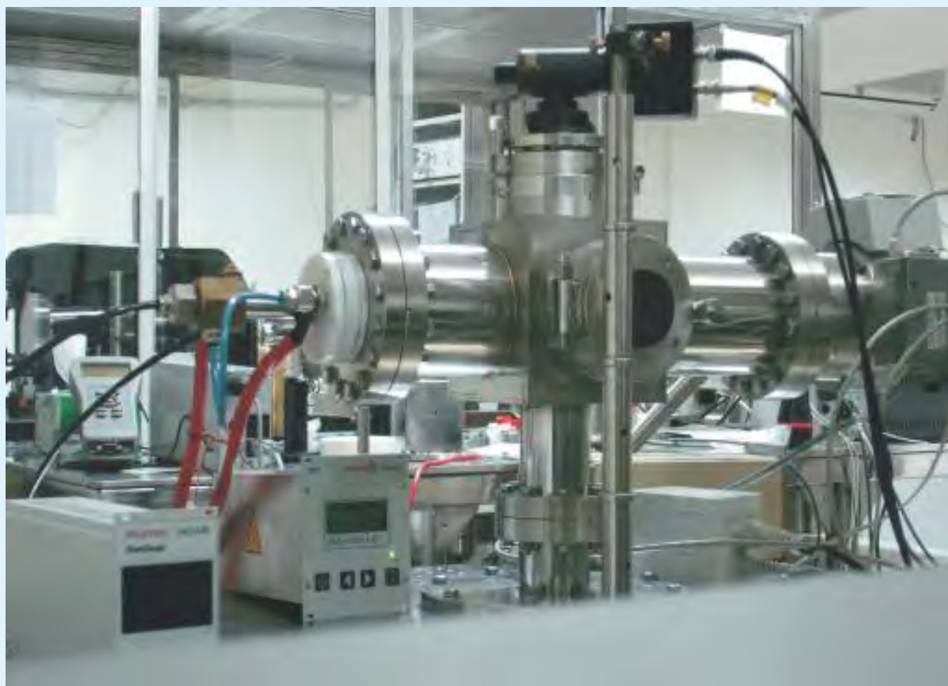
Atomic beam fluorescence spectrometer developed for high precision measurements of isotope shifts and hyperfine structure
