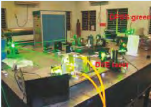
Dye laser Pumped by DPSS green laser beam
