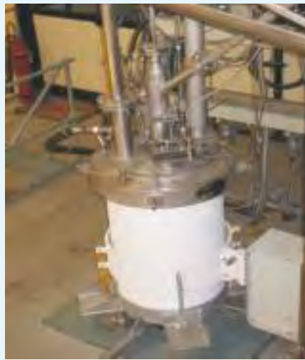
Plant adaptable cold crucible induction melter for Low Level Waste
