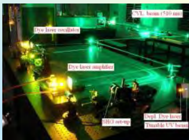
Tunable UV generation from copper vapour laser pumped dye laser beam developed at RRCAT
