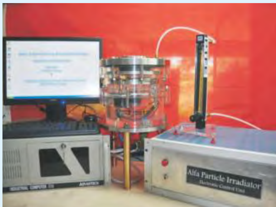
Complete set up of \alpha -particle irradiator with control unit
