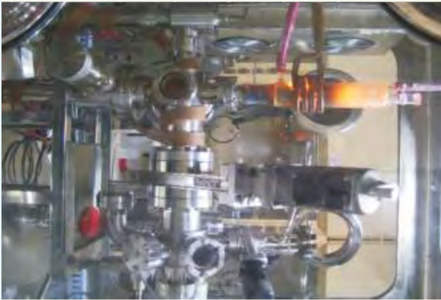
Glove box adapted TG analyser for Pu-fuels
