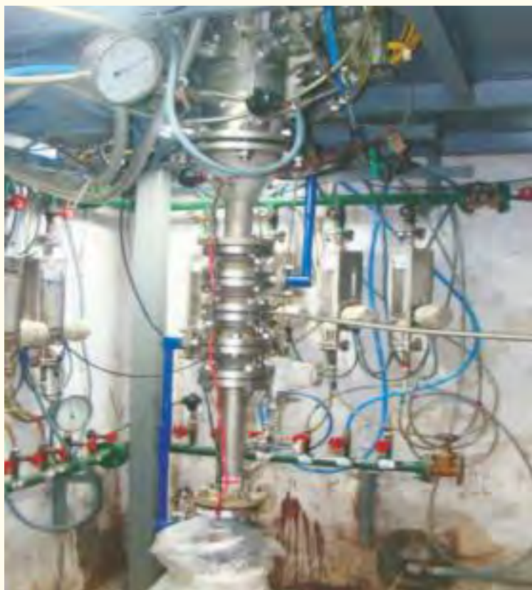
Plasma chemical reactor and the \text{UF}_4 powder collected from the bottom of the reactor
