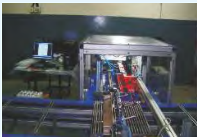
Machine vision based automated pellet inspection system installed at NFC, Hyderabad
