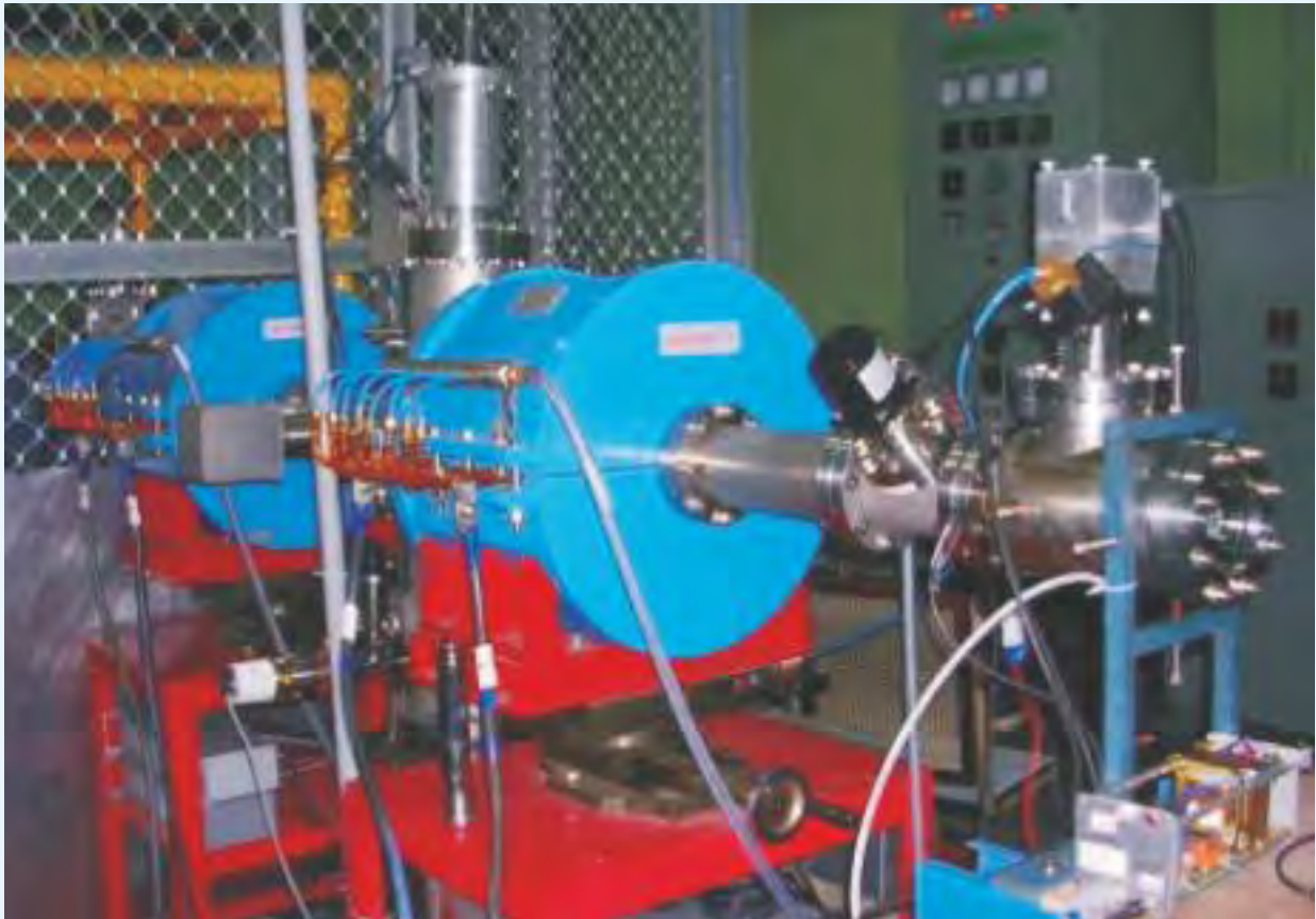
A test bench used to characterize Low Energy Beam Transport System.
