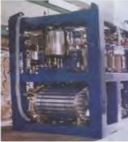
Compact Water Electrolyser Plant
