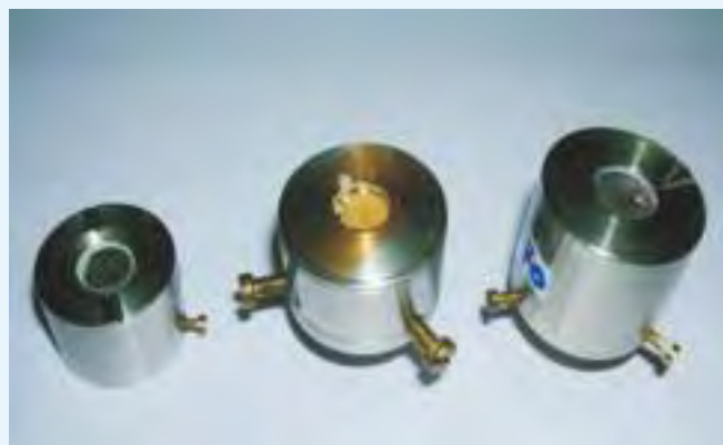
Diamond film based alpha particle detector developed at BARC
