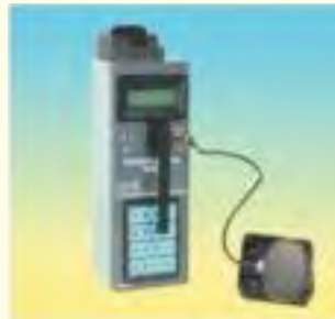
Detectors: GM tube Type: 7134 LND
