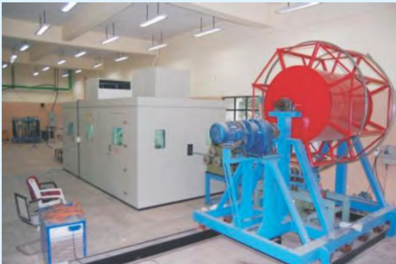
On-line cable-in-conduit-conductor (CICC) fabrication facility at Trombay where fabrication of 100m long 30kA Nb-Ti based hybrid CICC is in progress
