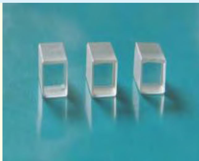
Elements fabricated from Nd:YVO 4 crystals
