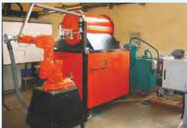
TEA CO 2 laser-based paint stripping system and paint stripping in progress
