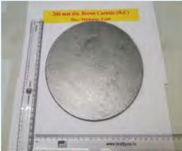
Vacuum hot pressed B 4 C disc
