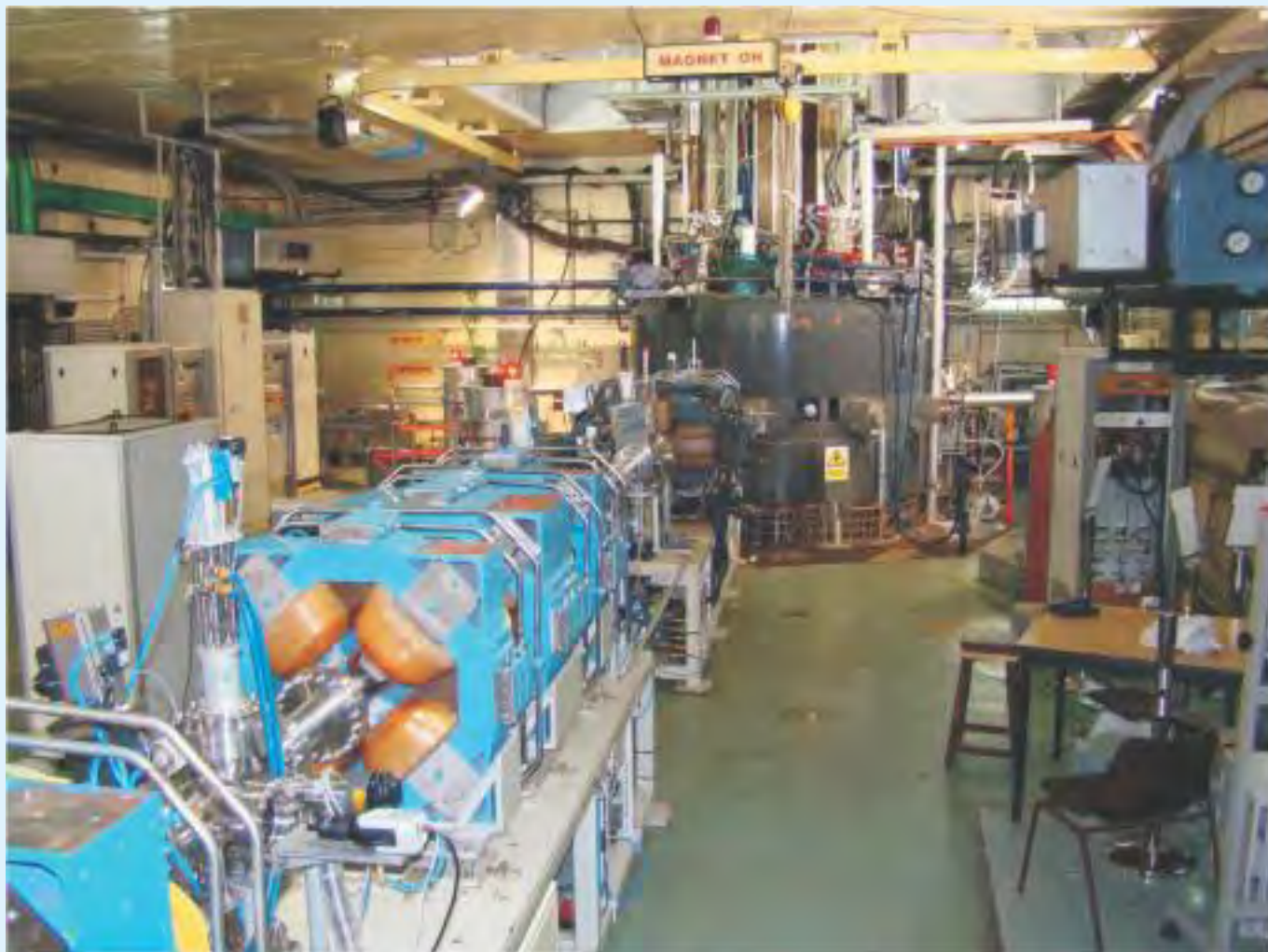
K-500 Superconducting Cyclotron with one of its external beam lines
