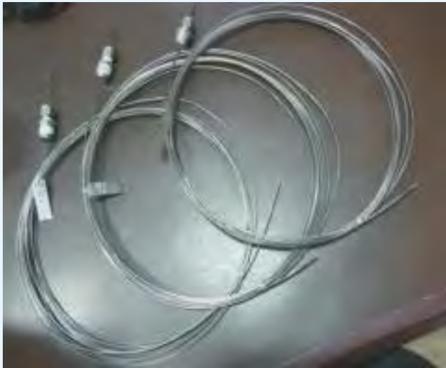
Successfully developed indigenous 3-pitch integral Self-Powered Neutron Detectors (SPNDs) for 700MW Project along with panel for in-pile testing at TAPS-4
