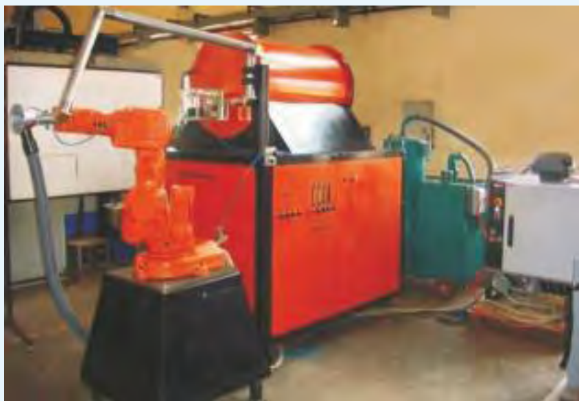
TEA CO 2 laser-based paint stripping system and (right) Paint stripping in progress
