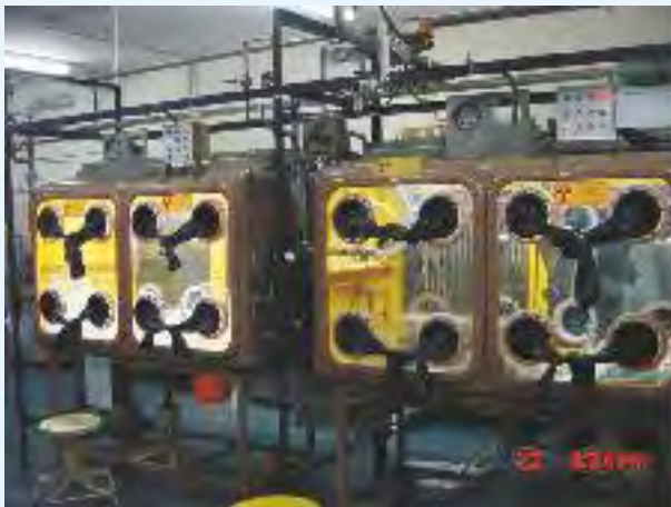
Mixer-settler facility used for flow sheet development studies with TiAP for fast reactor fuel reprocessing
