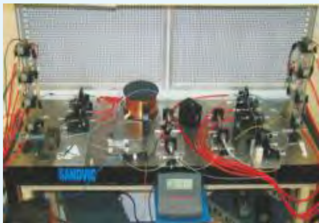
In-house developed 100 W single transverse mode CW fibre laser
