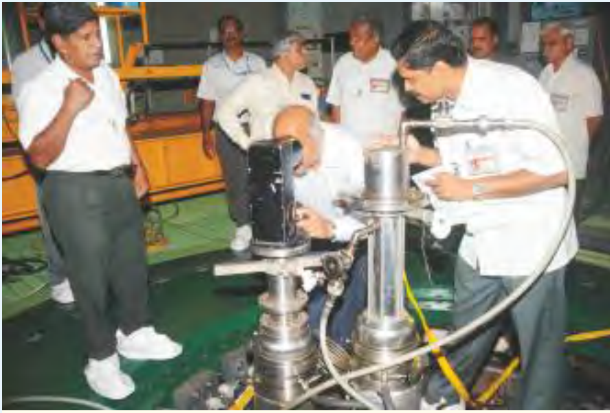
Internal inspection of reactor using periscope
