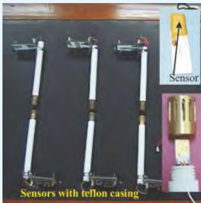
Humidity Sensors for leakage detection system in main steam line for PHWRs
