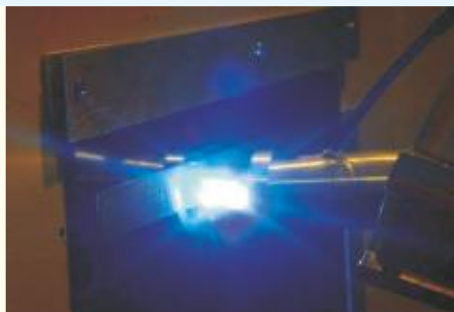
TEA CO 2 laser-based paint stripping system and paint stripping in progress
