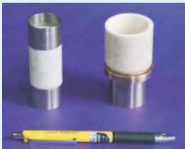
50mm dia ceramic-to-metal seal
