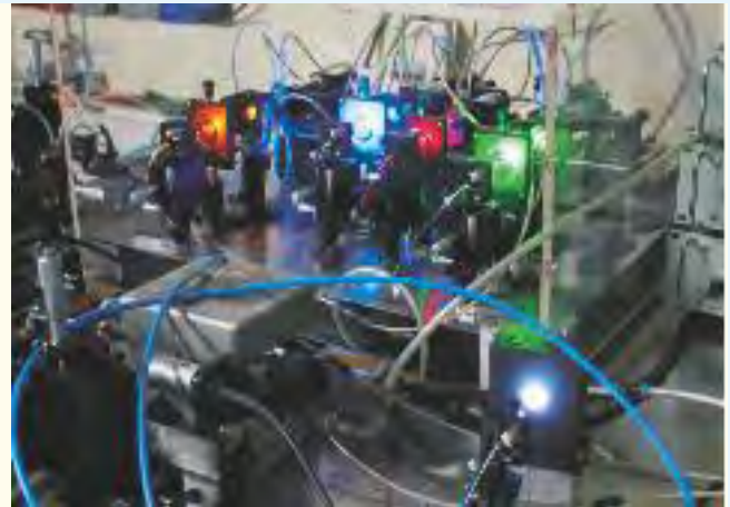
White light beam generation by combining of RGYB laser
