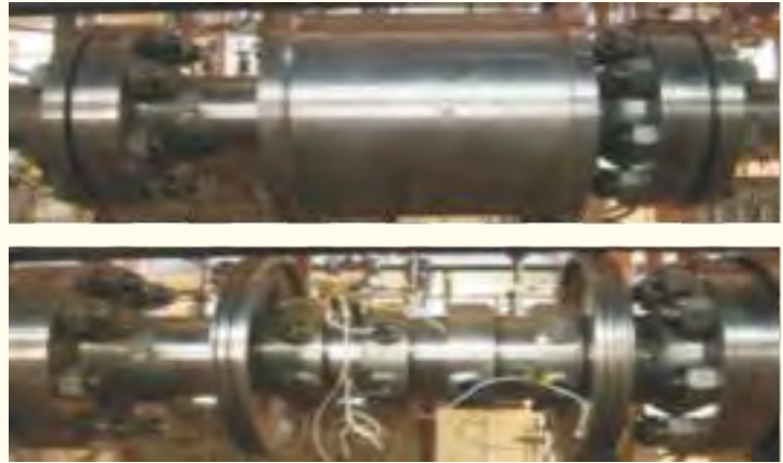
Three Channel Ultrasonic Flow Meter for Feed Water Flow Measurement Full Assembly (top) and Internal View (bottom)
