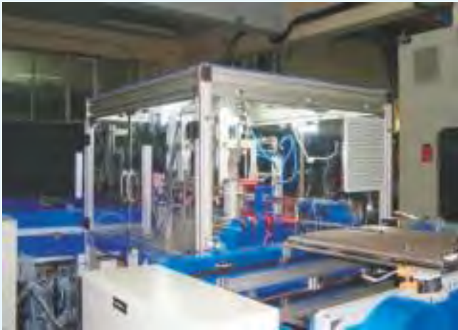
Automated Pellet Inspection System installed at NFC, Hyderabad
