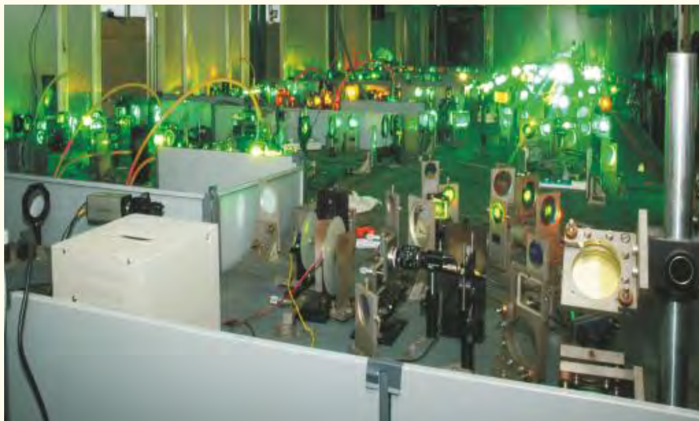
Copper vapour lasers pumped dye laser system
