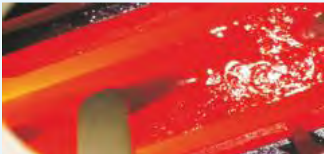
Molten glass pool inside the oblong shaped Metallic melter
