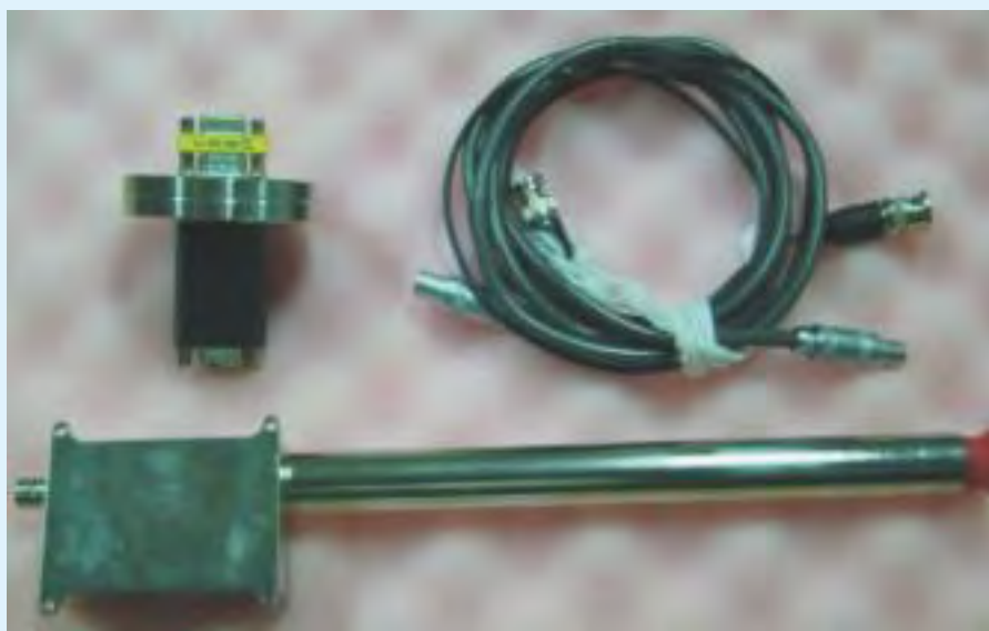
X-ray detector with feed through and cabling
