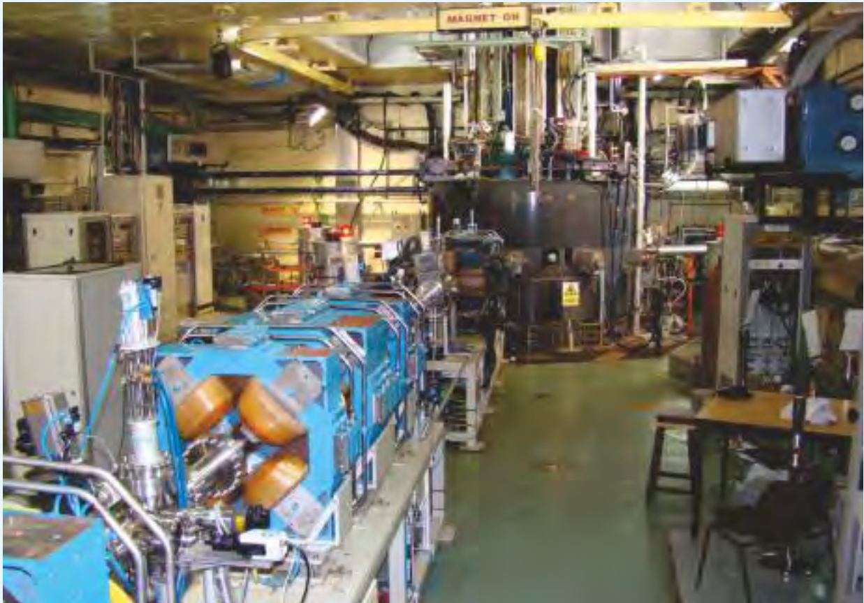
K-500 Superconducting Cyclotron with one of its external beam lines, at VECC, Kolkata
