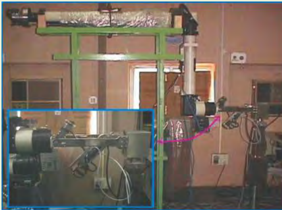
Hot cell Visual Metrics System Tele-Robot Operated Periscope at Trombay
