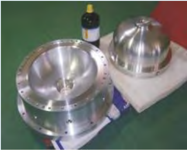
650 MHz superconducting RF cavity forming Dies
