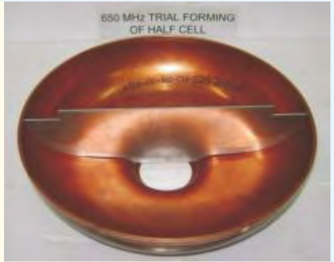
Formed half cell-inside view with inspection template also in view
