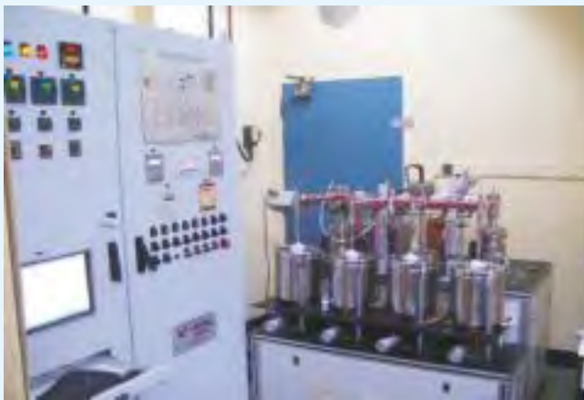
Hot Vacuum Extraction-Quadrupole Mass Spectrometer
