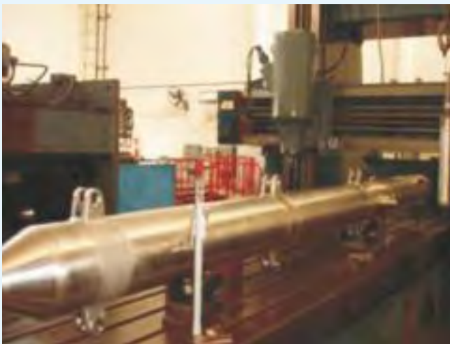
Machining of guide roller bracket of transfer pot
