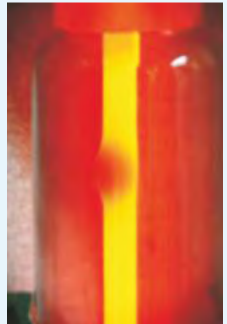
Ballooning of fuel pin : A fuel pin that was subjected to impulse heating to around 1200 deg Celsius
