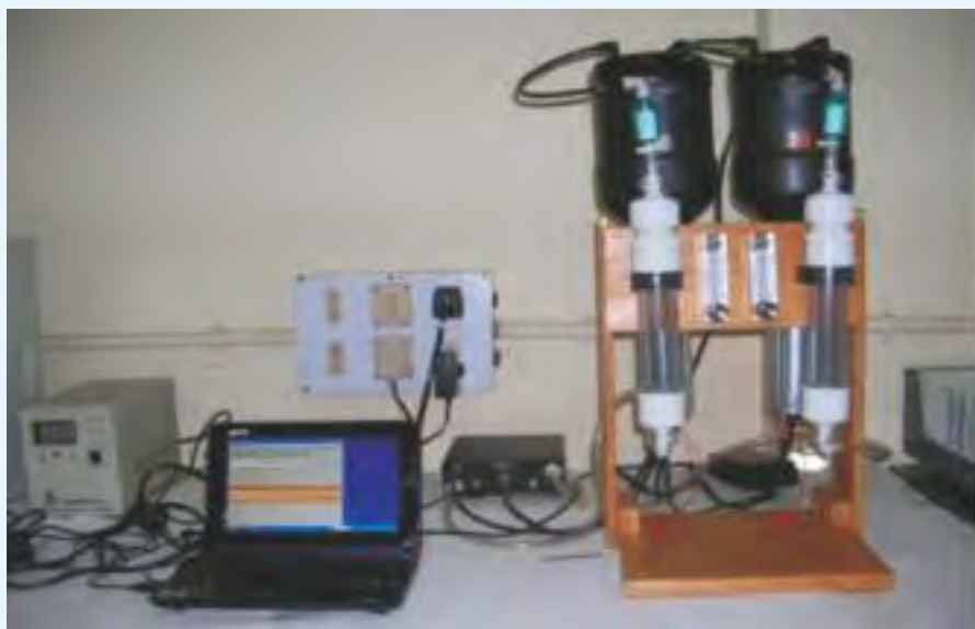
Delayed coincidence counter for measurement of Radon-223 and Radon-224
