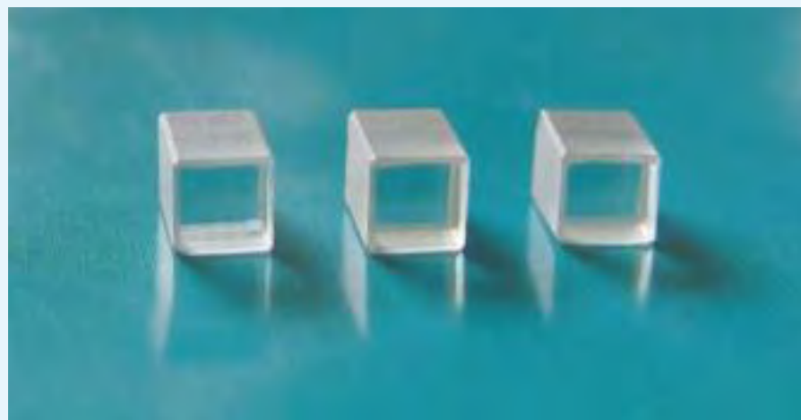
Elements fabricated from 0.3 atom % \text{Nd:YVO}_4 crystals
