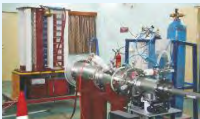
Capillary discharge X-ray laser system and right the spectrum of the emitted laser radiation
