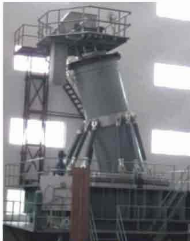
Inclined Fuel Transfer Machine for PFBR designed by BARC
