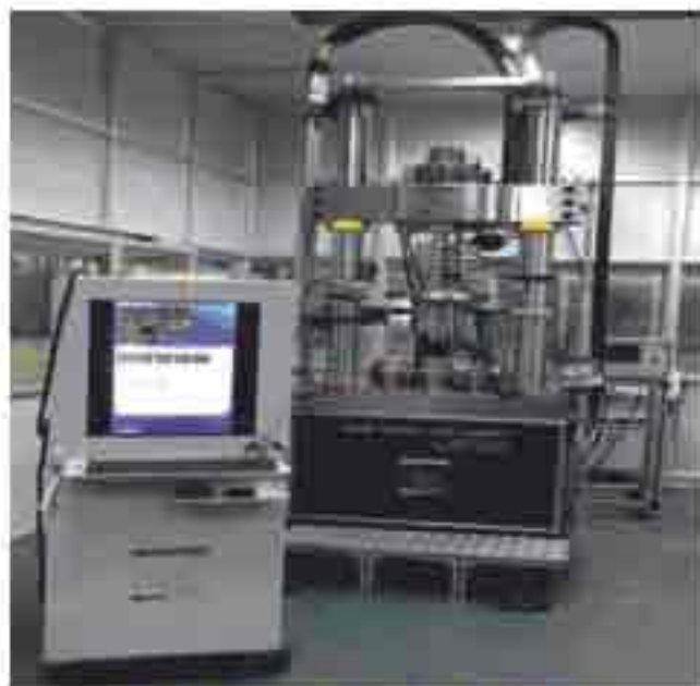
High-temperature combined axial and torsion testing system
