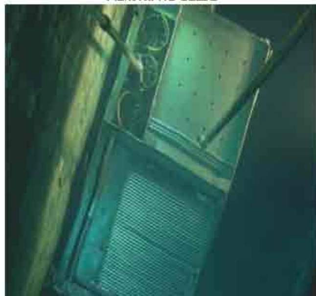
Cobalt-60 Rack Design of NIPRO Irradiator
