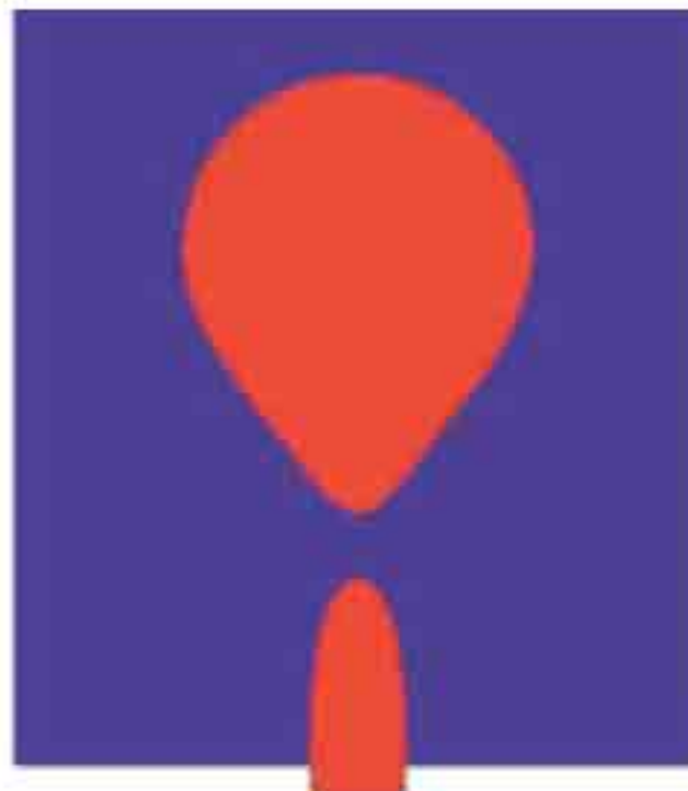
Drop formation at a single hole, a snapshot from numerical simulation
