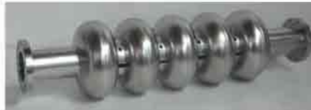
1.3 GHz five-cell superconducting RF cavity
