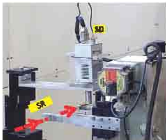
XRF-microprobe beamline used for measuring spot size of the focused Indus-2 photon beam
