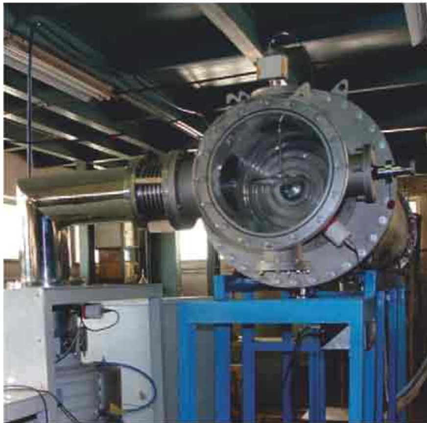
1kJ Rep rate Marx system with Reflex developed at BARC
