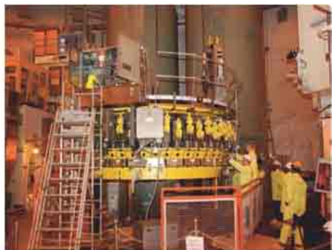
Multi Stud Tensioner (MST) for RPV sealing at Kudankulam Nuclear Power Project-1
