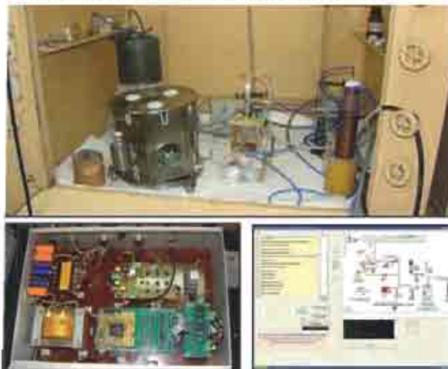
The AUTOSOLEX radiochemical process assembly Inside fumoid Screenshot of PC base GUI for AUTOSOLEX control AUTOSOLEX electronics assembly inside 19" rack
