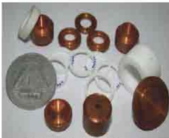
Penning Ion Trap Electrode Assembly fabricated at VECC
