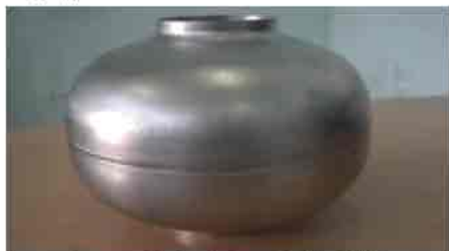
Laser welded prototype 1.3 GHz SCRF cavity made of niobium half cells
