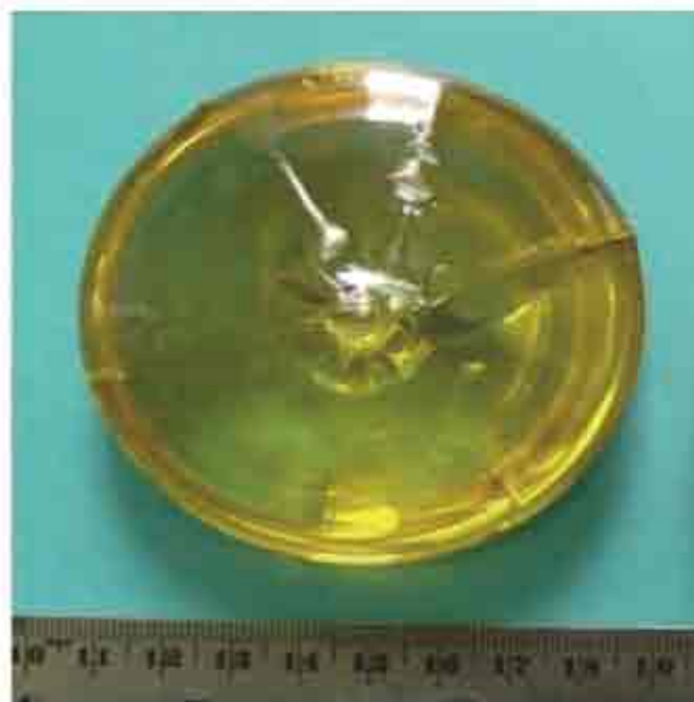
Growth of 70 mm diameter congruent lithium niobate single crystal
