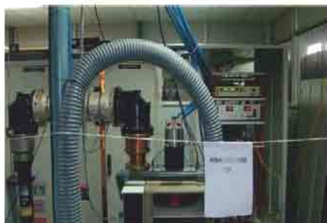
High power test of IOT based RF amplifier developed at VECC
