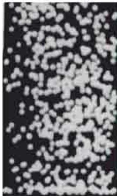
X-ray radiograph of compact showing the distribution of kernels in the matrix.
