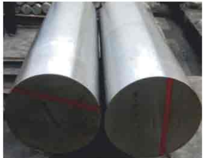
520 mm Ø Arc Melted and Machined Ingots
