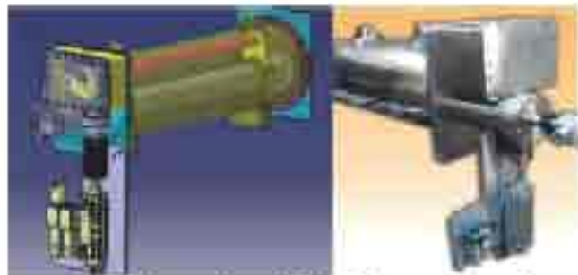
Innovative neutron shutter for beam lines of superconducting cyclotron
