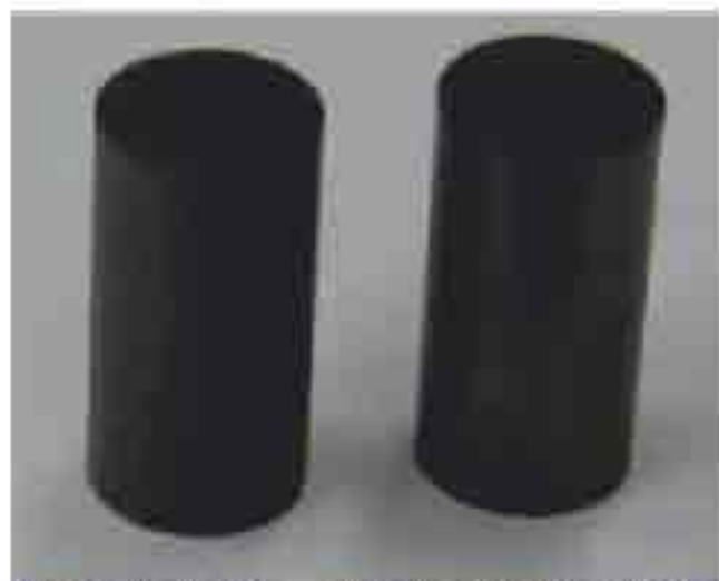
CHTR fuel compacts with 25 vol% TRISO coated ZrO_2 surrogate kernel
