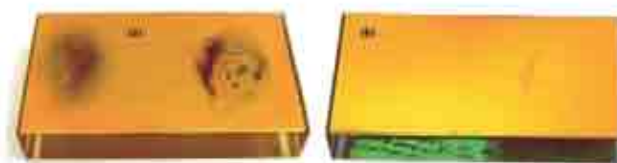
Pulse compressor grating, a) before and b) after RF plasma cleaning
