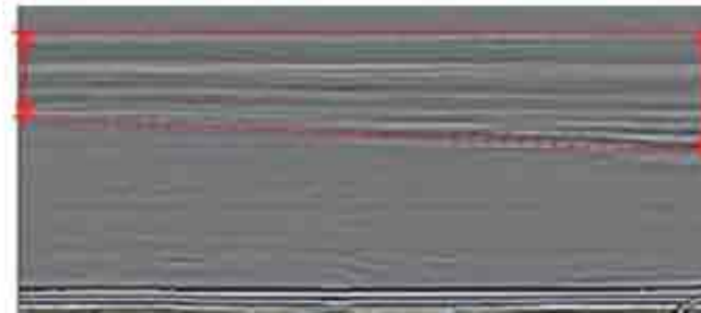
Axial scan image of the rod with crack showing extend of the crack along the length of the rod
