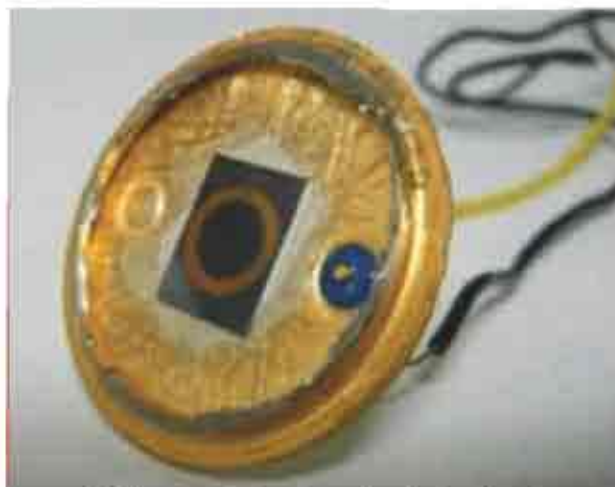
Indigenously developed radiation hard GaAs photodetector
