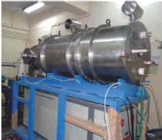
Linear Induction Accelerator: LIA-400
