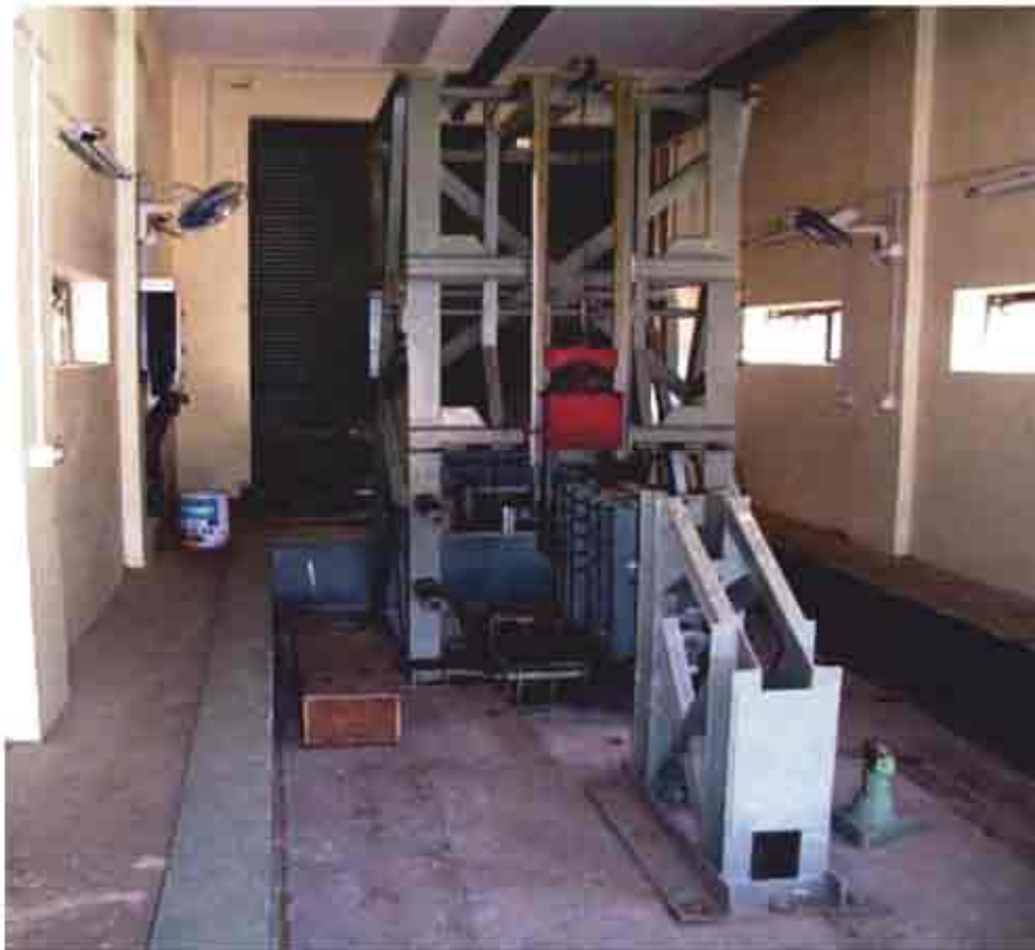
K-200 shock testing machine Installed at BARC
