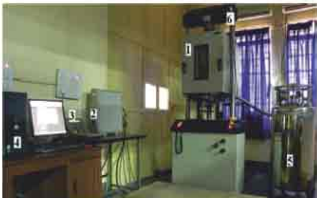
1 Cryo-chamber 2 Controller 3 Operator panel 4 Support computer 5 Liquid nitrogen cylinder 6 Temperature indicator.
