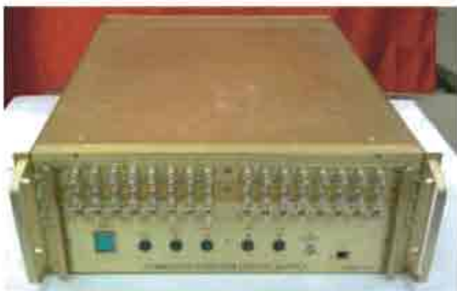
A 48-channel High Voltage crate
