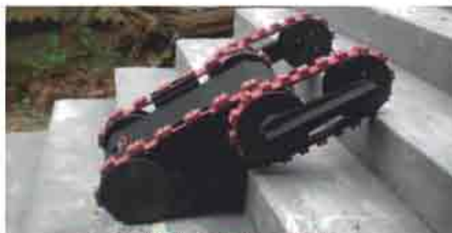
Tracked Robot Climbing Staircases
