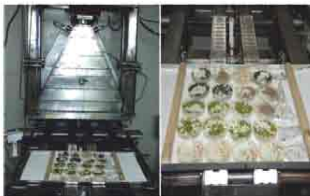
Electron beam irradiation of seeds for phyto-sanitary treatment
