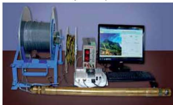
Borehole online survey system with video imaging and deviation measurement
