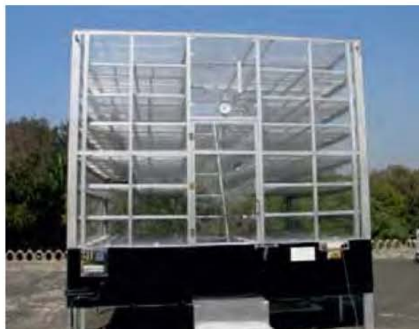
200 kg capacity Solar Dryer
