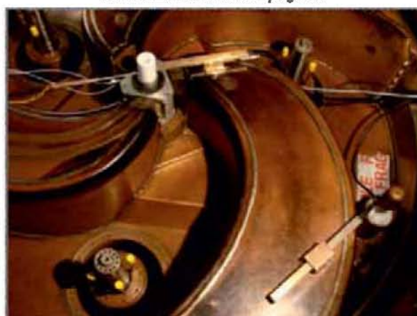
NMR probes kept at the center and on the hill for the calibration of the search coil
