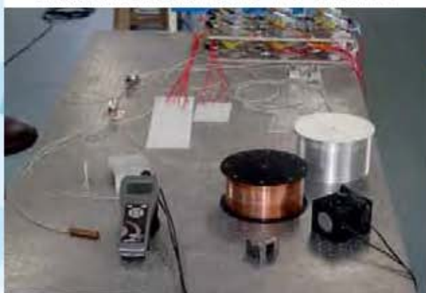
200 W all-fiber Yb-doped CW fiber laser
