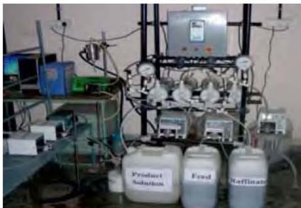
Bench-scale setup with four Hollow Fiber modules in series
