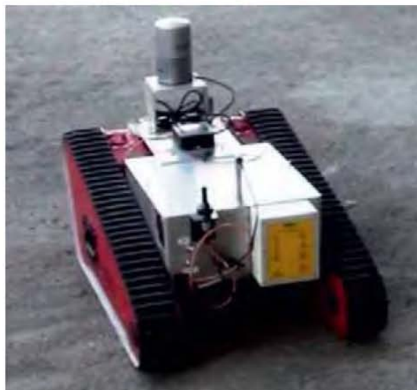
DORAbot- An Outdoor radiation survey robot
