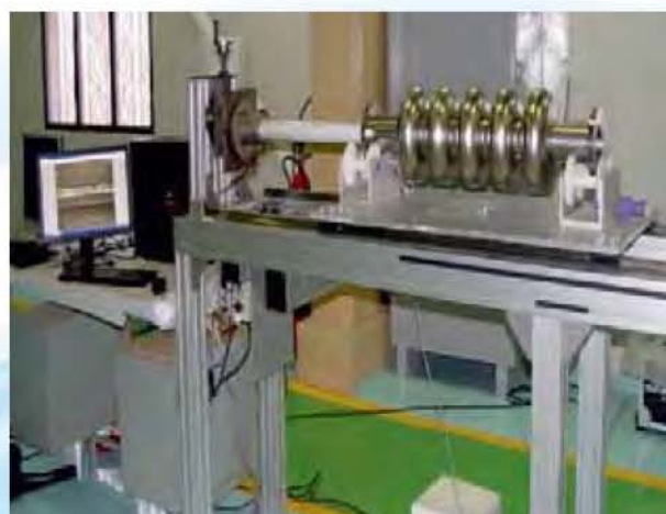
Niobium five-cell 1.3 GHz SCRF cavity being inspected on optical inspection bench
