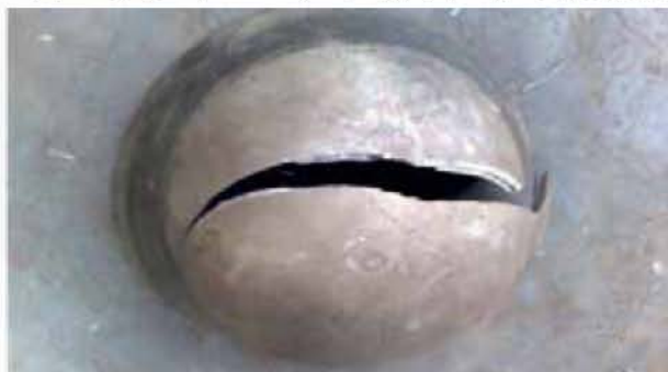
An Inconel 693 dome which failed during hot working
