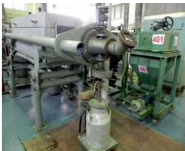
Rotary Expulsion Unit for UF 6 expulsion
