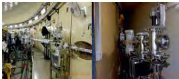
X-ray diagnostic beamline installed at Indus-2 (left) and filters and phosphor screen assembly installed in the hutch (right)
