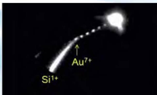
Quasi-mono-energetic gold ions of different charge states ( Au^{-1} to Au^{7+} ) observed in ultra-intense laser plasma interaction.
