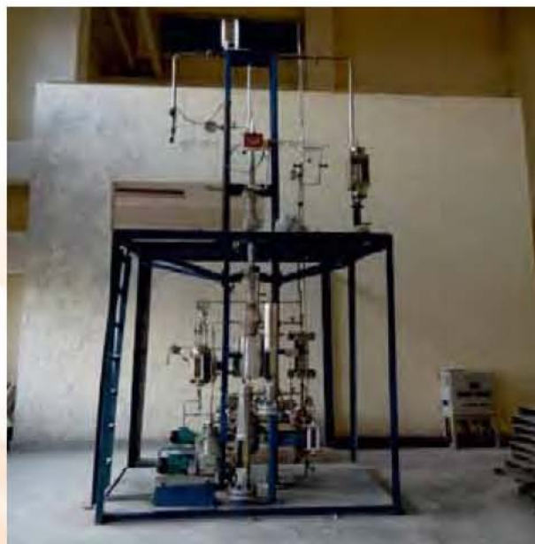
High pressure SS reactive distillation setup
