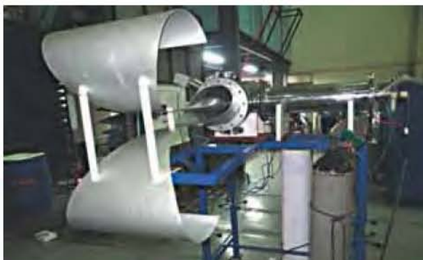
100kV UWB source with antenna
