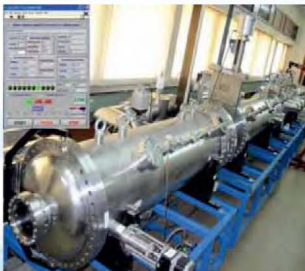
9-meter-long multi-cathode magnetron sputtering system
