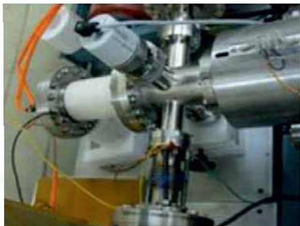
Triode type electron gun for the 10 MeV electron linac
