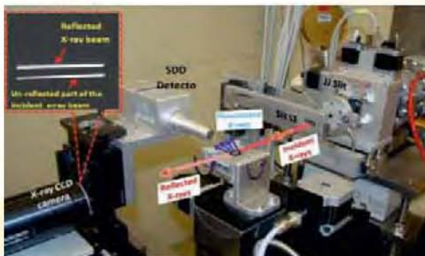
Total external reflection x-ray fluorescence facility at X-ray micro-focus beamline
