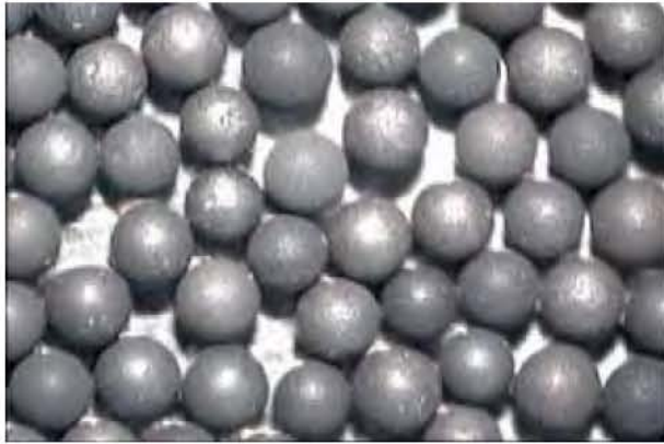
ThC 4 microspheres prepared by sol-gel process
