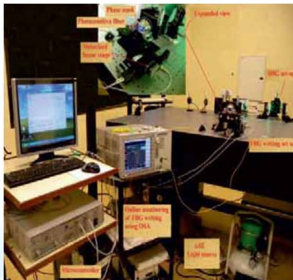
Computer controlled fiber bragg grating (FBG) inscription set-up
