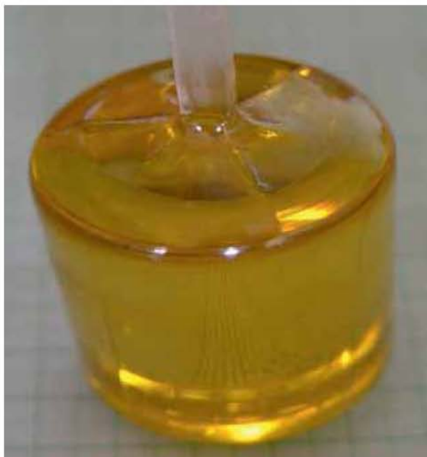
LiTaO 3 , single crystal; 42 mm dia. and 50 mm length
