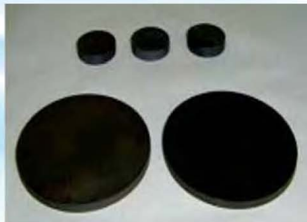
Indigenously developed ferrite resonator discs
