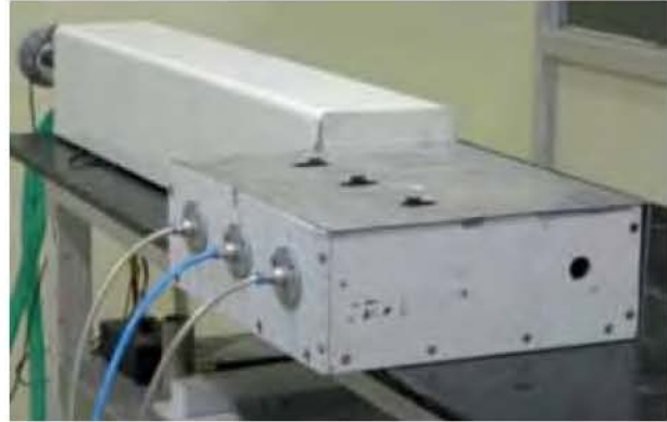
10 kW fiber coupled Nd:YAG laser
