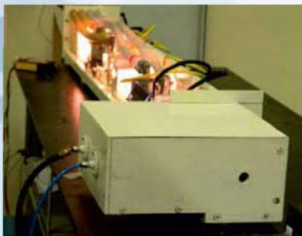
Prototype model of 20 kW peak power industrial Nd: YAG laser
