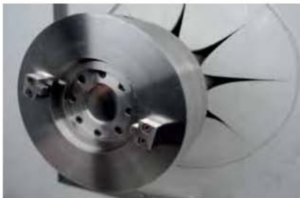
Titanium window for proton beam irradiation of biological samples
