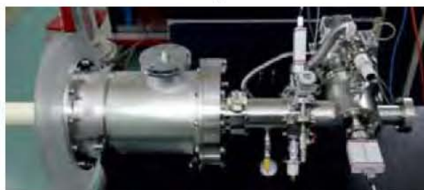
Compact capillary discharge soft x-ray laser
