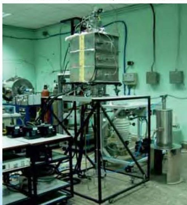
RF Plasma CVD Facility for Deposition of Boron Carbide Coatings on inner walls of S.S. tube
