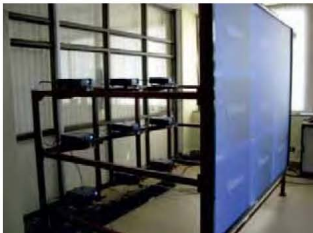
Projection based Seamless Tiled Display
