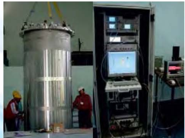
The VTS facility for characterization of SCRF cavities and RF instrumentation
