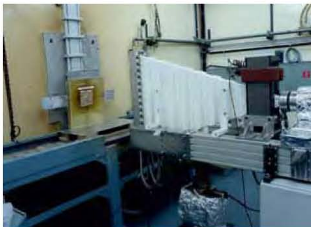
Irradiation of seeds by 7.5 MeV beam from electron linac
