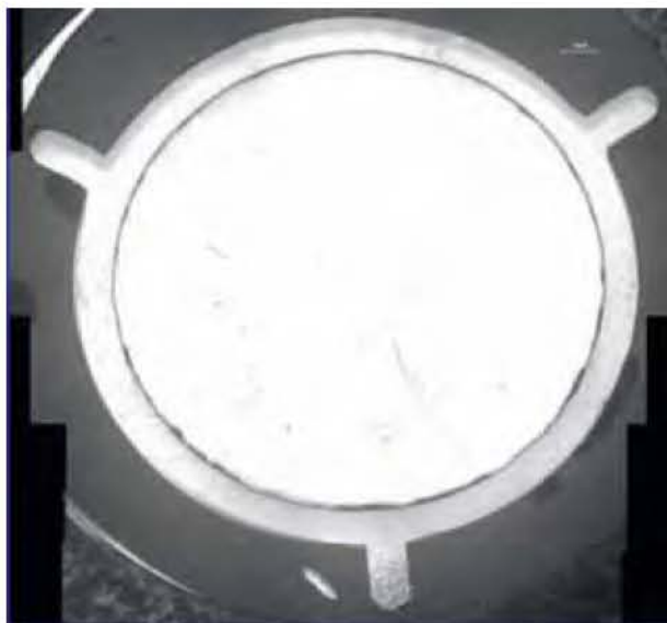
Dhruva fuel pin cross section U-rod and Al clad
