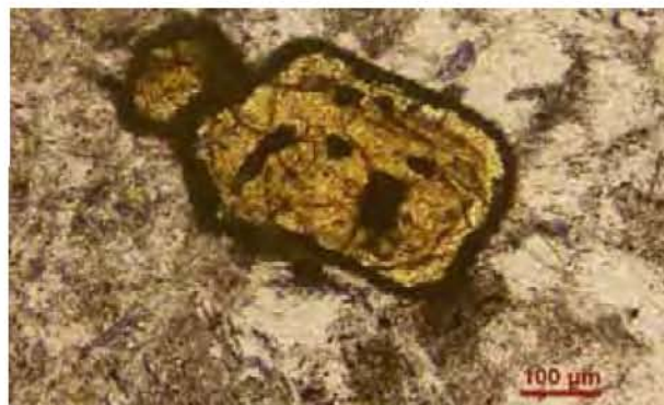
Photomicrograph of Metamict REE mineral in alkali granite
