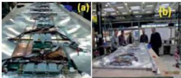
(a) & (b): Assembly of RPC Super-module at CERN
