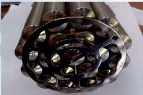
A carrier tube assembly of PHWR fuel bundle
