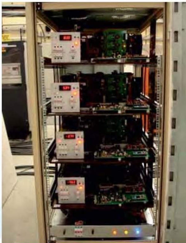
Power supplies for fast corrector magnets for Indus-2
