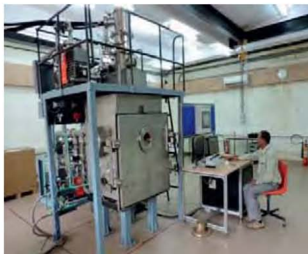
80 kV, 12 kW EB welding machine
