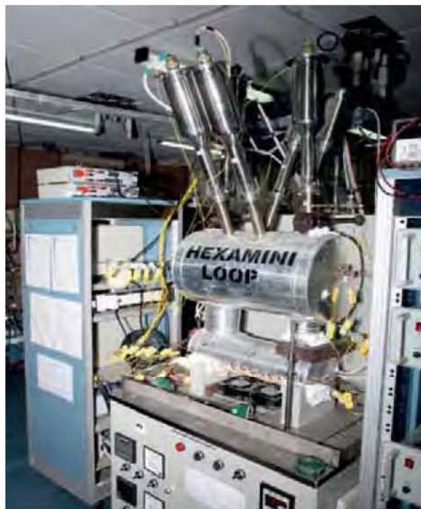
ECHMs undergoing long-term performance test in bench top sodium loops
