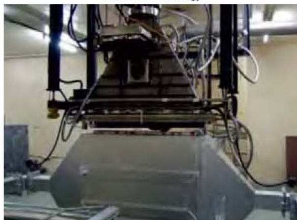
40 mm dia electron beam exits the high vacuum horn through titanium foil
