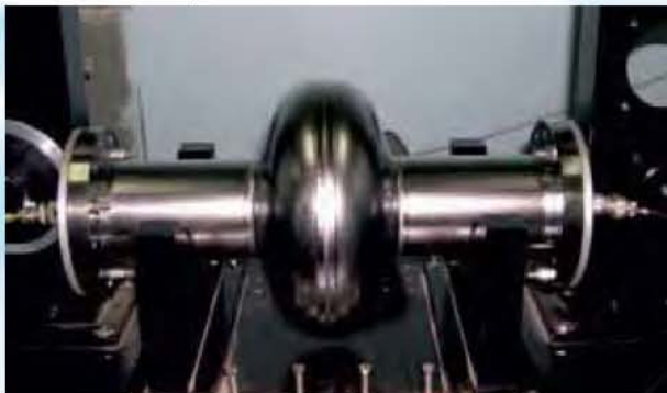
World's first laser-welded single-cell 1.3 GHz niobium SCRF cavity
