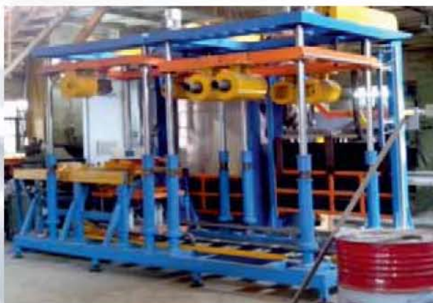
The 3-axis mechanical manipulator employed for the waste assay
