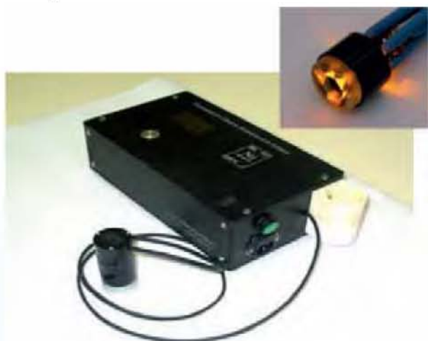
Fluorescence lifetime measurement probe for Nd doped laser materials
