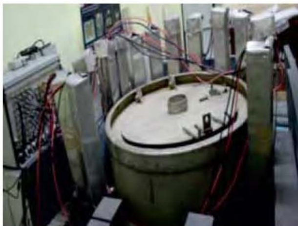
Experimental assembly showing bank of He-3 detectors surrounding the simulated hull vessel
