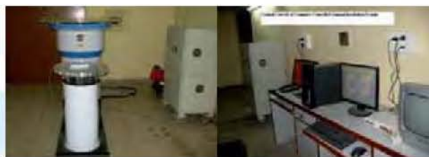
Irradiator and control console parts of gamma calibration system
