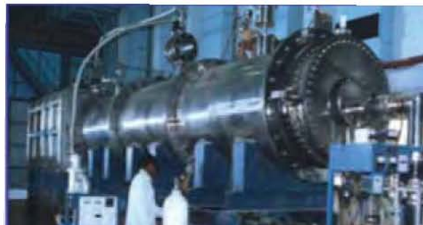
1MV, 30kA, 80ns Pulsed e- Accelerator
