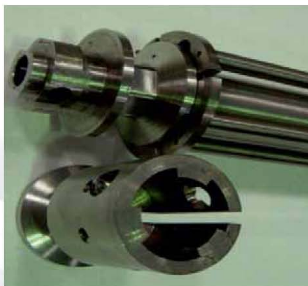
A dismountable type cobalt absorber assembly for 700 MWe PHWRs
