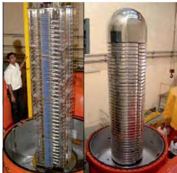
3m tall accelerating column to generate electron beam of 3MeV energy
