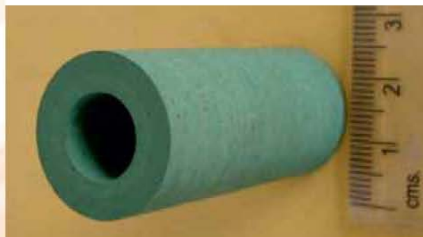
NiO-YSZ porous ceramic sleeves for use as liquid film breaking device
