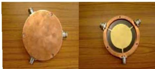
Stripline ferrite 3-port circulator
