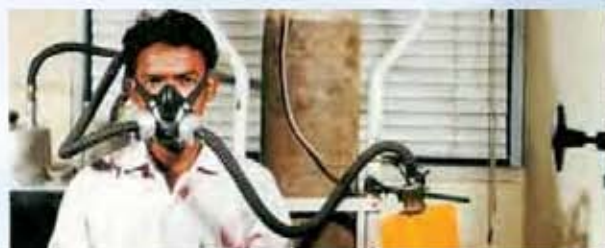
Measurement of Radon/Thoron in Exhaled Breath
