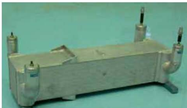
Plate-fin heat exchanger for indigenous helium liquefier
