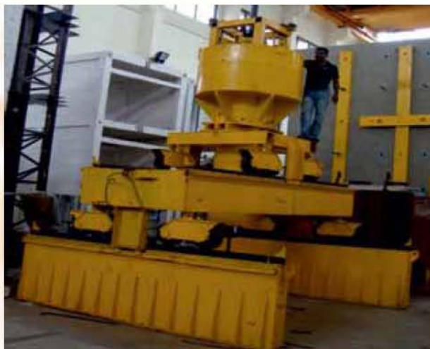
1:4 Scale Model of AHWR Fuelling Machine for Seismic Testing
