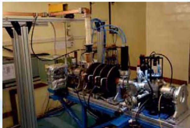
Developed prototype 5 MeV TW electron linac
