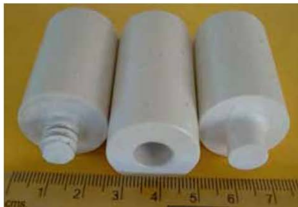
3YSZ Components for use as end plugs in Heat Pipes (CHTR programme)
