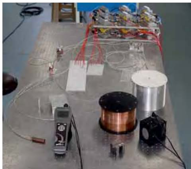
200 W all-fiber Yb-doped CW fiber laser
