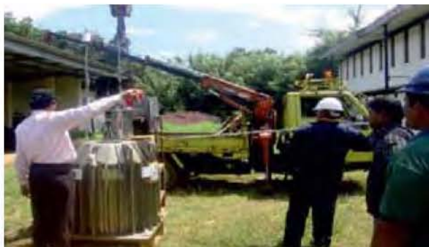
BLC 125 flask for exporting Cobalt-60 to Sri Lanka
