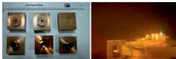
EB welding of Test coupons for parameter optimization and preparation WPS for the main crucible welding
