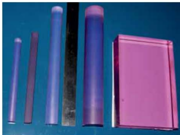
Indigenously developed Nd phosphates glass rods and slab.
