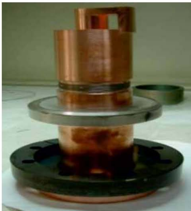
A coaxial coupler developed & used upto 60 kW during beam acceleration from RFQ
