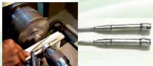
Reduction of core diameter of wire in lathe and laser welded ESPLDs
