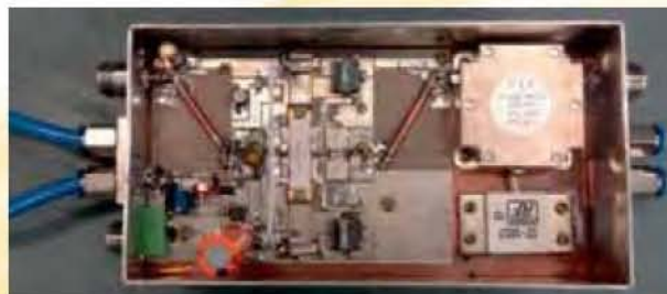
500 W solid state amplifier module at 650 MHz
