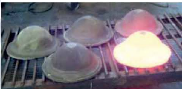
Domes of Inconel 693 successfully forged using optimised process
