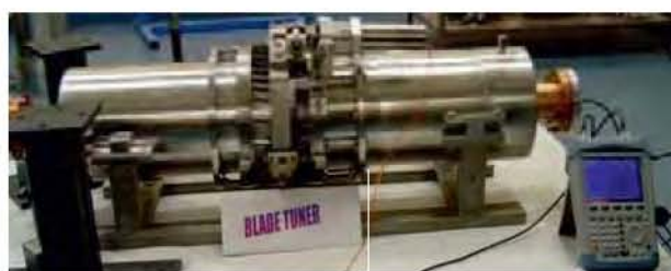
Blade tuner integrated with 1.3 GHz prototype dressed cavity
