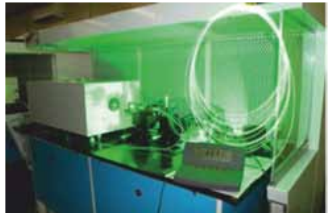
DPSS green laser under operation with fiber coupling
