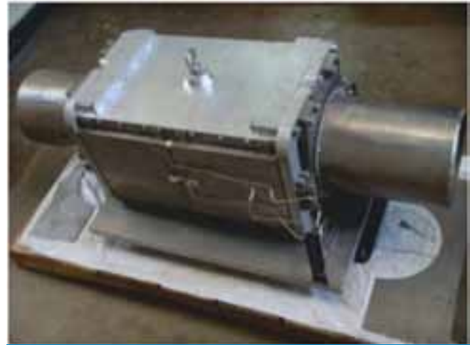
Indigenously manufactured permanent magnet flow meter
