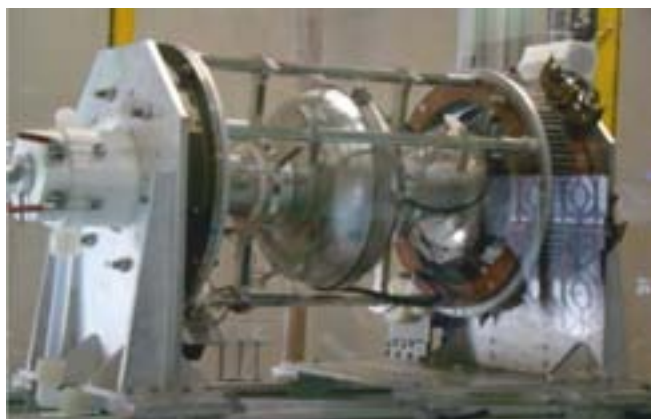
Electro-polishing of single-cell 650 MHz SCRF cavity
