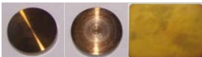
Boron Carbide films on stainless steel discs & Al for neutron detection in DHRUVA
