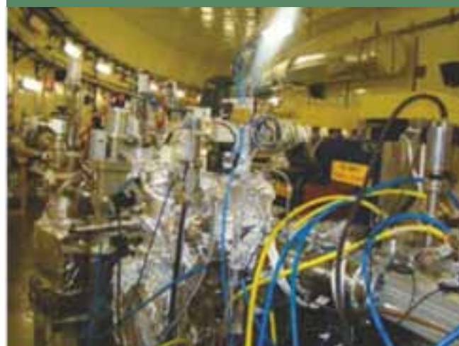
Front end part installed in BL-10 ARPES beamline
