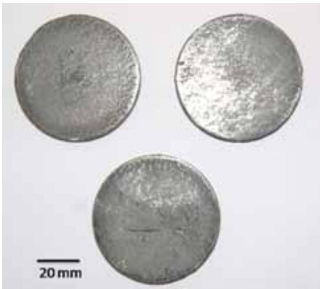
60 mm diameter and 5 mm thick Mo-Ti-Si alloy plates produced by vacuum hot pressing
