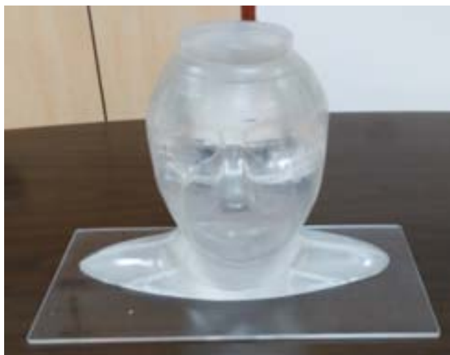
A specialized anthropomorphic HN dosimetry audit phantom
