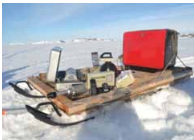
Radiation survey over the sea ice of McLeod Island with system mounted on a movable platform
