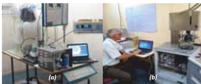
Facility for testing of (a) Respirators (b) Particulate Filter Media
