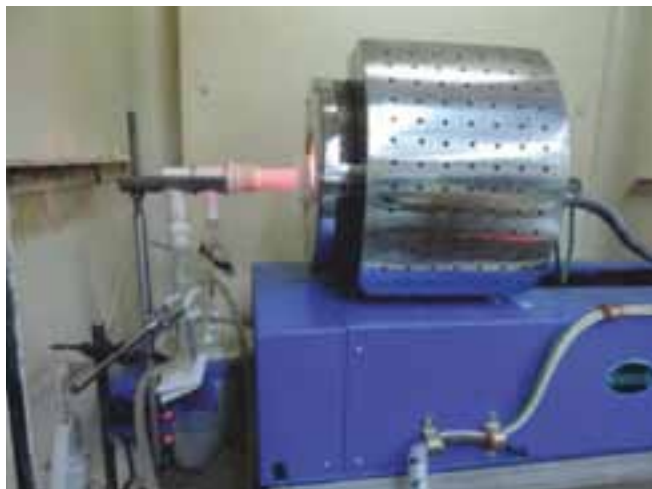
High Temperature Pyrohydrolysis System
