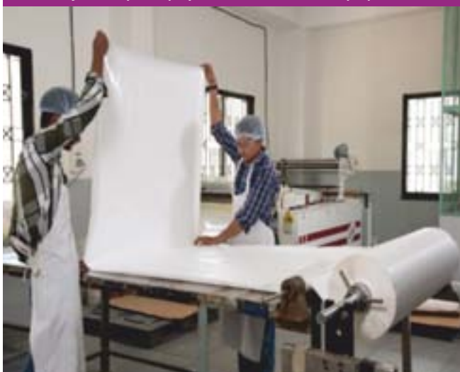
Rolling of commercial size 8040 spiral membrane element
