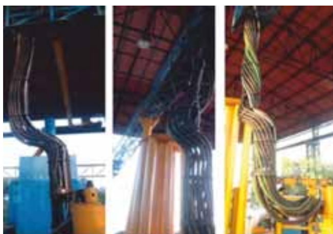
Profile for trailing cables under different plug
