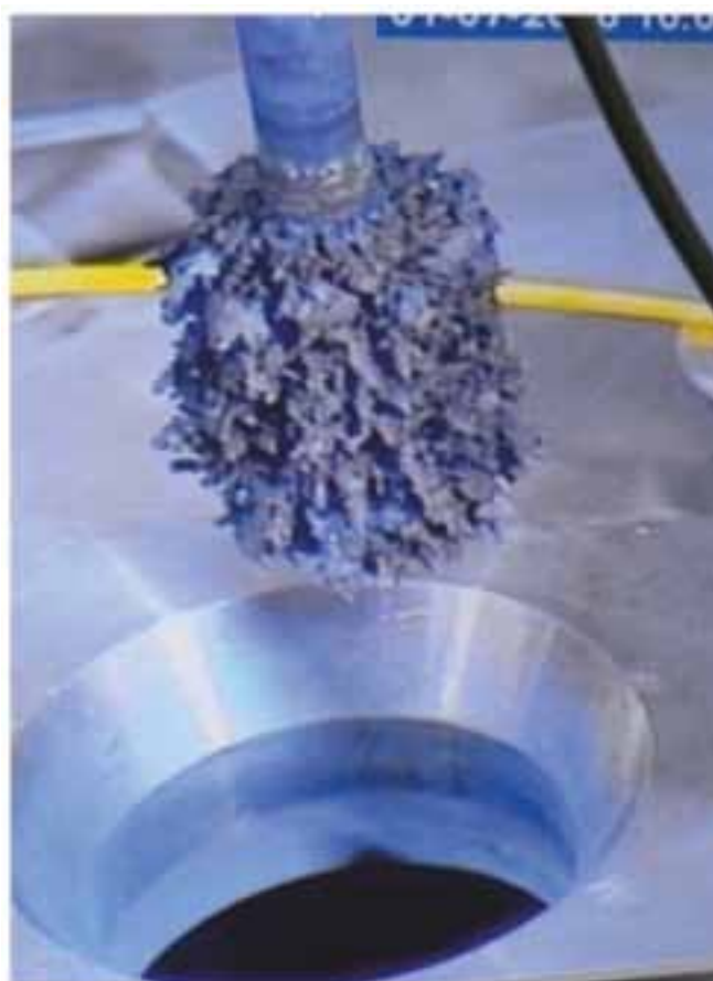
Uranium deposit from electro refining of U-Zr alloy in hot cell
