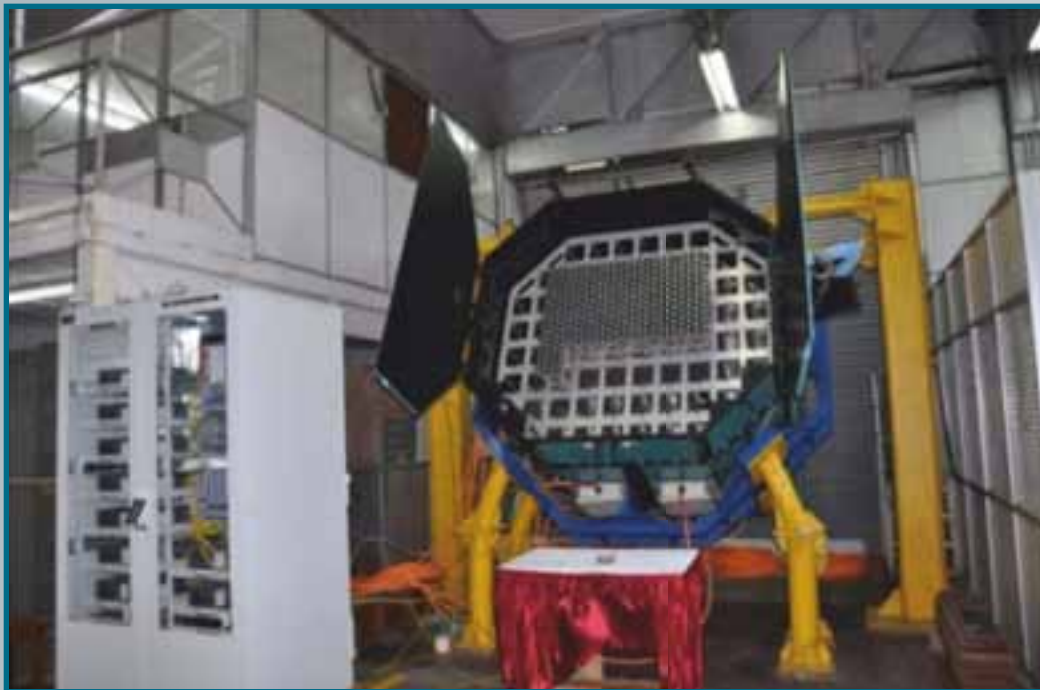
MACE camera loaded with Camera Integrated Modules CIMs
