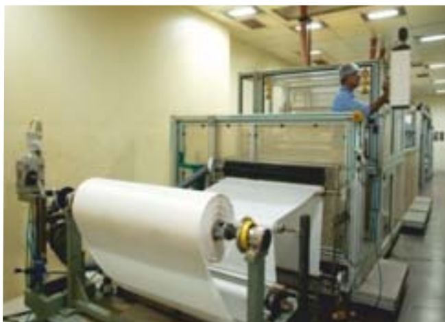
Thin film composite polyamide RO membrane in preparation
