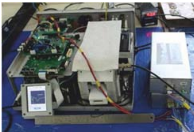
Oxygen detection on detector's screen with RRCAT HV pulse and HV DC supplies
