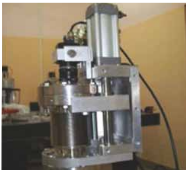
Beam Profile Monitor installed in Indus-2 ring
