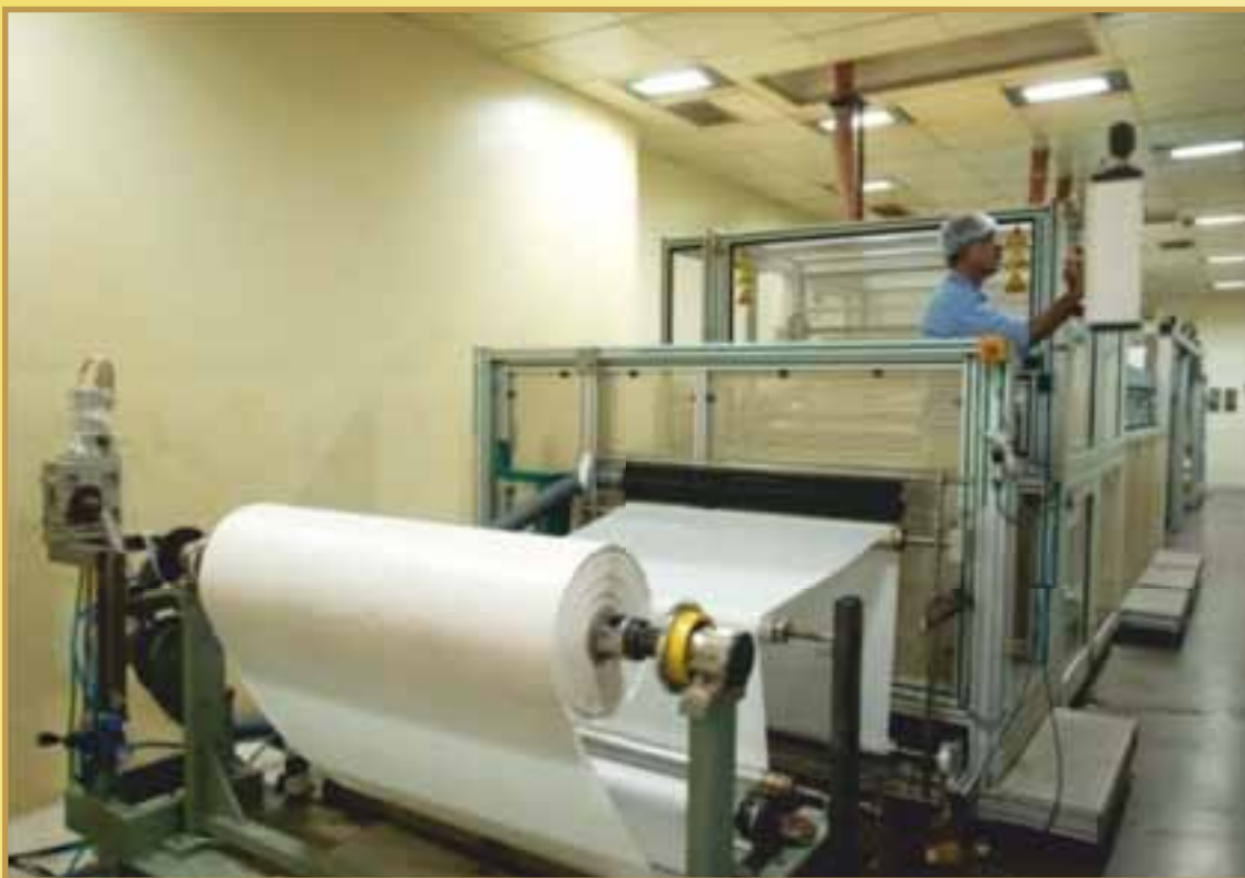
Thin film composite polyamide RO membrane in preparation
