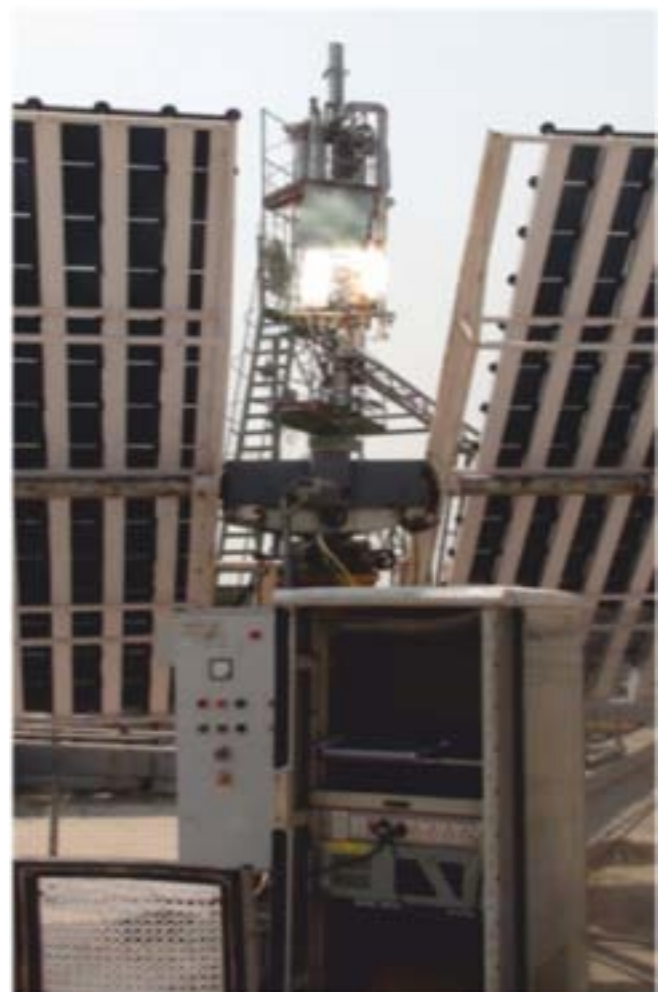
Heliostat control system for Sun tracking
