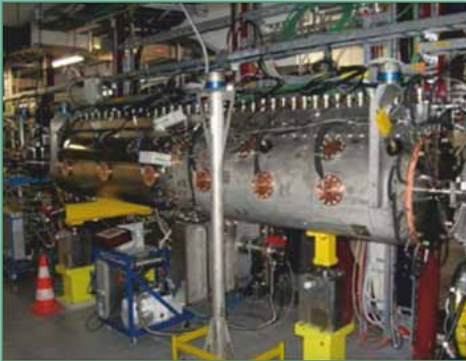
One of the WR 2300 copper coated Stainless steel power couplers installed with the CCDTL accelerating structure of linac-4 tunnel at CERN
