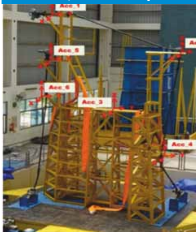
Seismic qualification experiments for long extended stem valves
