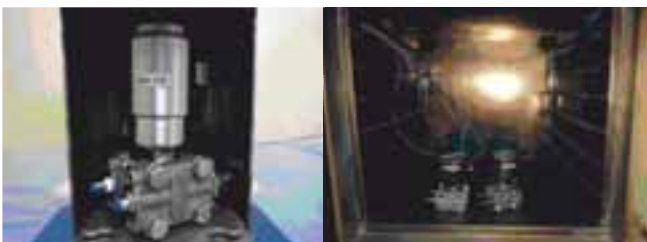
Radiation Test on Transmitter and Accelerated Thermal Ageing on Transmitter in progress
