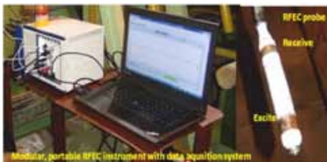
RFEC instrument and probe developed for baseline data generation of SG tubes
