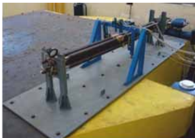
Shake table experiments on air heat exchanger tubes
