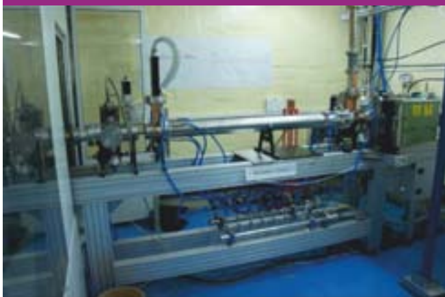
Second linac tested at beam power of 1 kW
