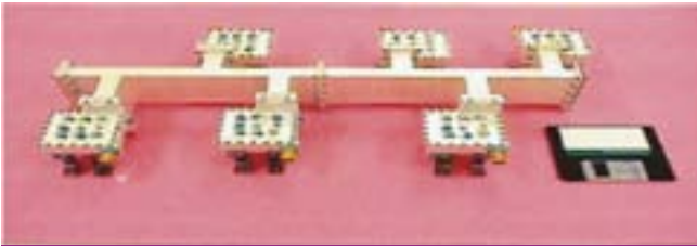
Multiplexer Module in Indian Communication Satellite
