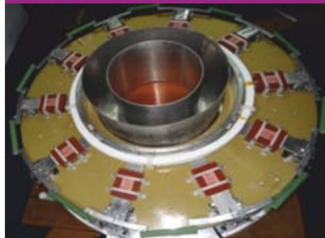
Layout of LTD cavity with ten bricks (top plate and load removed)
