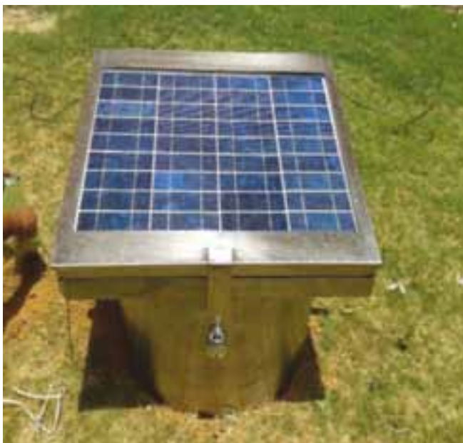
Solar powered geo-gas ( ^{222}\text{Rn} & ^{220}\text{Rn} ) monitoring station
