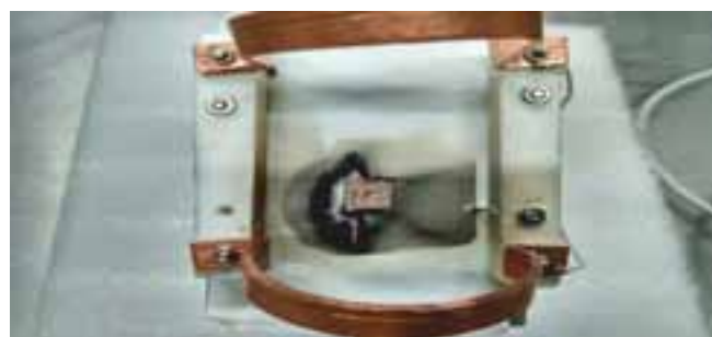
The sample holder and the beam spot taken before doing the actual experiment with the ECR Ion Source of IOP
