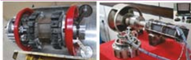
PIG with speed control mechanism
