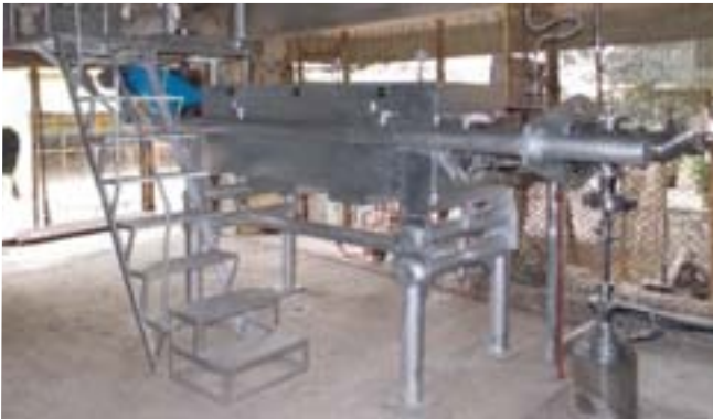
Rotary reactor for the synthesis of solid breeder material in continuous operation
