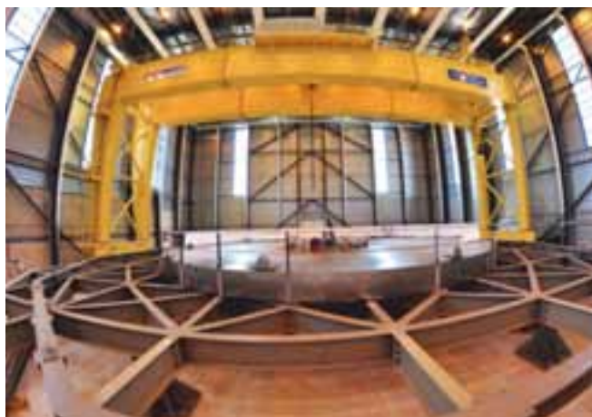
Base section of Cryostat, manufactured by L&T
