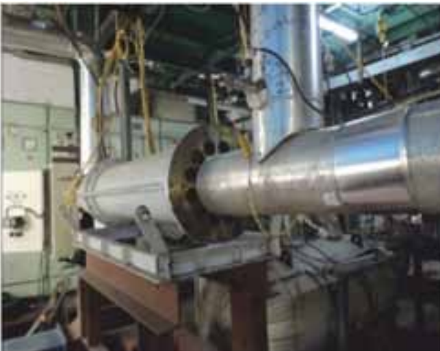
1.5 m 3 /h Annular Linear Induction Pump during testing
