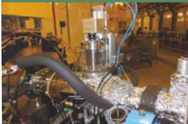
Photographs of BPM and bellow assembly during lab test
