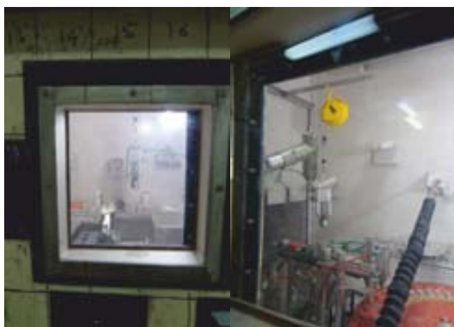
Pneumatic vial capping and de-capping tools, in 131I capsule plant
