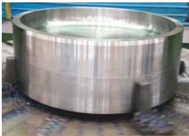
Indigenous 700 MWe SG Tube Sheet Under Machining
