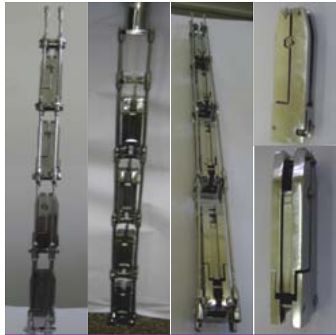
Prototype sample holder for the for Corrosion Loop Experiments flow (CLOE) for Jules Horowitz Reactor (JHR)
