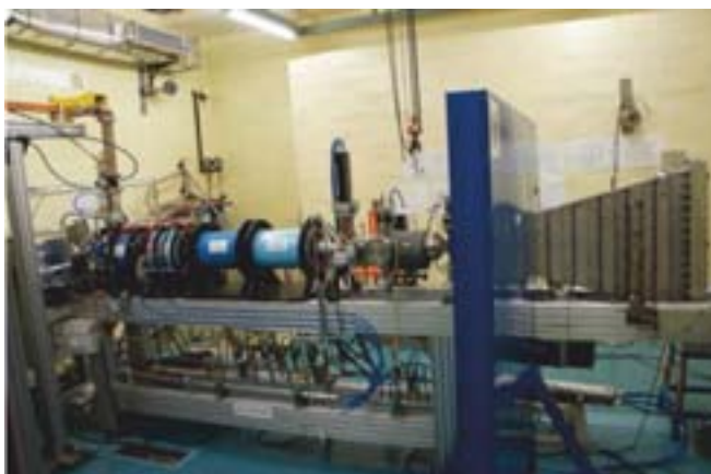
First linac tested at beam power of 5 kW
