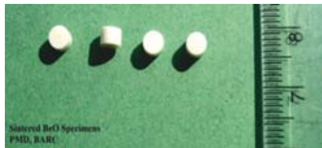
Sintered BeO specimens for multiplexer-support application
