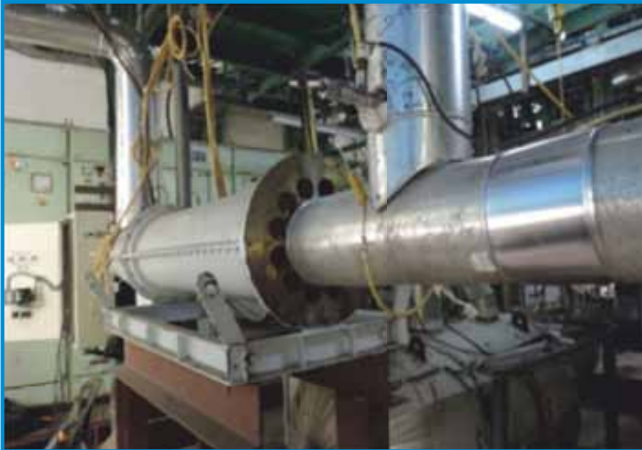
1.5 m 3 /h Annular Linear Induction Pump during testing
