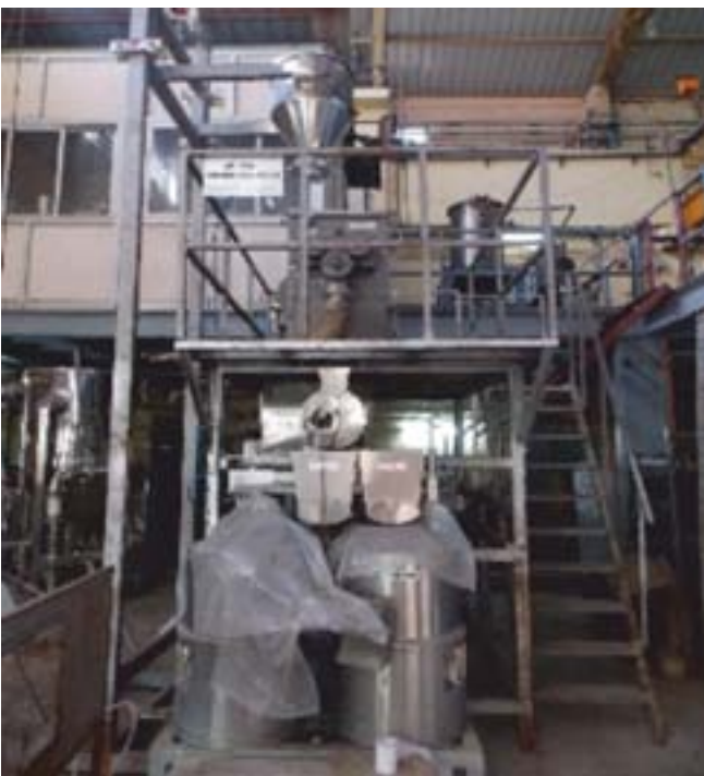
Automated granulation system for the fabrication of pebbles of solid breeder material
