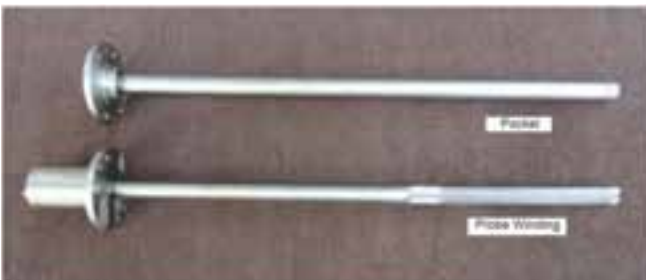
Mutual inductance type level probe
