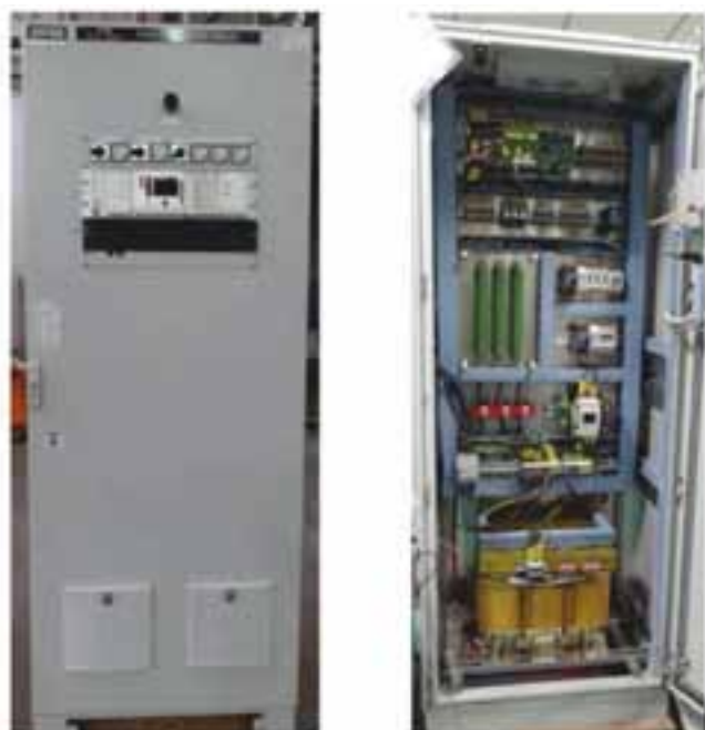
Power converter for electromagnet developed for FAIR
