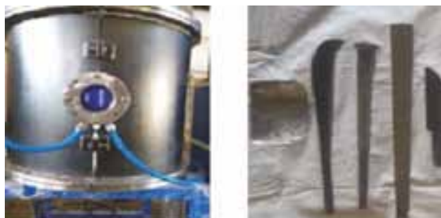
(a) radical plasma nitriding system developed in FCIPT and (b) radical plasma nitrided agricultural tools
