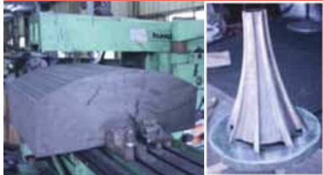
Machining of hexagonal graphite fuel tube and downcomer tubes
