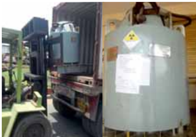
Installation of 125 kCi Co-60 sources for Sri Lanka Atomic Energy Board
