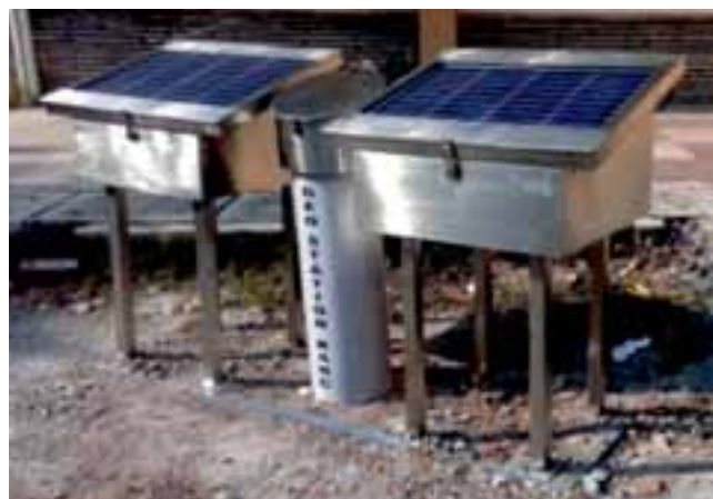
In-house developed Radon Geo-Station
