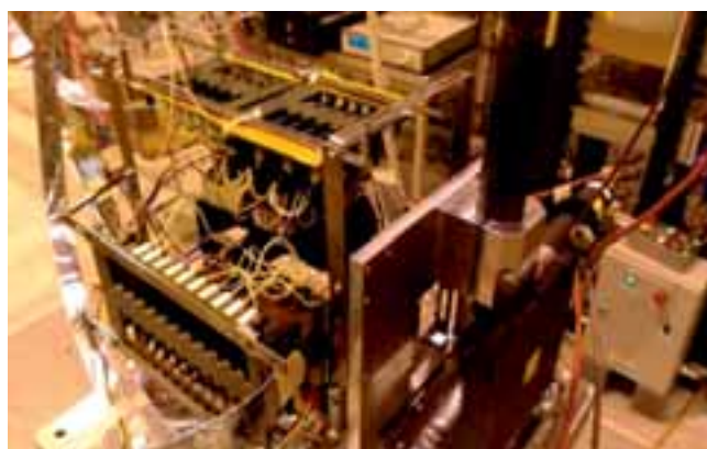
A 20Xr thick sampling type silicon-tungsten calorimeter prototype
