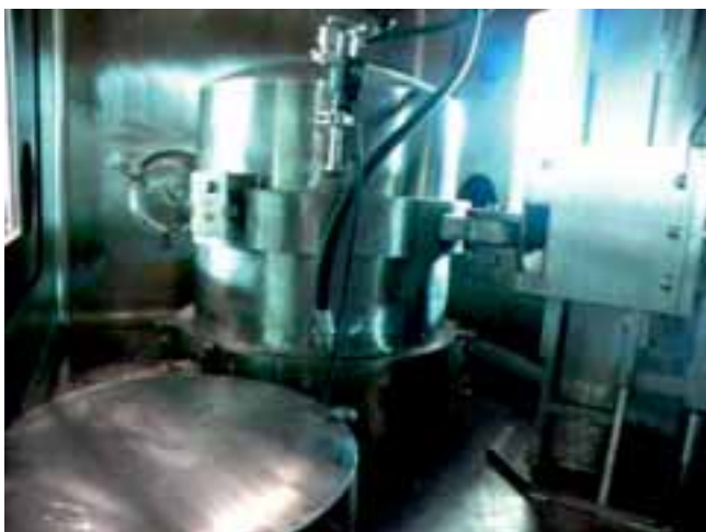
High temperature MOX sintering furnace inside glove box
