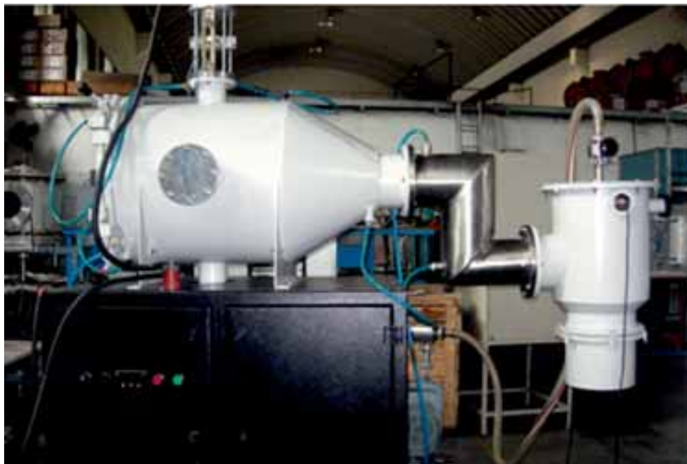
Nano-titania production system installed at Institute for Plasma Research, Gandhinagar
