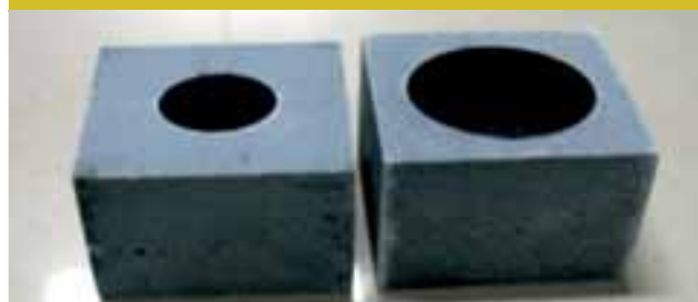
Beryllia blocks fabricated by vacuum hot pressing
