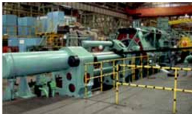
The high pressure return rams in which specialized major welding repairs carried out on the underside
