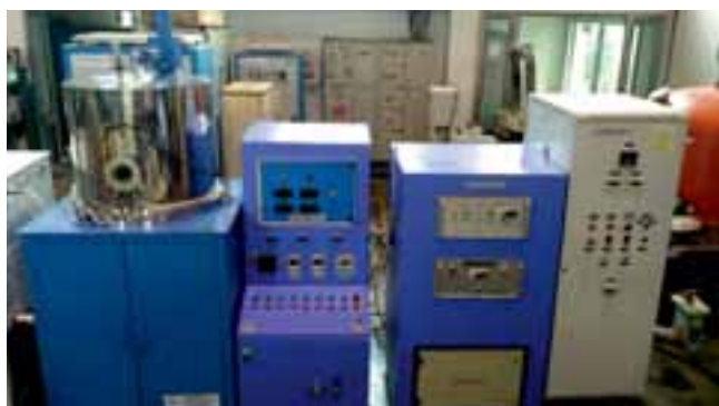
Indigenously developed plasma nitriding system for ISRO Inertial Systems Unit
