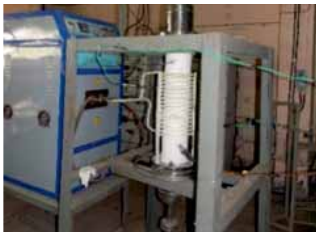
Experimental setup to study pebble bed heat transfer with internal heat source
