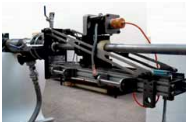
Compact BARCIS Drive System for Coolant Channel Inspection in PHWRs
