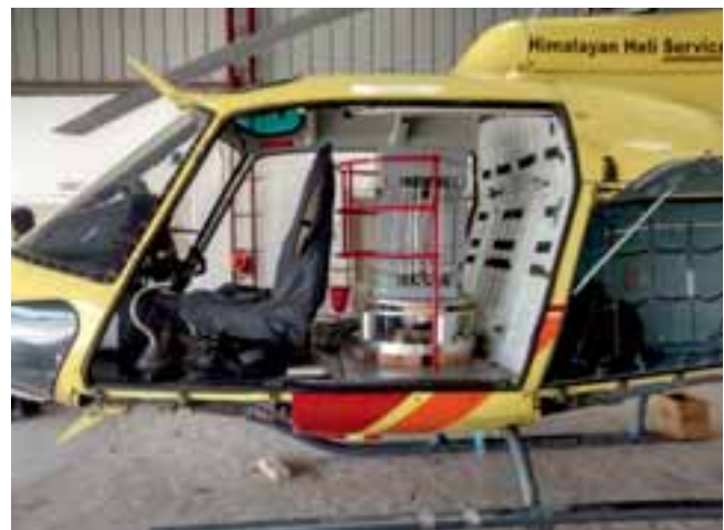
Gravimeter (GT-1A) installed on helicopter platform before survey
