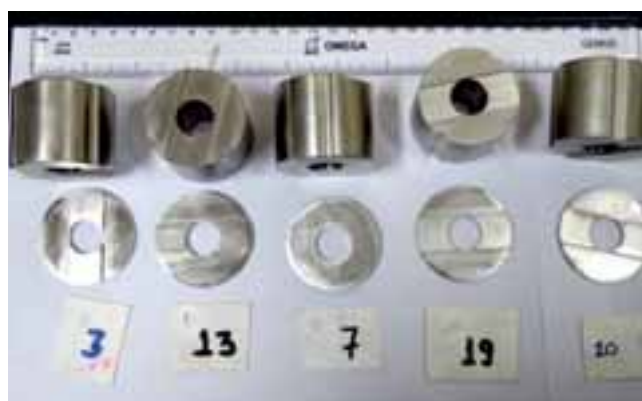
Corrosion/erosion resistant nano-Ni coated Alnico-3 magnets
