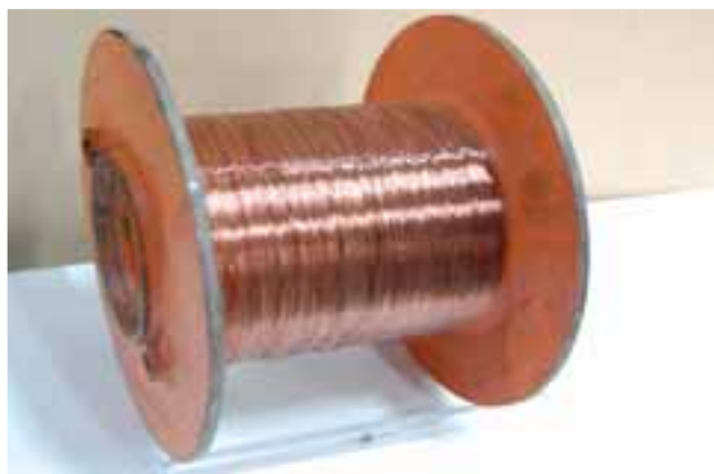
200m long Nb 3 Sn Superconducting wire on a Bobbin
