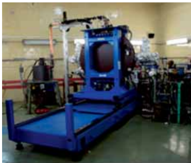
A view of the indigenously developed RF cavity installed with the Indus-2 ring straight chamber
