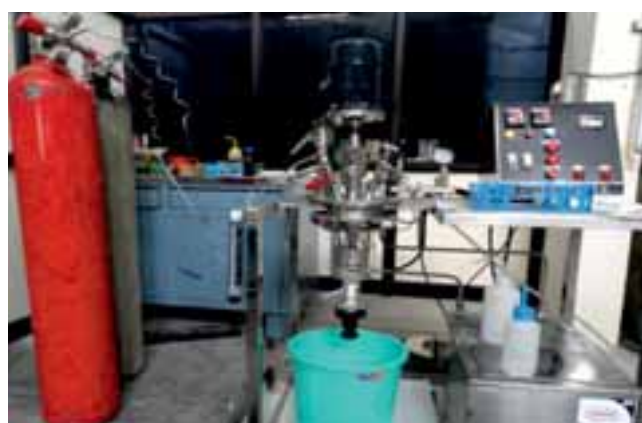
Glass autoclave setup for catalytic hydrogenation of uranyl nitrate
