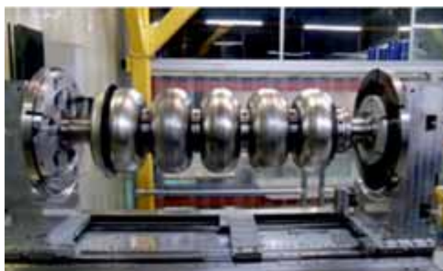
First 650 MHz ( \beta=0.92 ) five-cell SCRF cavity developed at RRCAT
