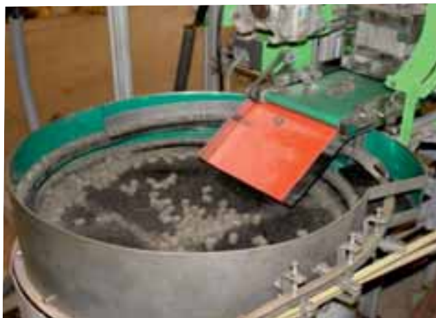
Development of Automatic \text{UO}_2 Pellet Unloading System for Moly Charge Carrier
