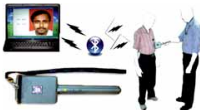
The RFID based Hand Held Reader for Attendance Recording
