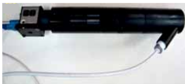
Hand held orthogonal polarization spectral imaging setup for in-vivo imaging of micro-vasculature
