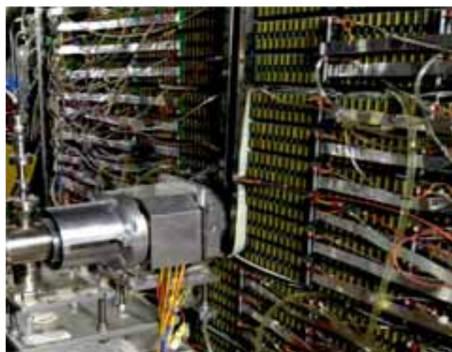
Photon multiplicity detector after repair in 2017
