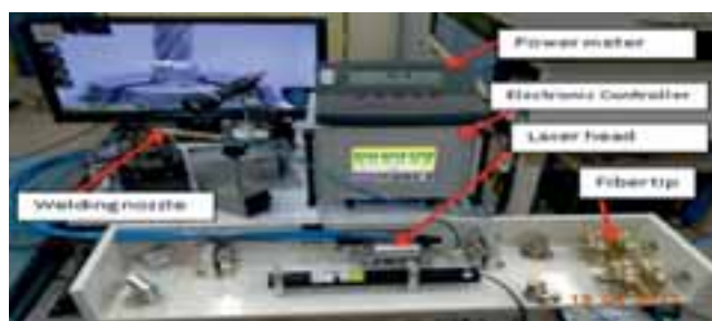
A view of in-house developed laser welding system for brachytherapy assemblies
