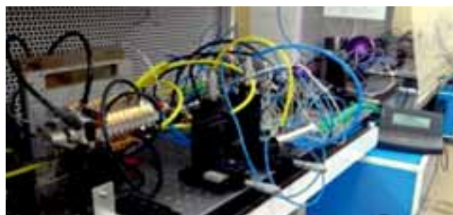
Diode pumped fiber coupled high power CW Nd:YAG laser
