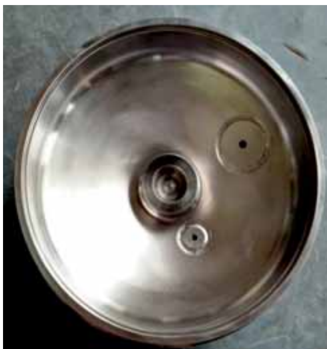
Electron Beam Welding of Nozzle less Booster (NLB) Head for DRDL, Hyderabad
