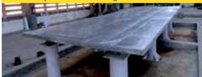
Rolled and final machined plate ready for dispatch (First such End Shield Plate developed in the country)
