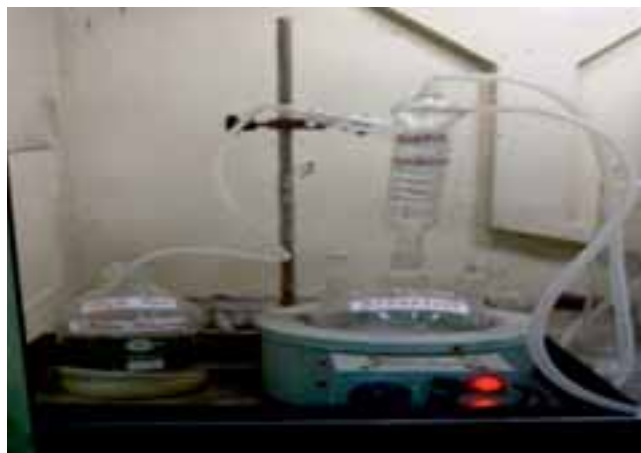
Dissolution Set up housed in Fume hood
