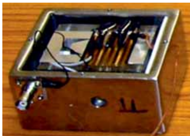
A miniature parallel-plate type Free Air Ionization Chamber
