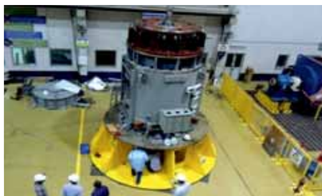
Assembled 6.0 MW PCP Motor
