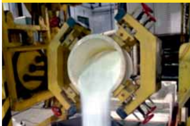
60L Refractory Pot and Trial tilt cast operation
