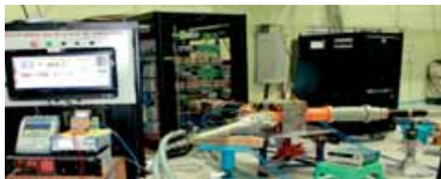
High power RF testing of 505.8 MHz circulator
