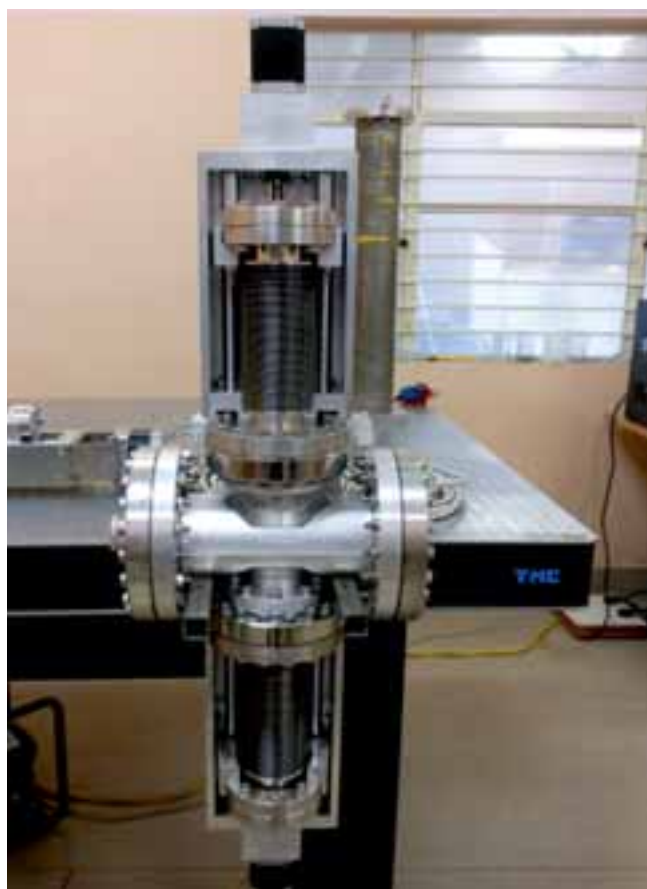
In-house developed upgraded vertical scraper for Indus-2
