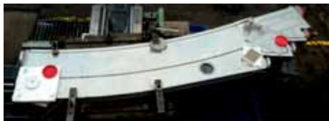
Indus-2 dipole magnet vacuum chamber after modifications
