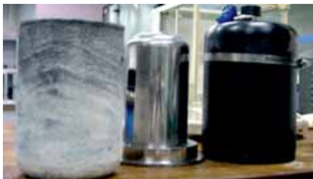
Green MgO crucible shape formed by CIP
