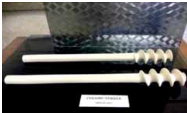
Stirrer designed and fabricated at CGCRI
