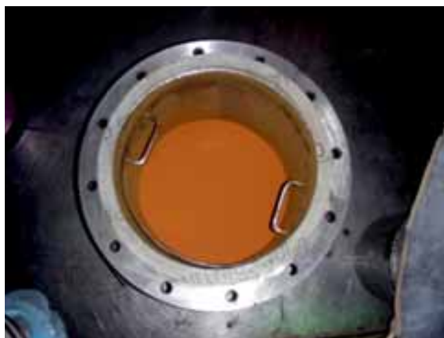
Product UO 3 discharged from the reactor to the product collection vessel
