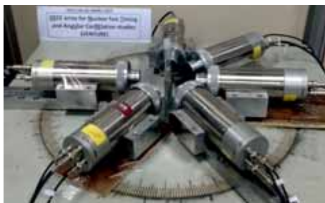
VENTURE array used for the lifetime measurements in ^{117}\text{Sn} and ^{160}\text{Dy}
