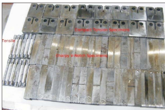
Types of mechanical testing specimens from Thermal Ageing Surveillance Specimen from Kudankulam VVER reactor
