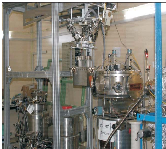
Hexapod based mirror alignment system for Indus-2 beamline
