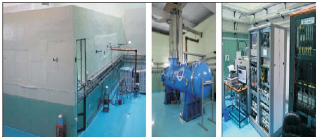
HTS Vault with 40kW SSA. HTS Cryostat and LLRF & Control System
