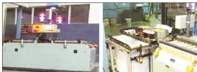
Successful shop floor demonstration of Automatic Guided Vehicle (AGV) for movement of UO 2 pellets
