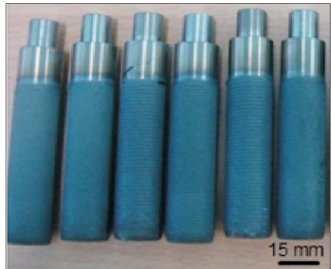
Laser based direct energy deposited tungsten carbide (WC) as deposited
