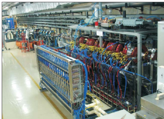
IR-FEL setup installed inside a 60 m long radiation shielded area
