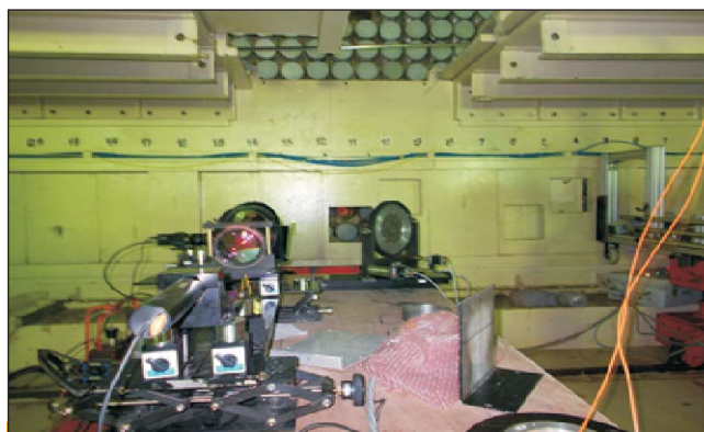
Laser based sag measurement setup in the vault of KAPS-1
