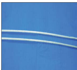
As Extruded tubes of Pure Nickel
