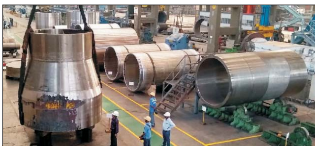
Steam Generator Forgings under Manufacture
