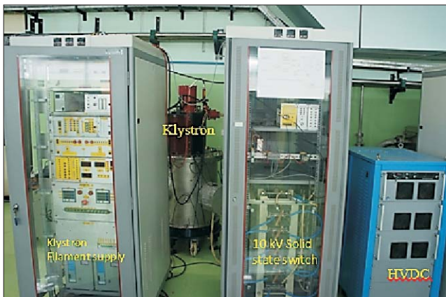
Test set up of high voltage solid state switch with the klystron
