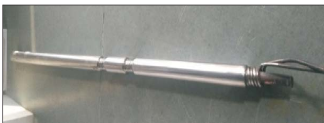
Pressuriser Heater with Sheath Partly Removed
