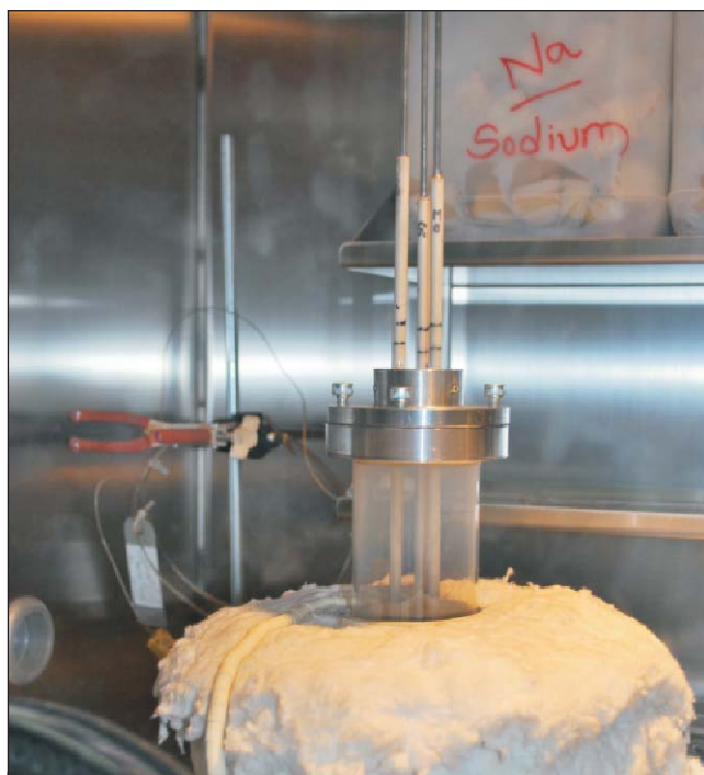
Electrochemical salt purification demonstration facility located inside an inert gas glovebox
