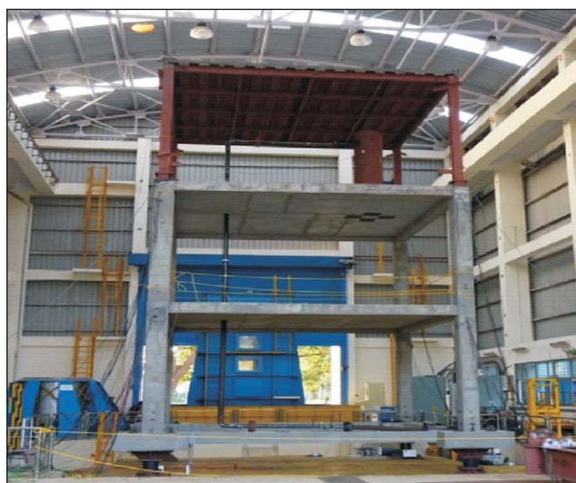
Multi-story concrete building mounted on shake table with base isolators
