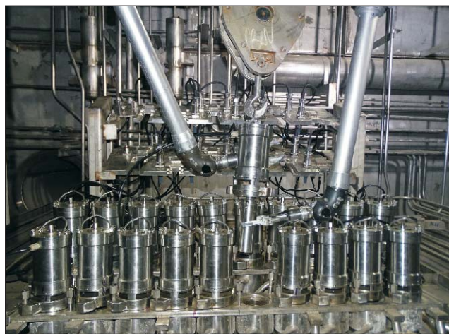
Centrifugal Extractors with remote handling
