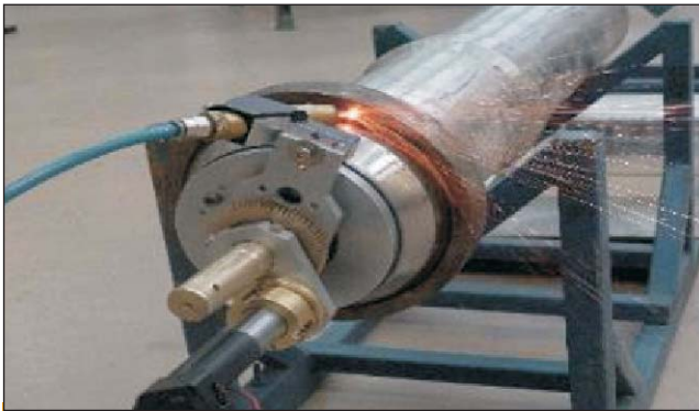
Bellow lip cutting tool mounted on end fitting for mock up
