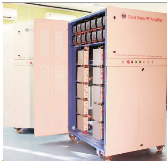
325 MHz pulsed solid-state RF amplifier for RFQ
