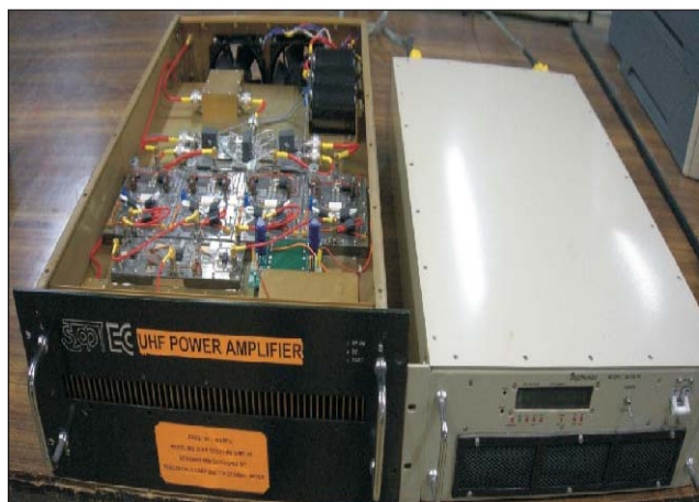
Transmit Receiver (TR) Module in 50MHz and 400 MHz
