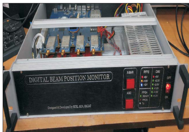
Single pass digital beam position monitor unit
