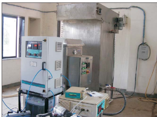
Advanced Effluent Water Treatment Plant (AEWTP) pilot plant
