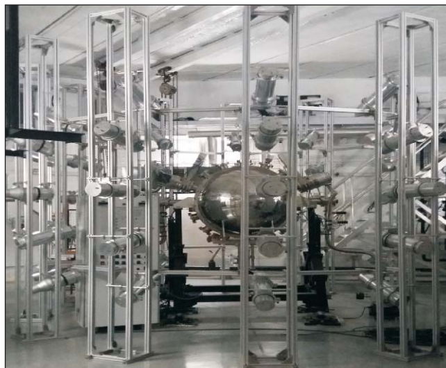
Indigenously developed neutron detector array at VECC
