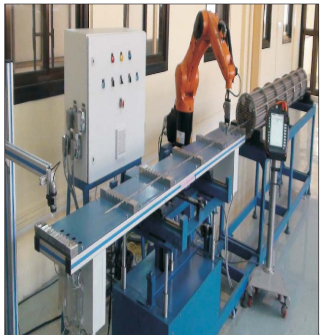
Autonomous robotic solution for loading of PFBR fuel pins
