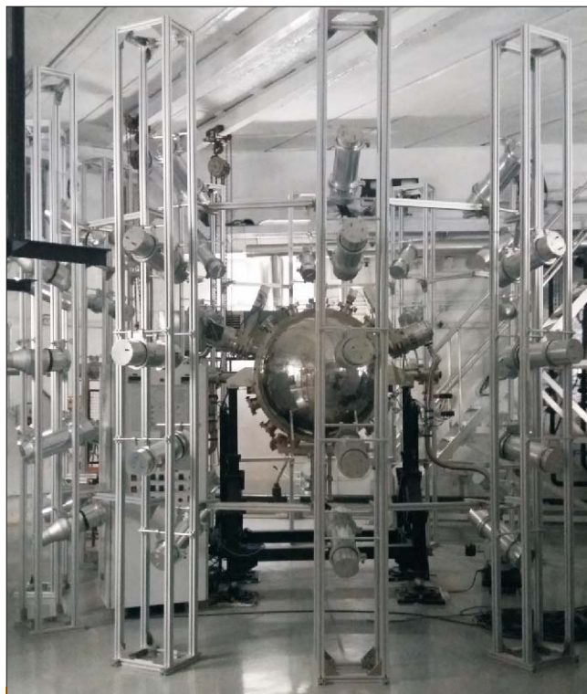
Indigenously developed neutron detector array at VECC
