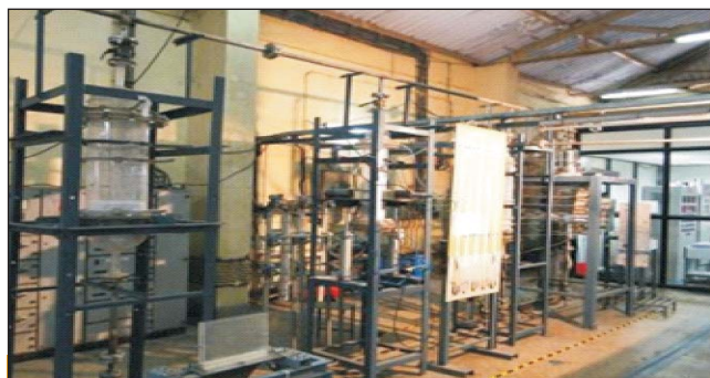
Experimental set-up for adsorption and recovery of Trichloroethylene
