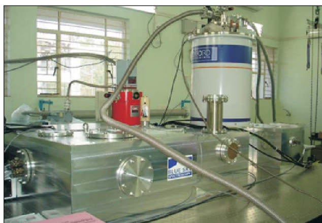
IR-THz frequency domain spectrometer set up for the utilization of FEL radiation
