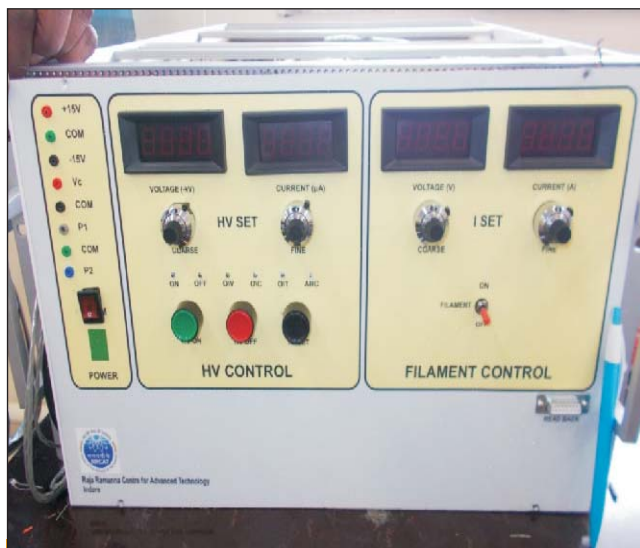
A view of in-house developed HV power supply unit for SEM
