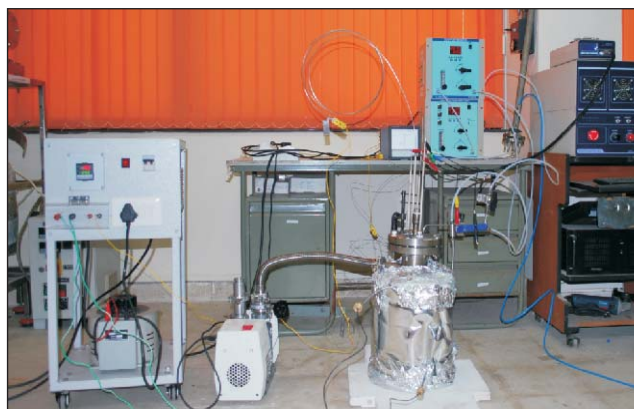
Facility for demonstration of online measurement of impurities in molten fluoride salts
