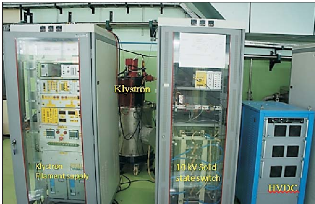
Test set up of high voltage solid state switch with the klystron
