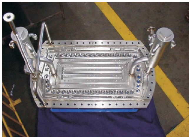
High Heat Flux testing of Back Plate of NBI PINI ion source
