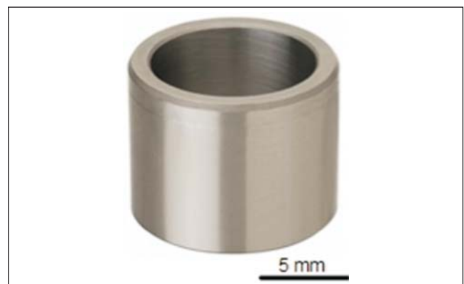
Laser based direct energy deposited tungsten carbide (WC) after machining
