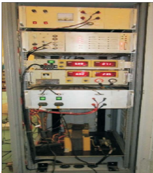
In-house developed vertical pinger magnet power supply
