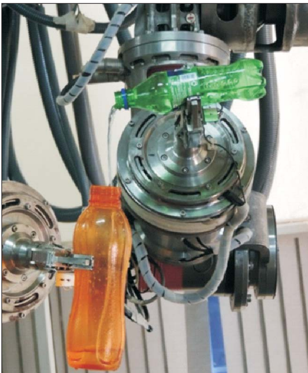
Delicate operations using Servo manipulator
