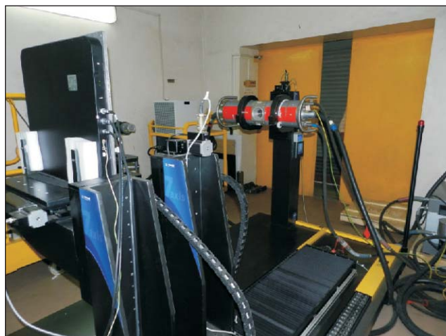
X-ray based Industrial Digital Imaging and Volume Computed Tomography facility
