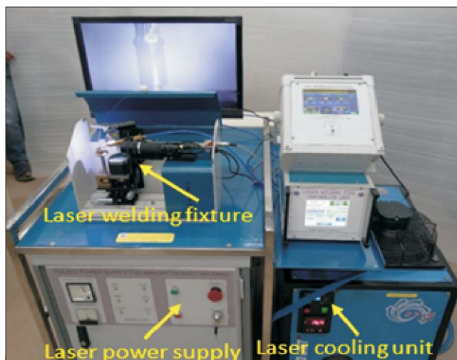
In-house developed Nd:YAG laser system for welding of Ir-192 brachytherapy assembly
