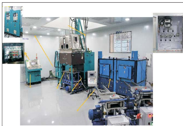
BRNS funded: 15 L Induction furnace setup at CGCRI at Kolkata for RRCAT, DAE
