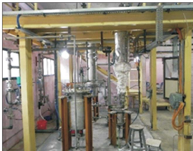
Experimental set-up of Fluidization based chemical vapour deposition technique
