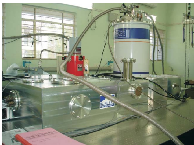
IR-THz frequency domain spectrometer set up for the utilization of FEL radiation
