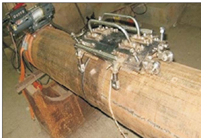
Magnetic Flux Leakage (MFL) based tool for sectoral inspection of pipelines
