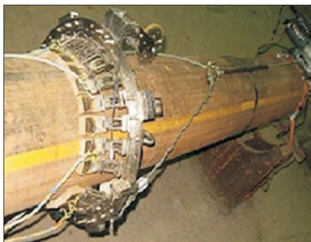
Ring-type Eddy Current based inspection system for Pipeline Inspection Gauges
