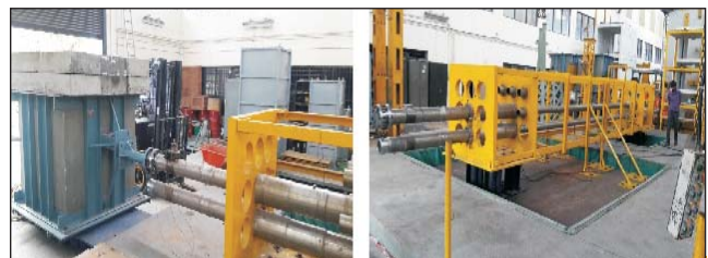
Seismic Testing of Coolant Channel Assembly
