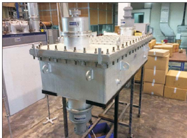
A new type of wideband Hybrid Megawatt (MW) Level Continuous Wave (cw) Radio Frequency Combiner/Splitter has been designed and developed
