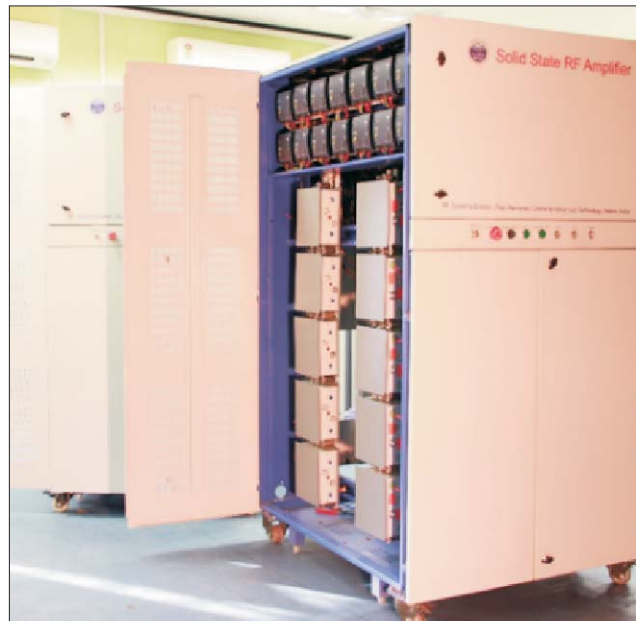
100 kW, 325 MHz pulsed solid-state RF amplifier for RFQ
