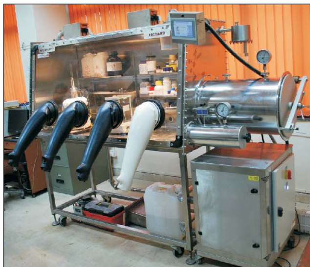
Electrochemical salt purification demonstration facility located inside an inert gas glovebox with oxygen and moisture content kept below 1 ppm each
