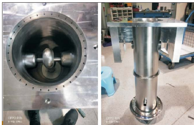
Photograph showing Niobium Quarter Wave Resonator (QWR) cavities being prepared for tests at TRIUMF
