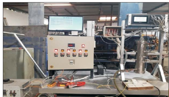
19 Element Fuel Bundle Simulator Test Setup
