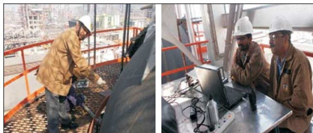
Gamma scanning of Extractive Distillation Column (ED)
