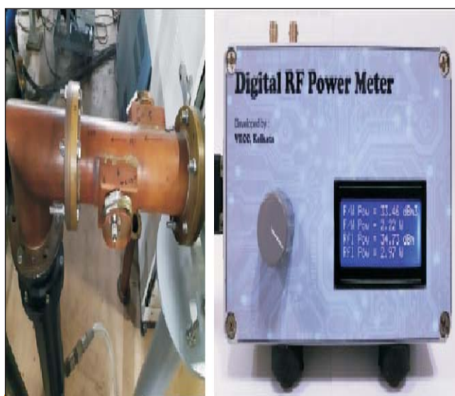
(left) Dual Directional Coupler (DDC) and (right) RF power meter designed and developed indigenously at VECC
