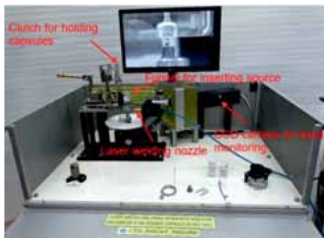
Laser micro-welding workstation for Ir-192 brachytherapy assemblies
