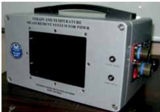
User configurable multichannel strain and temperature measurement system for 700 MWe PHWRs
