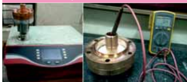
Qualification checks for vacuum and electrical compatibility
