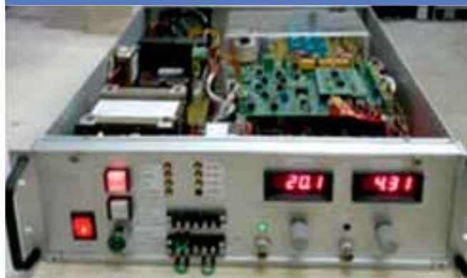
0-20kV/5mA High-Voltage DC Power Supply
