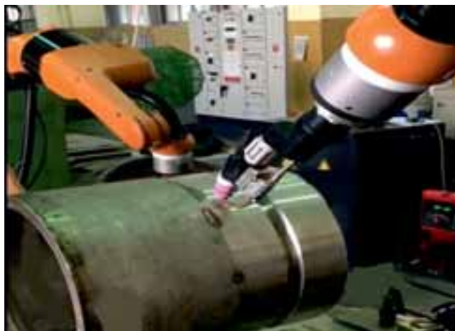
At play are the twin two robotic arms of the welding station
