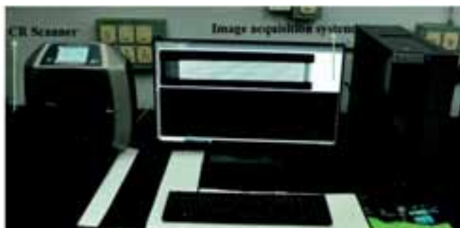
Computed Radiography Scanner System installed at BARC Radiometallurgy Division
