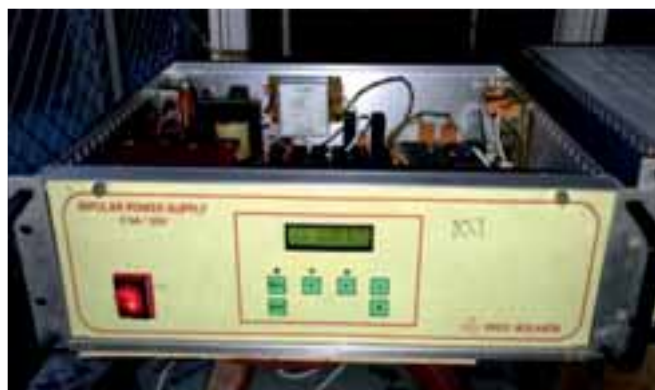
\pm 5A , \pm 20V current-regulated true-bipolar dc power supply
