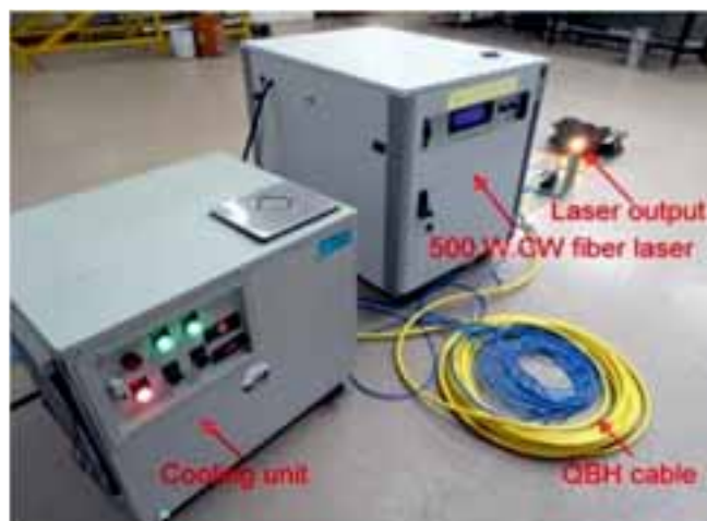
In-house developed 500 W Continuous Wave (CW) fiber laser system
