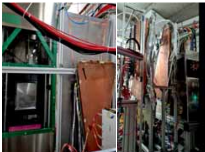
Picture of the upgraded mMUCH detectors (left) Picture of the RPC module (in large Aluminium enclosure) and GEM module placed back-to-back under test at GIF++ (right)
