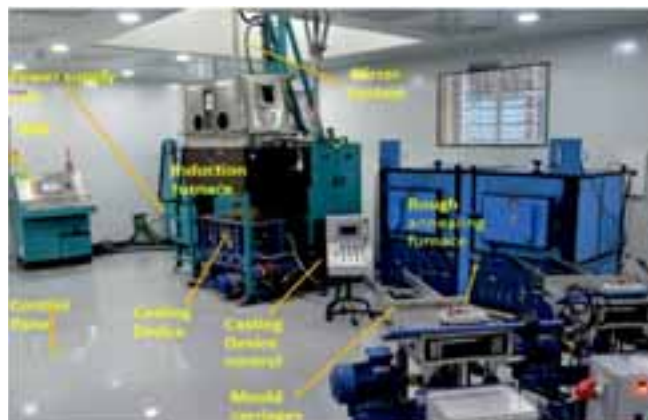
Development of technology for large sized Nd-doped phosphate LASER glass blocks and discs
