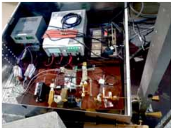
100 GHz quadrature based (IQ) heterodyne interferometer
