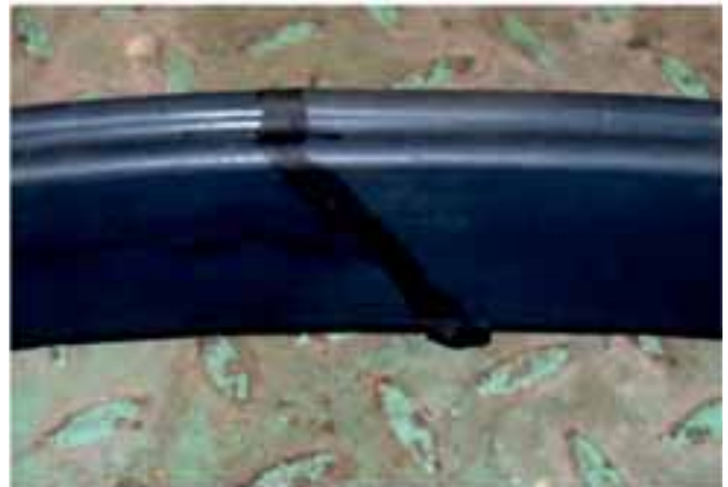
Test Seal with In-Situ Joint
