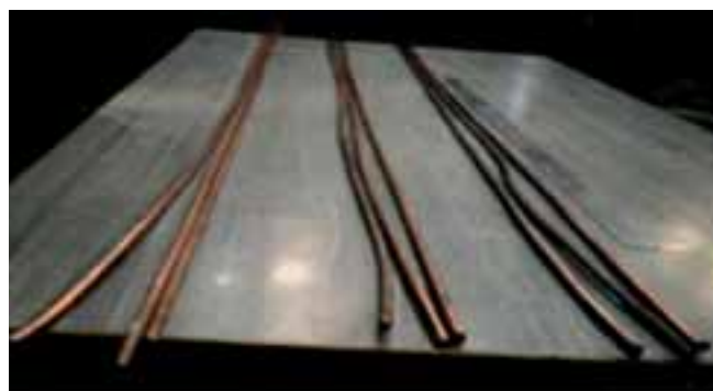
Development of low diameter (9m dia) Zr-2.5Nb-0.5Cu (ZNC) extrusion
