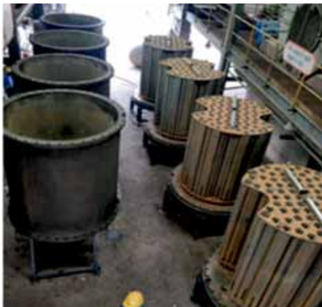
Stage internals of 12TI exchange tower at HWP, Hazira
