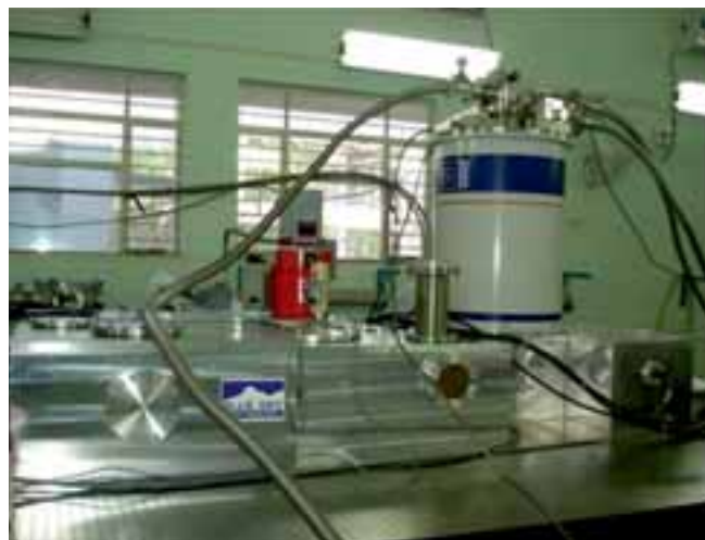
Set-up for doing frequency domain spectroscopy at low temperatures (5- 300 K) and high magnetic fields (up to 7 T) using FEL and laboratory based sources
