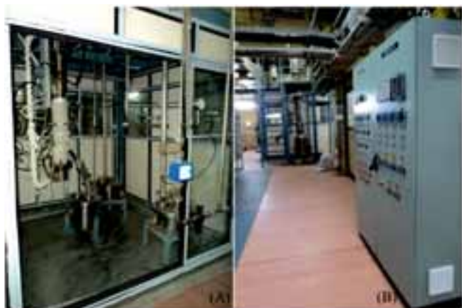
Fluidized bed reactor system inside enclosure (left) and Instrumentation control panel in Direct Denitration Demonstration Plant (right)
