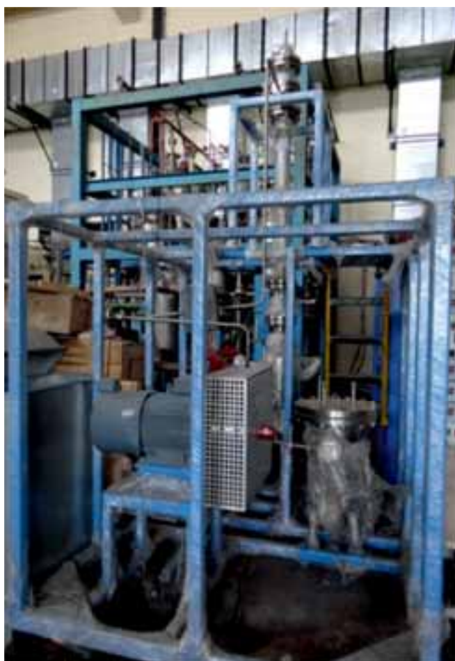
Pb-Li Extractor Loop showing high temperature electromagnetic pump
