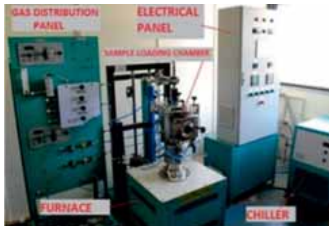
Auto dipping set up for corrosion studies
