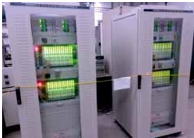
CAAS panels undergoing burn-in test at ECIL facility in Hyderabad
