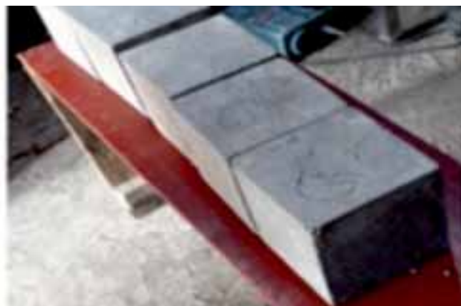
The developed Concrete-Graphite Oxide cubes and their compressive strength
