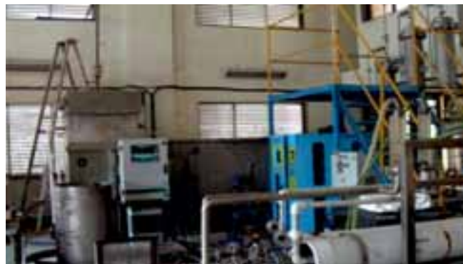
Effluent Water Treatment Plant (AEWTP) of 500 litres per hour capacity
