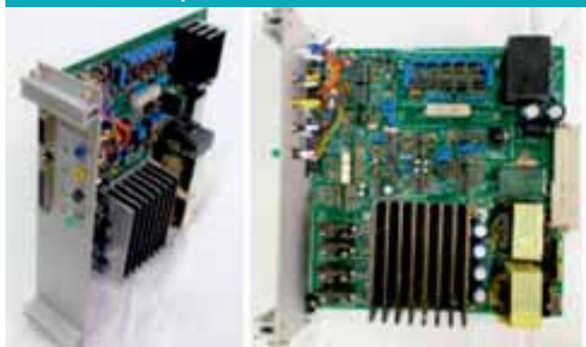
Bipolar power converter on 6U printed circuit board
