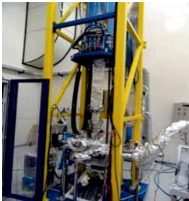
Magnetron sputtering deposition system with vacuum chamber installed for coating
