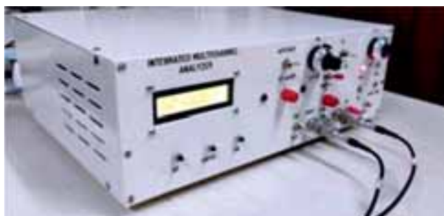
Integrated high resolution multi-channel analyzer
