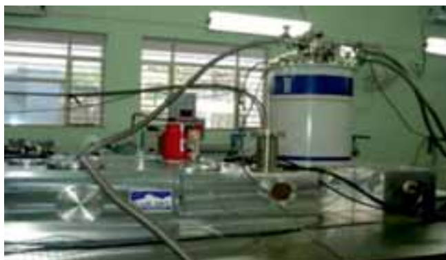
Set-up for doing frequency domain spectroscopy at low temperatures (5- 300 K) and high magnetic fields (up to 7 T) using FEL and laboratory-based sources
