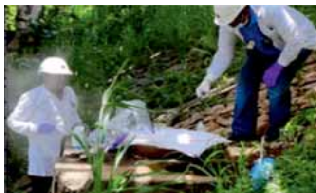
Radiotracer study for Oil Leakage Detection in a Petrochemical Plant
