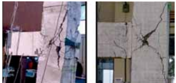
Crack pattern in Un-corroded (left) and Corroded (right) frames at failure
