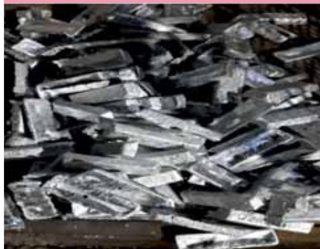
Ingots of Al-Zr Master Alloy
