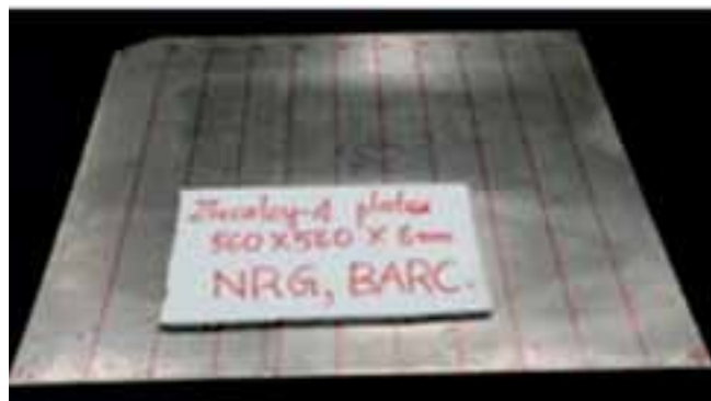
Zircaloy-4 plates of 525 x 525 x 6 mm size
