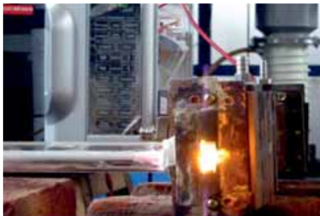
Microwave plasma arc at atmospheric pressure fluorescent tube
