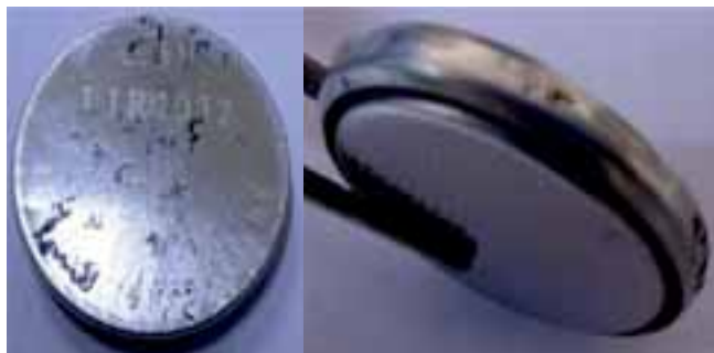
Supercapacitor made using nanocomposites of poly (3,4-ethylenedioxythiophene)-poly (styrene sulfonate)
