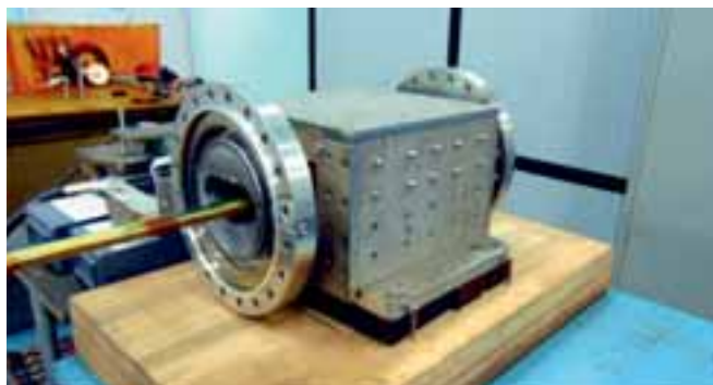
The horizontal pinger magnet under magnetic measurement
