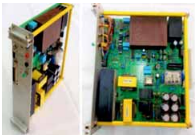
Unipolar power converter on 6U printed circuit board
