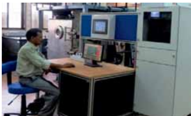
80 kV, 12 kW Electron Beam Welding Machine developed in BARC
