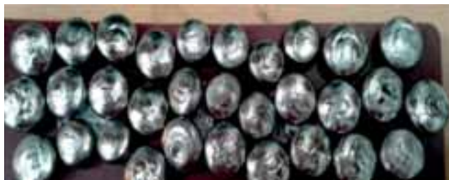
Ti 2 CrV alloy samples prepared using arc melting technique
