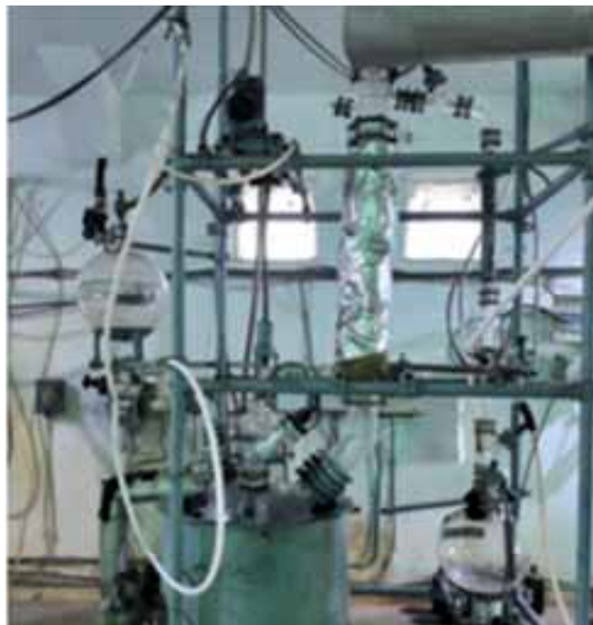
Pilot plant set-up for synthesis of calix Crown-6 at HWP, Talcher
