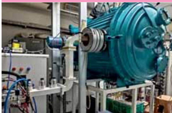
An indigenously developed SPIX facility with ECR plasma source for the ground testing of satellite solar panels before launching into space.
