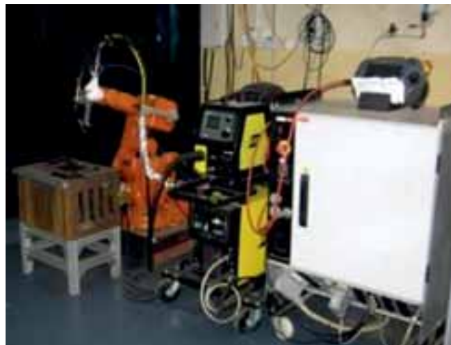
A view of developed Hybrid Laser Arc Welding System (HLAW)
