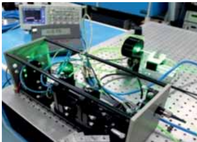
Photographs of compact green laser under operation
