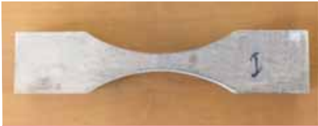
Borated Wood Test Specimen
