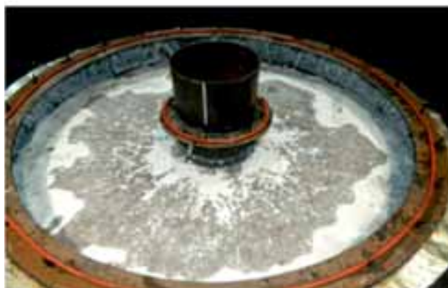
Experimental Setup for response time evaluation of core temperature probe
