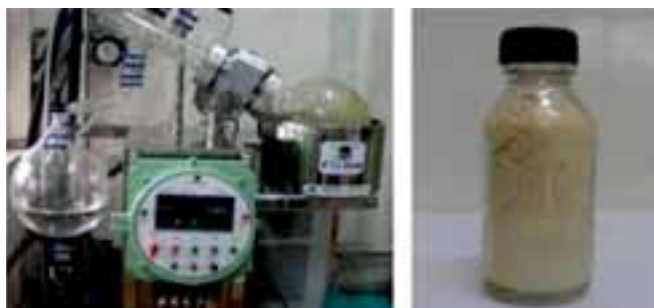
20 L rotary evaporator for recovery of solvent (on the left) and 95% pure DTBDB18C6 product (on the right)
