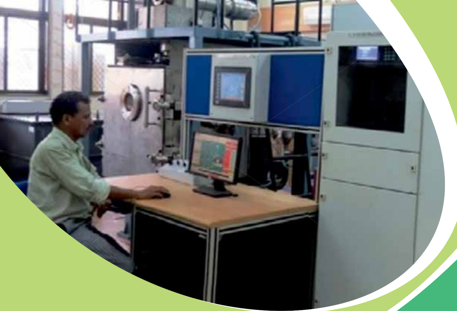
80 kV, 12 kW Electron Beam Welding Machine developed in BARC
