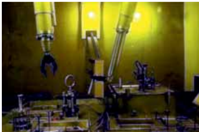
Facility for welding and overpacking of Cesium Pencil
