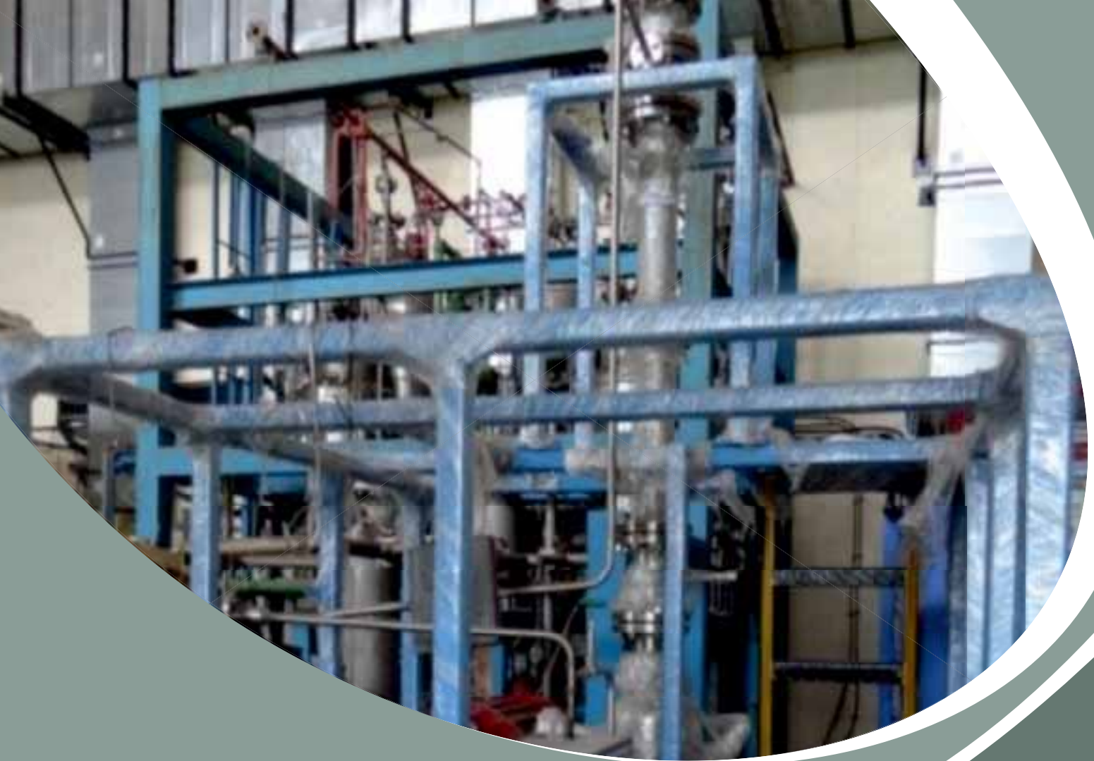
Pb-Li Extractor Loop showing high temperature electromagnetic pump
