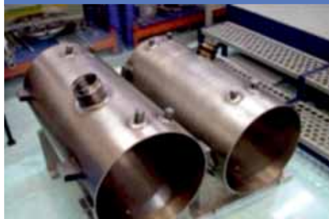
Ti grade 2 Helium vessels for dressing
