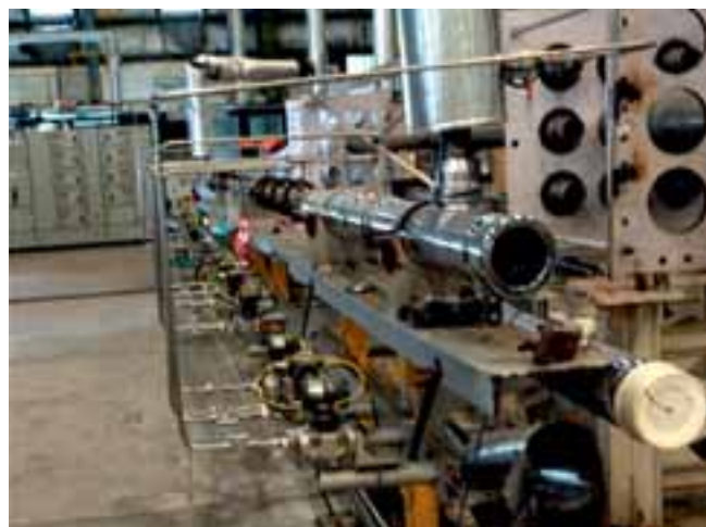
Test Set-up for Coolant Channel Pressure Drop Measurement
