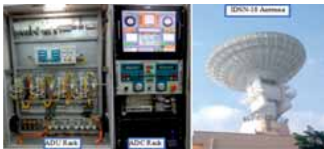
BARC developed Antenna Control Unit (extreme left), and Supervisory Gateway Controller (centre) for the IDSN -18 antenna (last)
