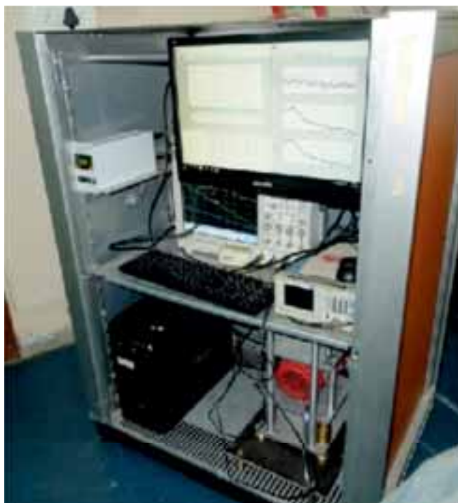
The 19-inch rack-mounted system for detection of heavy water in air installed in Dhruva facility
