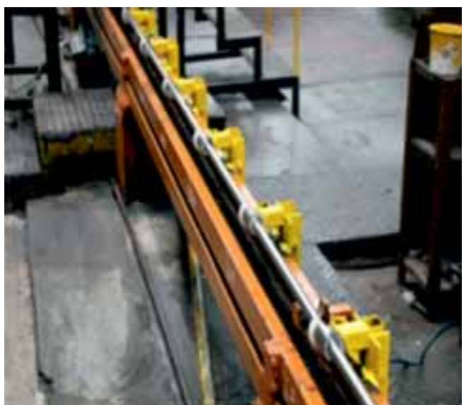
Modification of tube feeding system in CRTM 32 pilger mill
