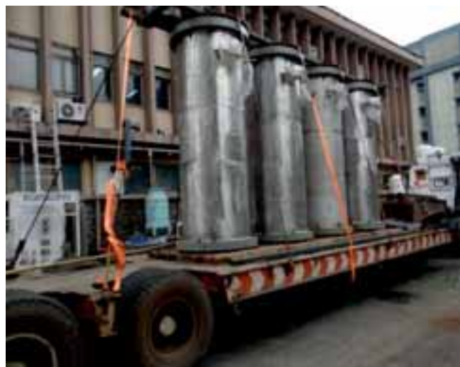
Column Sections of Heavy Water upgrading tower loaded onto a trailer for dispatch
