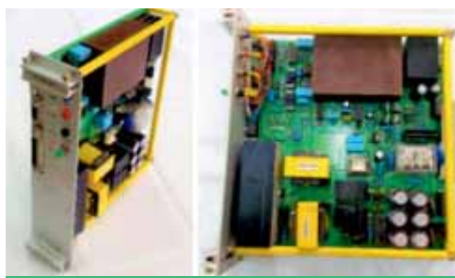
Unipolar power converter on 6U printed circuit board
