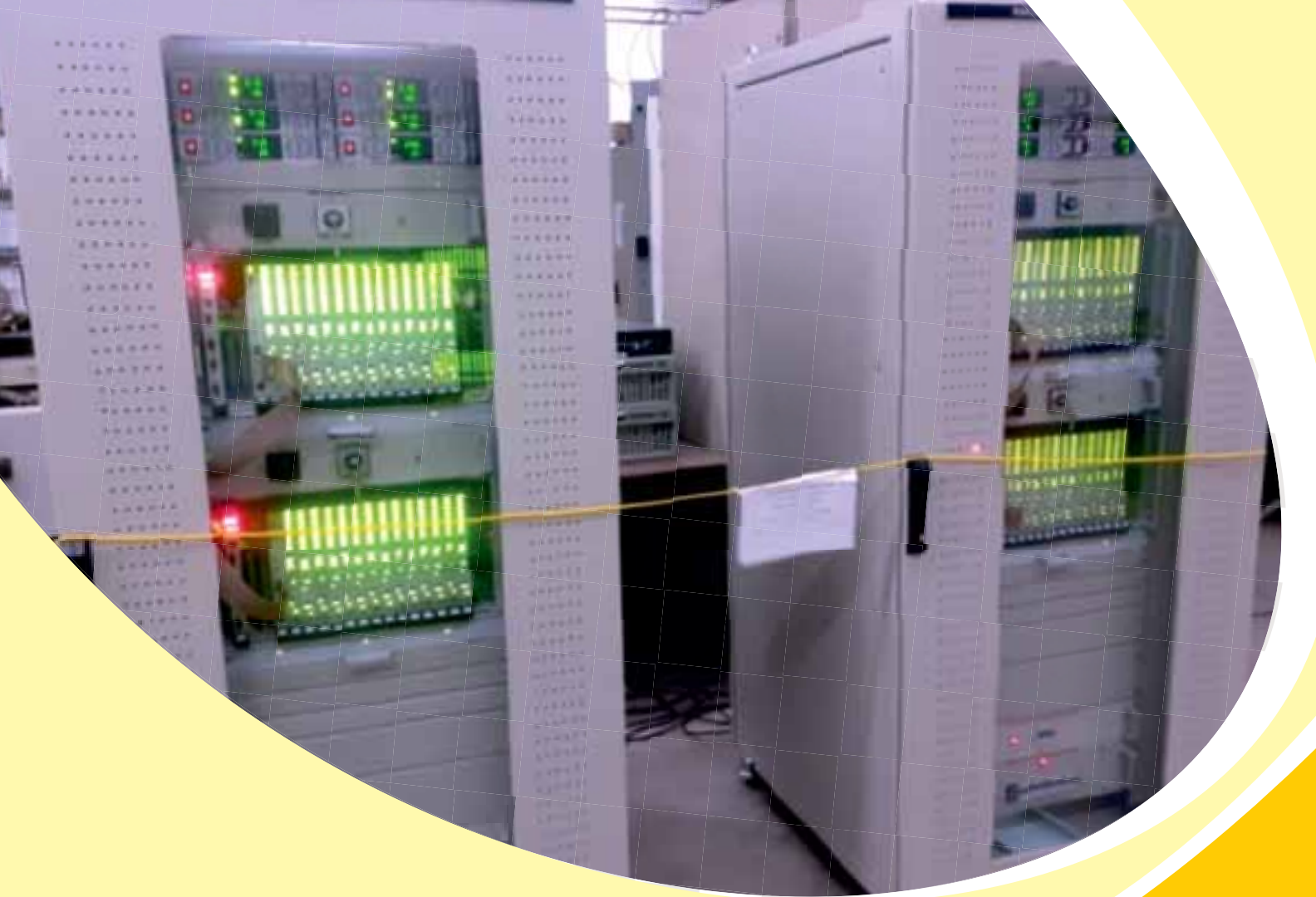
CAAS panels undergoing burn-in test at ECIL facility in Hyderabad
