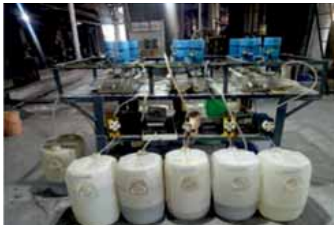
Bench scale mixer settler setup for Cobalt-Nickel separation at TDP, Mumbai
