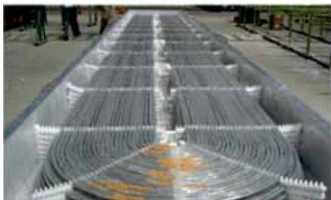
Manufacturing & delivery of 2nd set of Steam Generator tubes
