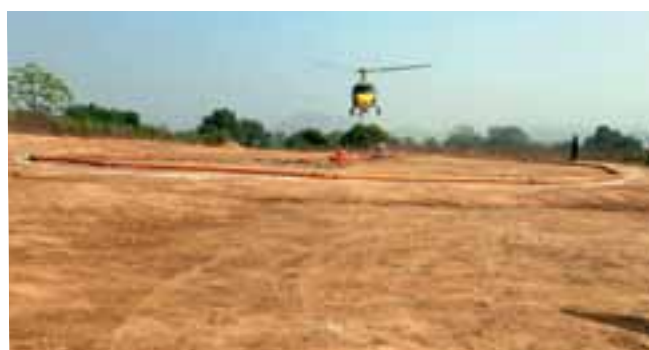
Preparation of heliborne geophysical survey with VTEM plus system, Kota helibase, Sonbhadra district, Uttar Pradesh
