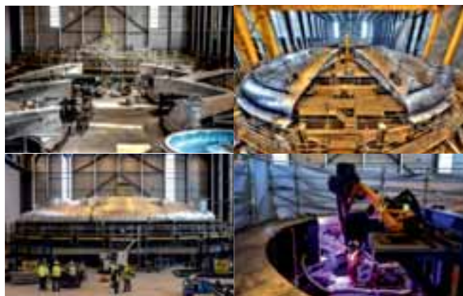
Clockwise from top; top lid segments at ITER India work shop undergoing pre assembly and alignment checks prior to welding with robotic arms
