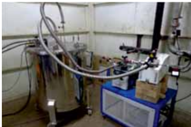
A cryogen-free low temperature set-up has been deployed by BARC for testing quantum components
