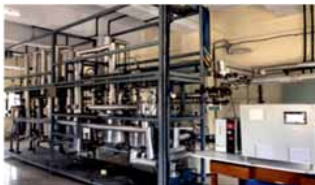
Electrolyser and Recombination unit to produce \text{H}_2^{18}\text{O} from \text{D}_2^{18}\text{O} at HWP, Manuguru
