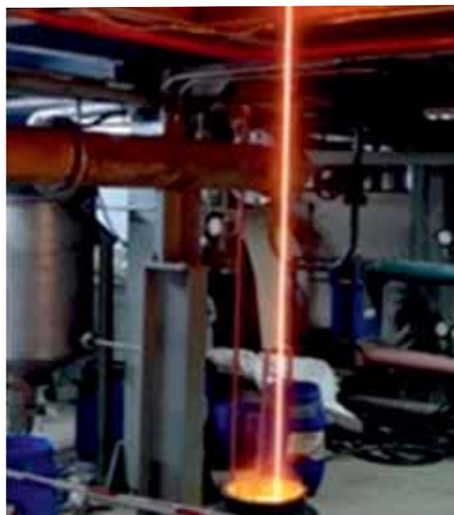
Cold Crucible Induction Melter for vitrification of HLW
