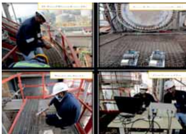
Gamma Scanning of Reactor Regenerator System of BPCL, Mumbai Refinery
