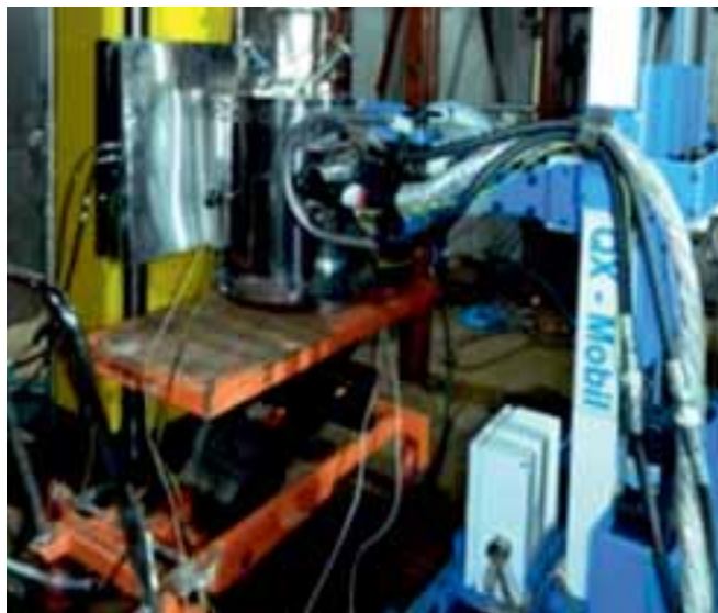
Sodium Boiling setup with X-ray imaging system
