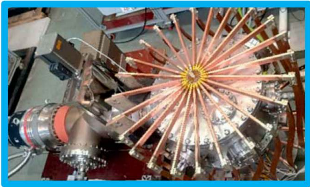
SMARTEX-C Upgrade with steady state TF coil
