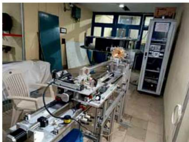
Assembly of Stripper drive mechanism completed
