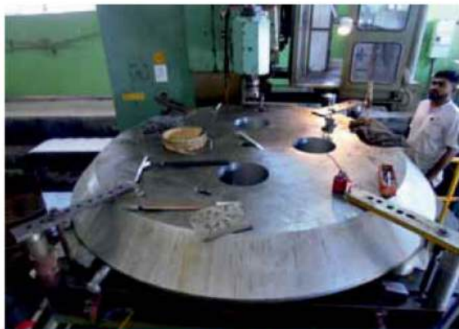
Pole cap machining in progress
