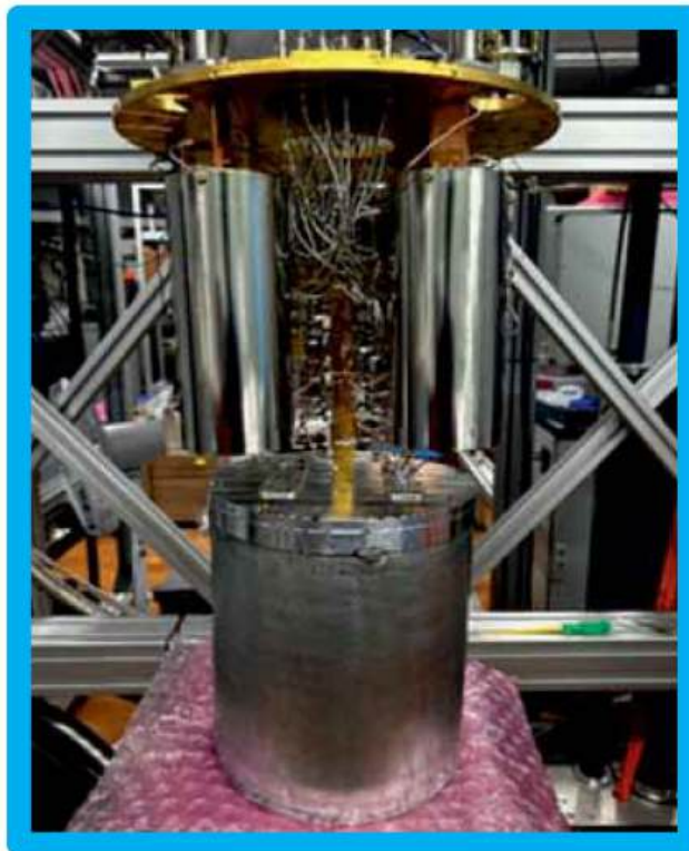
Cryogenic stage of a superconducting quantum computer, which cools down to -273.13^{\circ}\text{C}
