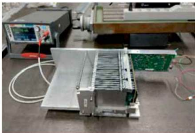
A prototype assembly structure of n-type Si detectors coupled to tungsten plates
